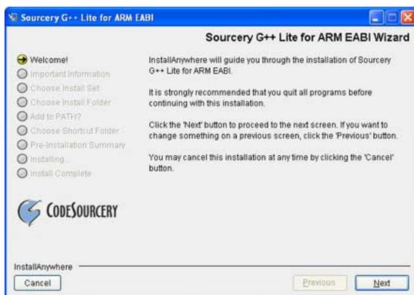
When the message box "Chose Install Folder" appears, type a simple path like `c:\codesourcery` avoid using the default path. On m XP for example the default path is `C:\Program Files\CodeSourcery\Sourcery_CodeBench_Lite_for_ARM_GNU_Linux` that Eclipse v not manage.
