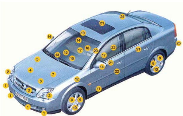
2002: Opel Vectra has over 40 sensors (25 types)
