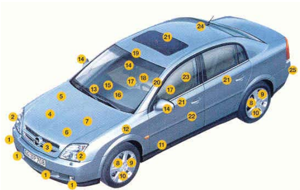
2002: Opel Vectra has over 40 sensors (25 types)
