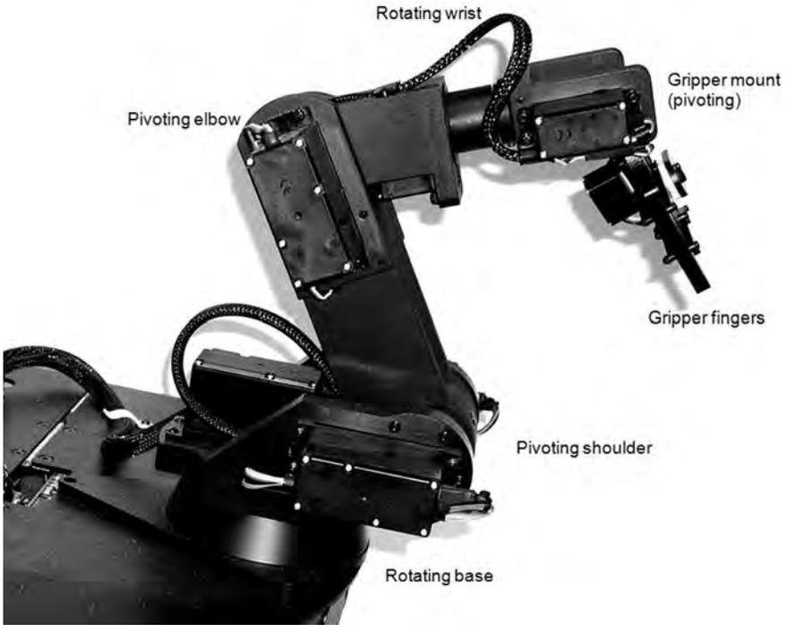
**Fig. 2.5** The joints on the Pioneer
