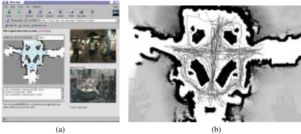
Fig. 16. (a) Web control interface. Users can authenticate themselves in on the left side of the window, and subsequently specify target locations by clicking on the map. The map shows current robot position and pending target locations, and a dialogue box displays the current speed of the robot. On the right, users can watch images recorded using the robot's camera (top image) and by a stationary camera with zoom mounted on a pan/tilt unit (bottom image). (b) Multihour path of the robot in the museum.
