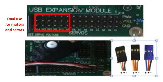
Figure 4.7: Servo ports include3 rows (PWM, Vsel, GND)
