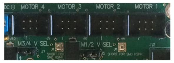
Figure 4.5: PCB Motor Ports and voltage select
