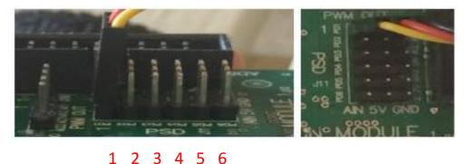
Figure 4.9: PSD connection from side and top view. Always start from PD1 when connecting PSD sensor
