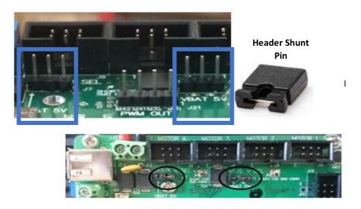
Figure 4.6: Shunt pin header on pin 1 and pin 2 for battery supply or to pin 2 and 3 for 5VDC supply.
