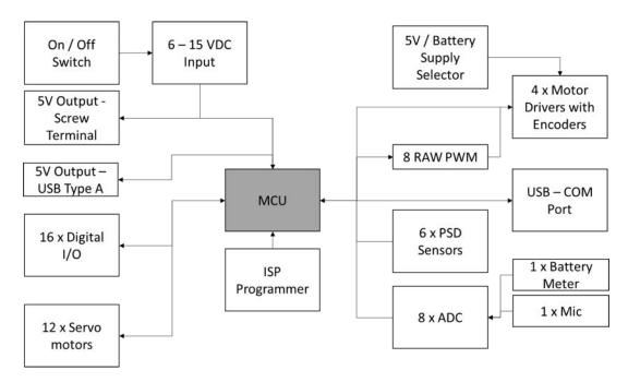
Figure 4.12: EyeBot7 IO-Board bock diagram
