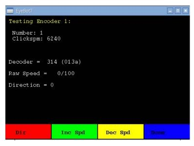
Figure 1.8: Encoder testing page (HDT)
