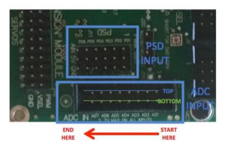
Figure 4.8: IOBoard 7 - Analog ADC Input pins and 6 PSD Input pins.
