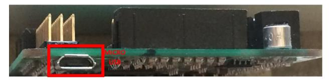
Figure 4.11: Micro USB to communicate with a host controller (e.g. Raspübery Pi)
