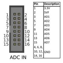
Figure 4.14: EyeBot7 Analog input
