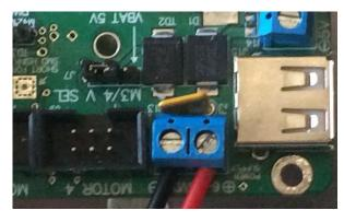
Figure 4.3: Power Supply Terminal Input
