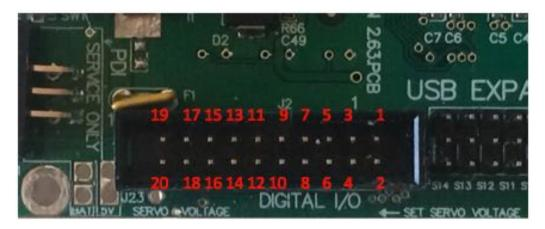
Figure 4.10: Digital I/O Port. These ports are designed so that a user can write and read data as a Byte.
