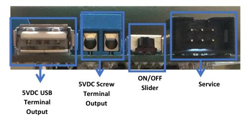
Figure 4.2: Power Connections
