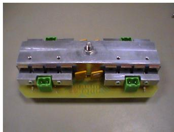
FIGURE F.8: MOSFET motor controller board.
