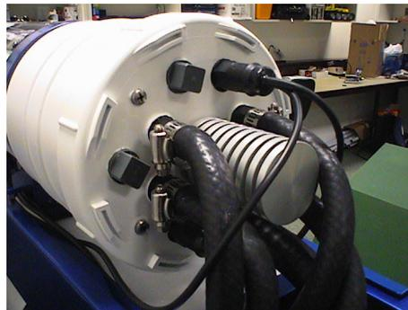
FIGURE 3.10: Heat sink located in the centre of the upper hull's end cap.
