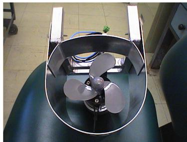
FIGURE F.5: Vertical motor mount.
