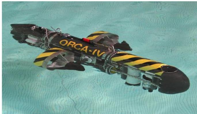
FIGURE 2.5: MIT's *Orca* AUV being tested in a swimming pool [27].
