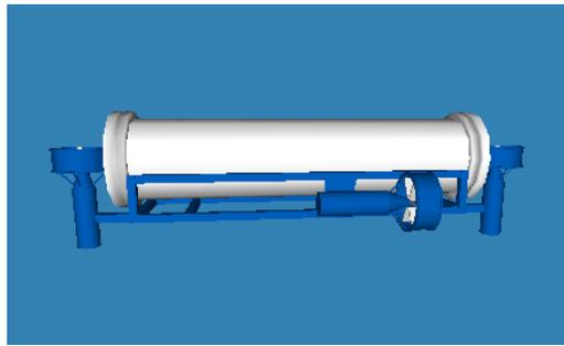
FIGURE C.2: The one-hull, four-thruster concept design.
