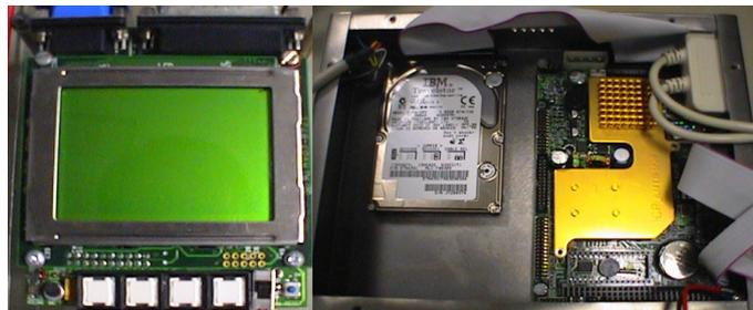
FIGURE B.3: (Left) Eyebot microcontroller. (Right) Cyrix mini PC .
