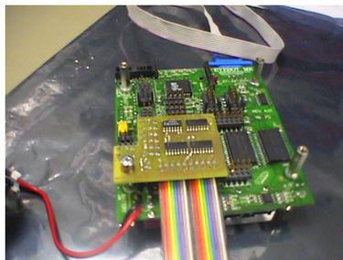
FIGURE F.7: Motor controller logic circuit board on the back of the Eyebot.
