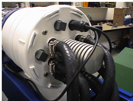
FIGURE F.14: The external connections on upper hull's end cap.
