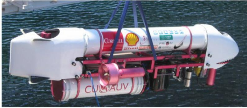
FIGURE 2.7: Cornell University's AUV being deployed [30].
