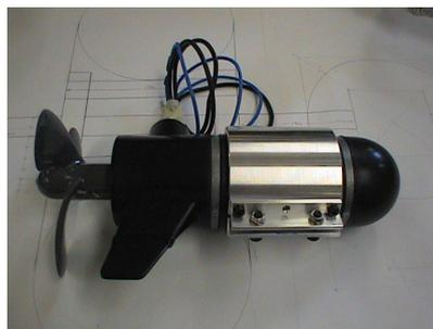
FIGURE F.2: Motor with clamp.
