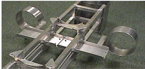
FIGURE F.6: The adjustable mount for the forward motors.
