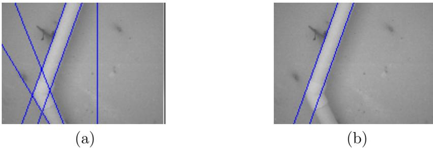
FIGURE 5.11: (a)Line extraction using the Hough Transform. (b)Extraction of parallel line pairs.
