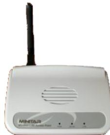
FIGURE A.3: Minitar wireless access point.
