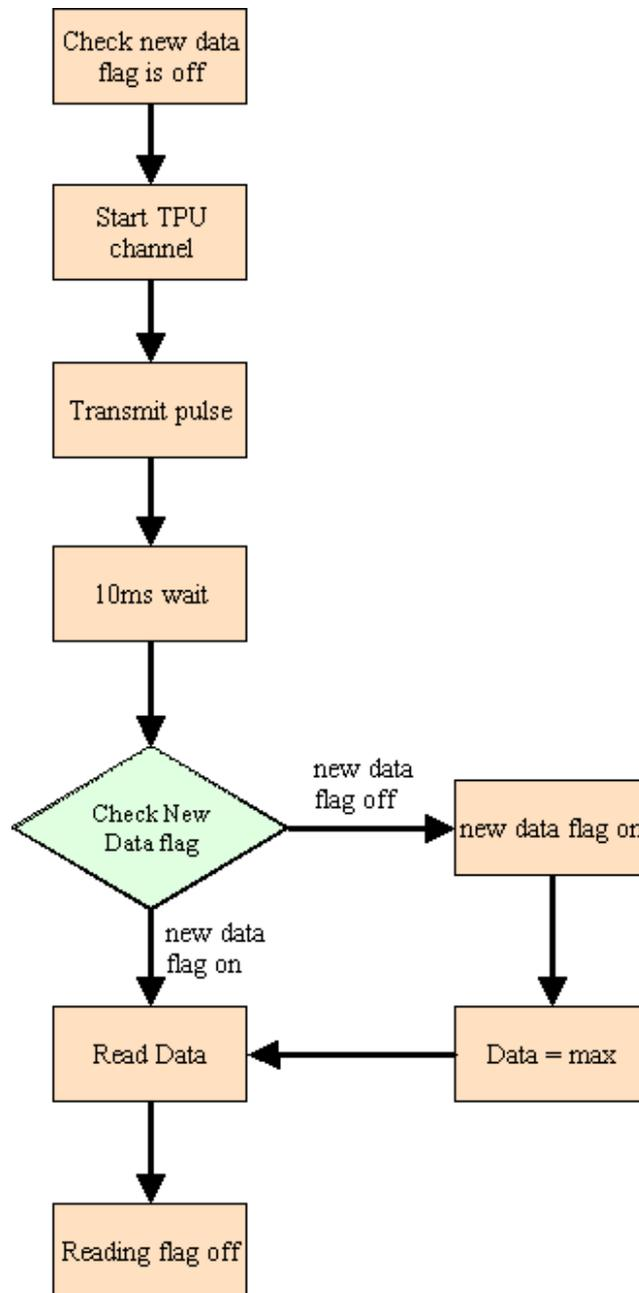
Figure 5.2: The flow chart for the echo sounding process
