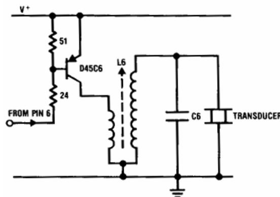
Figure 8.1: The pulse amplifier [14]
