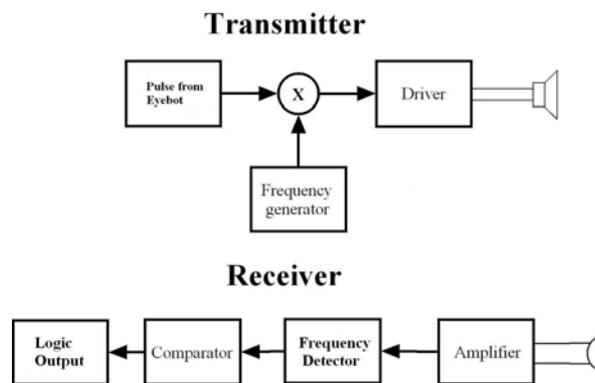
**Figure 2.3: Echo sounder operation flow chart**
