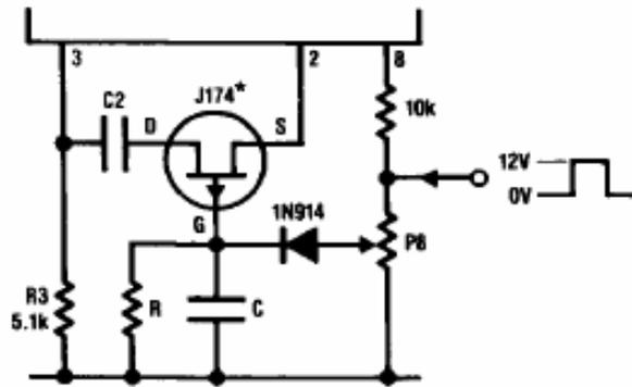
Figure 8.2: Time variable attenuator [14]
