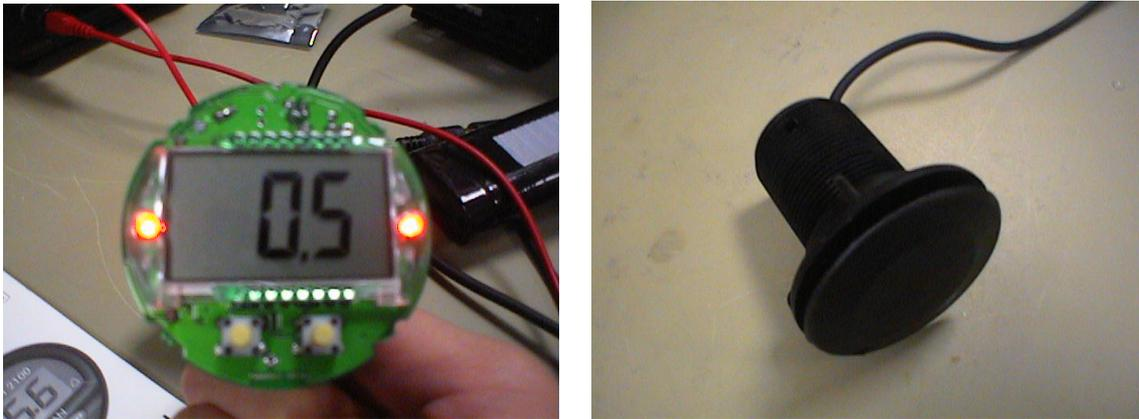
**Figure 4.1a) & b): the Navman echo sounder circuit board and transducer**
