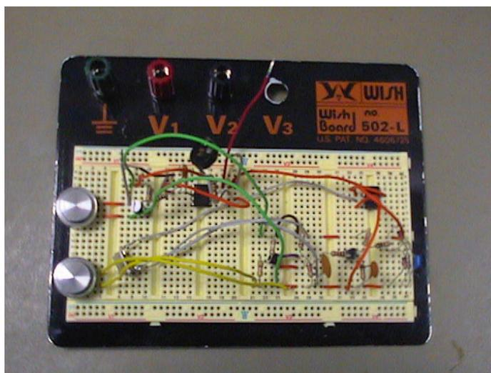
Figure 4.4: Circuit layout of an ultrasonic switch
