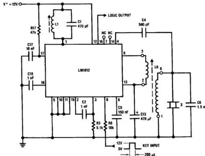
**Figure 4.5: Circuit diagram of the echo sounder circuit design [14]**
