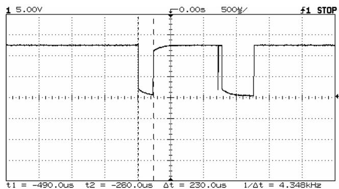
**Figure 6.5: 200 $\mu$ s pulse sent via the digital output, and the transducer is placed in water**
