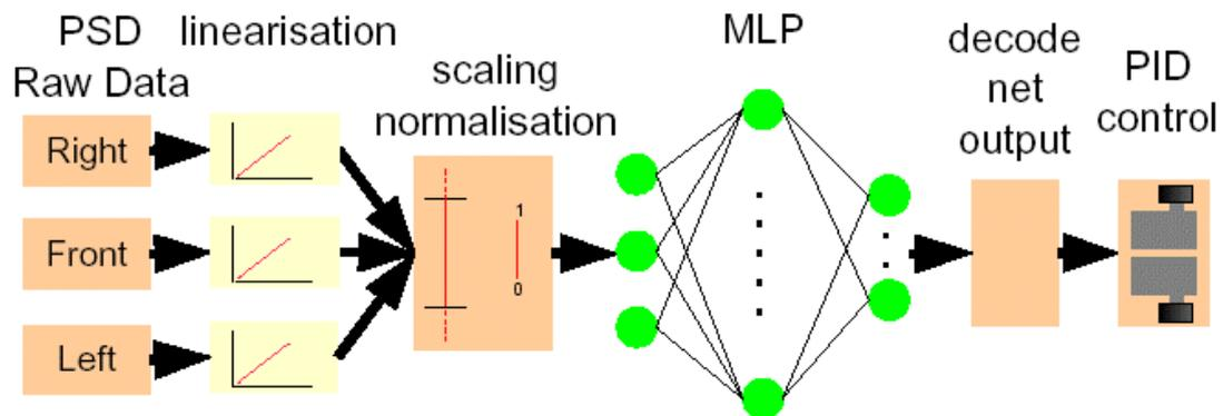
The used sensors (Sharp GP2D02) have a non linear-output. In order to get a distance measurement you have to do a linearization and a scaling first (detail 2.1). After that, I blend out distances that can either not occur or are not relevant for the task by clipping the distance measurements to the range from 92mm to 420mm. This range is than scaled to 0 to 1.
