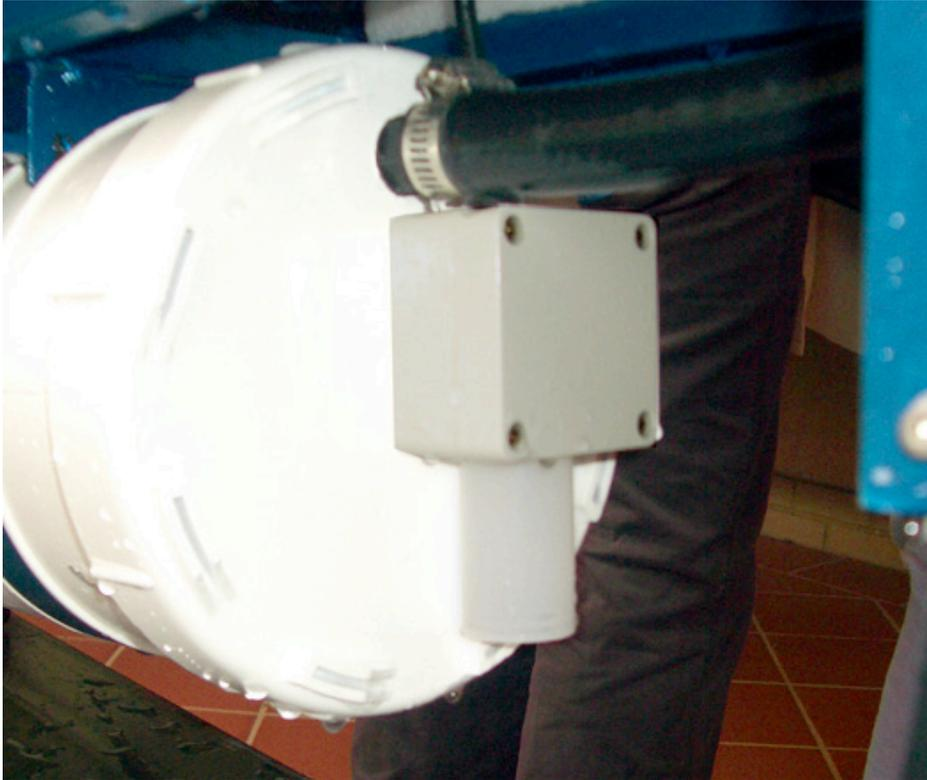
**Figure 20: Installed depth sensor**
