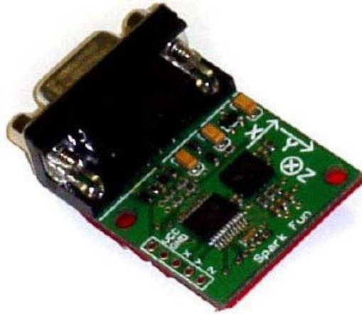
Figure 3.29: The Sparkfun Accelerometer
