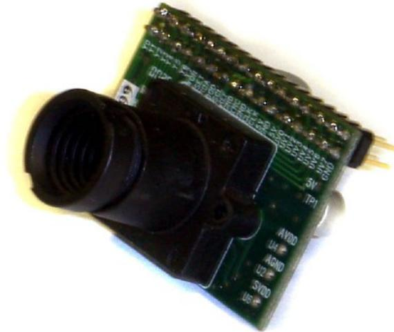
Figure 3.34: The camera module
