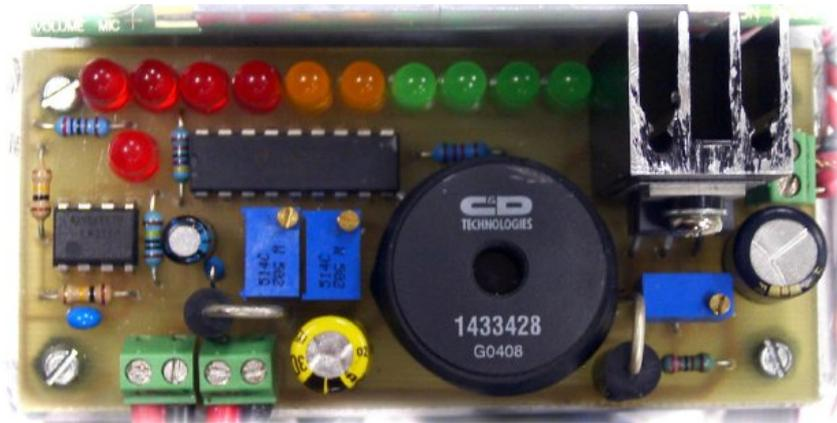
Figure 3.11: DC-DC step-down converter and battery gauge
