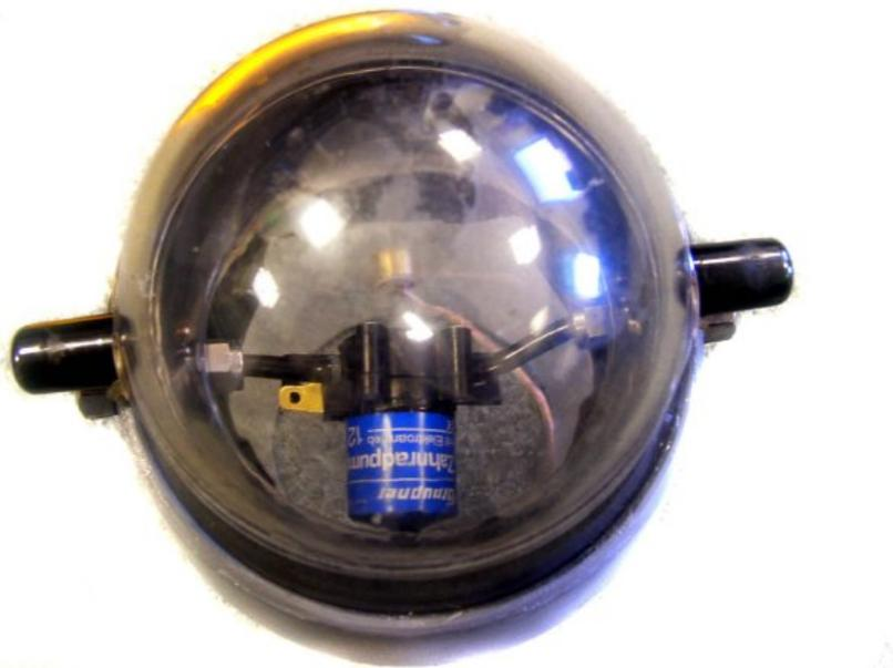
Figure 3.23: The bow thruster system
