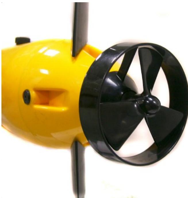
Figure 3.21: The 3-winged propeller of the stern thruster
