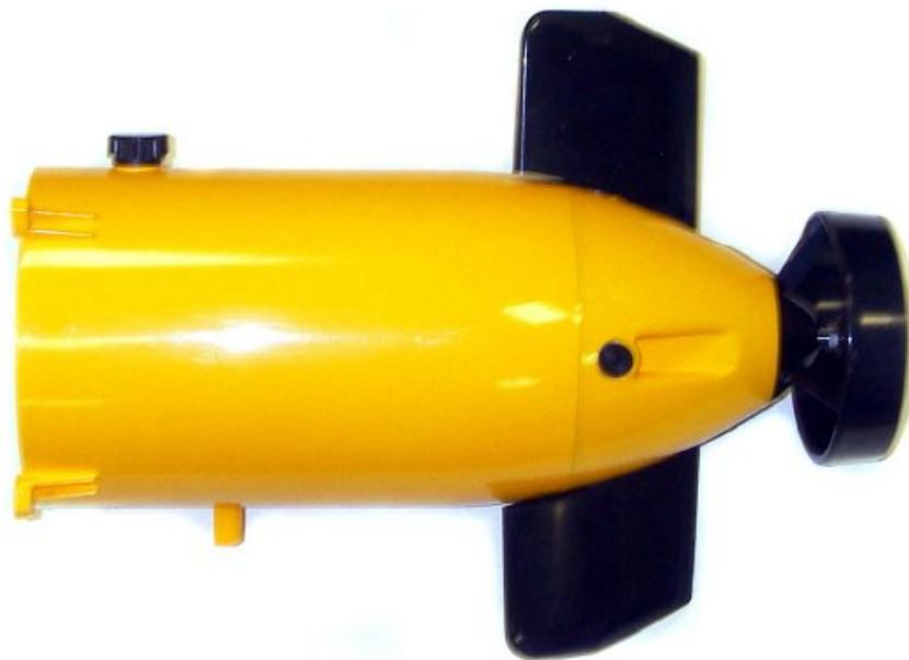
Figure 3.4: The stern hull
