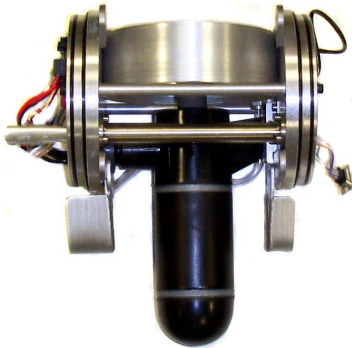
Figure 3.3: The heave thruster unit
