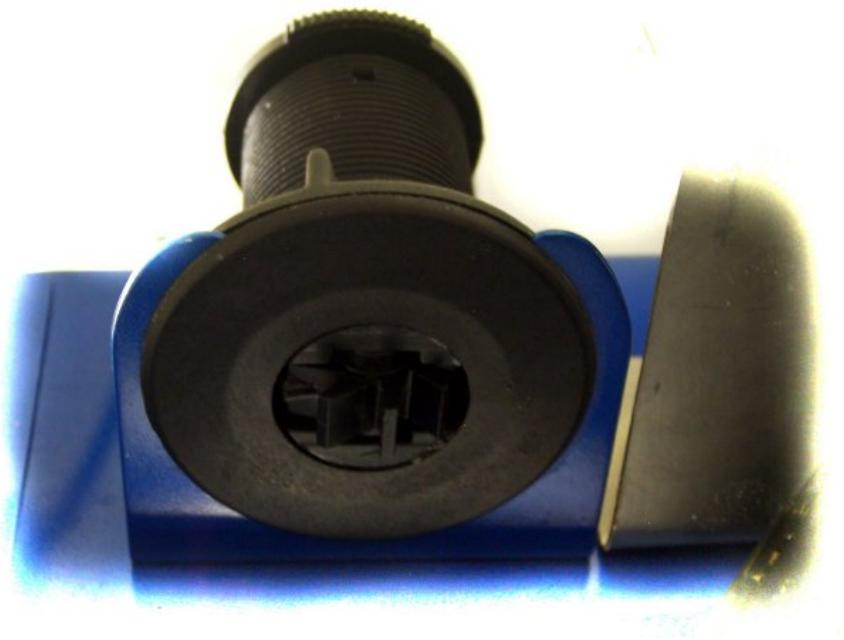
Figure G.02: Paddlewheel as used in bigger boats
