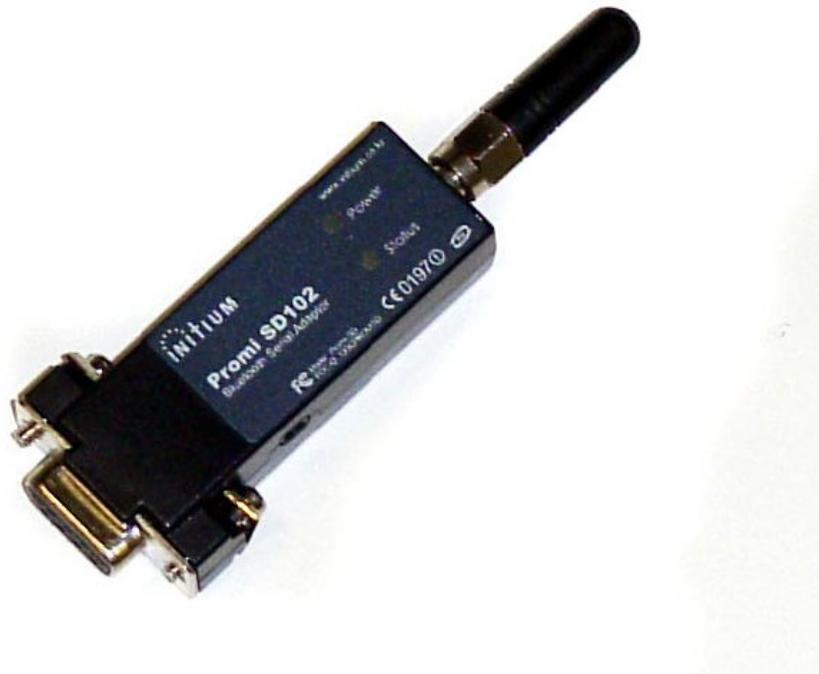
Figure 3.24: The Bluetooth communication device
