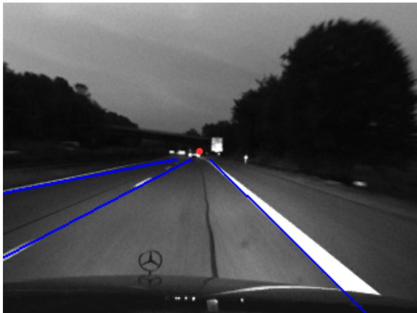
Figure 6.11: Detected lines in example image
