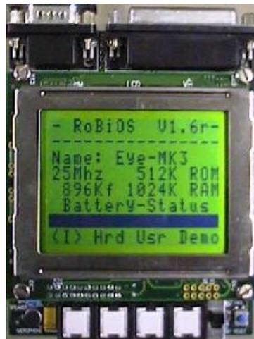
Figure 4.1: Eyebot controller LCD
