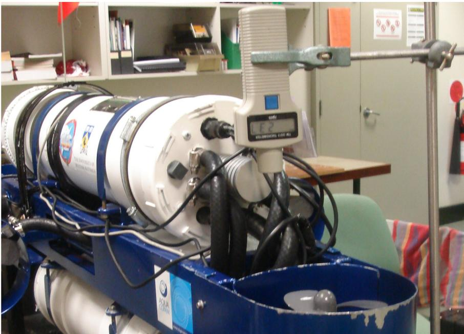
FIGURE E.3: An optical tachometer was used to measure the revolutions of the propellers
