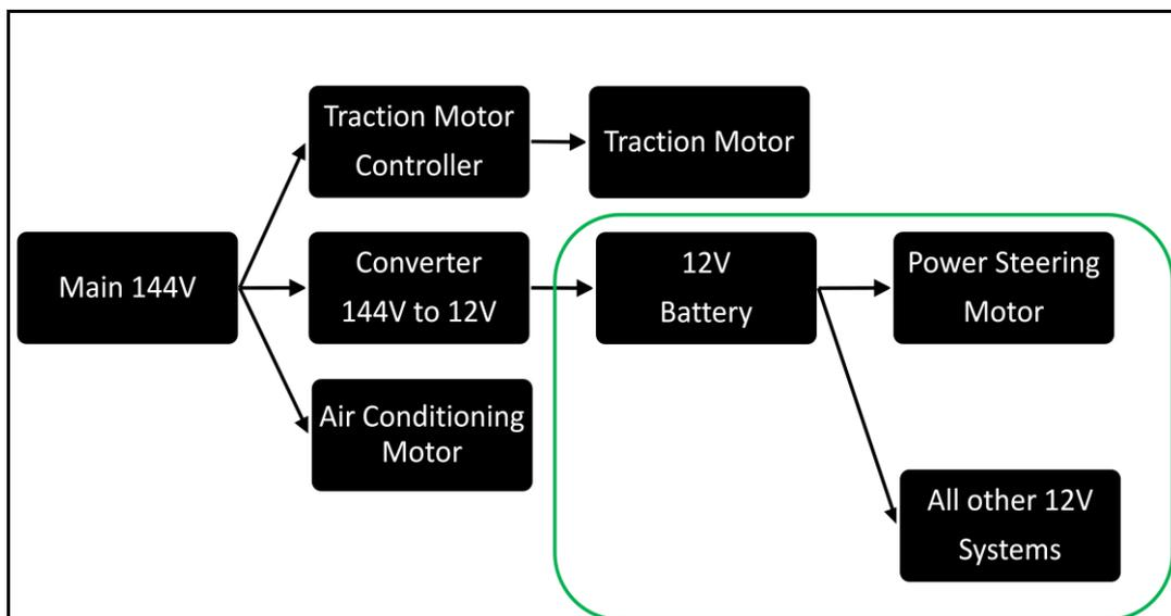
FIGURE 23: EHPAS ENERGY SUPPLY DIAGRAM
