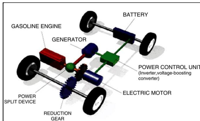
FIGURE 2: TYPICAL HYBRID CONFIGURATION,(PROKHOROV, 2008)
