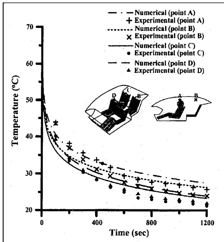
FIGURE 11: TEMPERATURE VS TIME PLOT OF EXPERIMENTAL & NUMERICAL DATA
