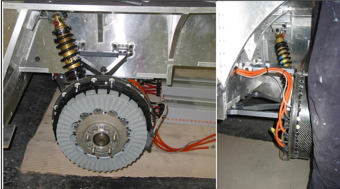
Figure 19: Wheel motor (HybridAuto.PTY.LTD, 2006)
