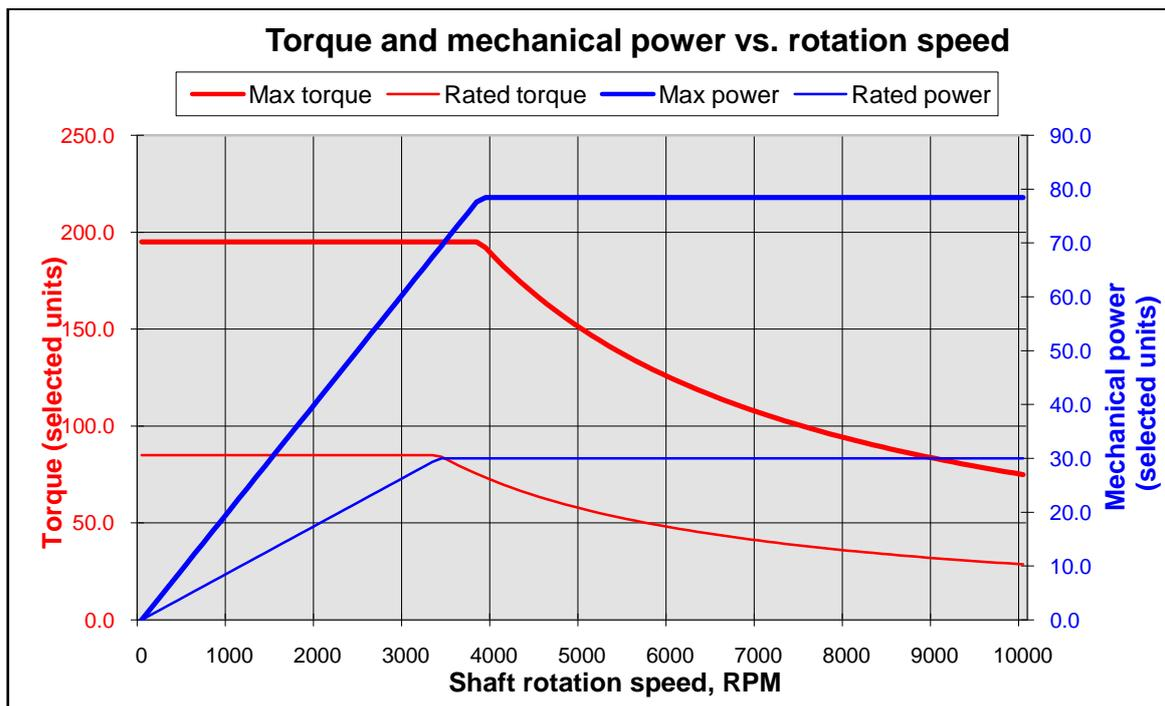
FIGURE 21: AC INDUCTION MOTOR PERFORMANCE CURVE (METRICMIND, 2008)
