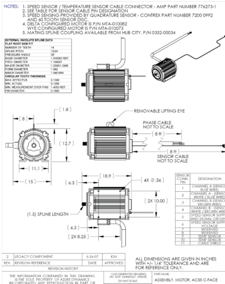
FIGURE 36: AC55 TRACTION MOTOR DIMENSIONS
