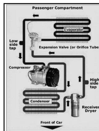
FIGURE 3: TYPICAL AUTOMOTIVE A/C SYSTEM CONFIGURATION, (CHILLYWILLYS.ORG, 2008)
