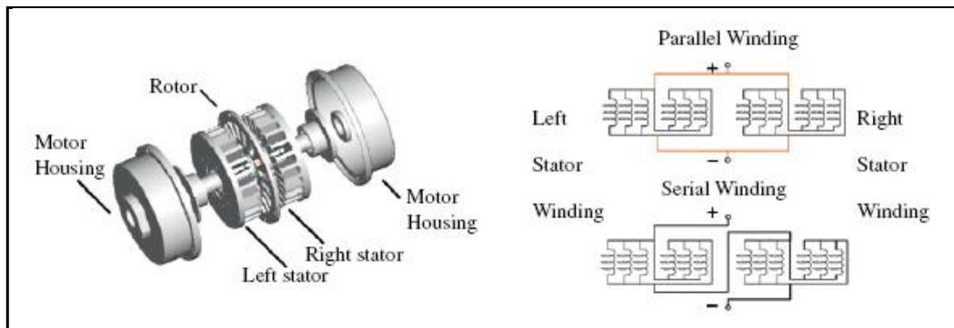
FIGURE 8: ELECTRIC WHEEL MOTOR CONFIGURATION(YANG AND LO, 2008)
