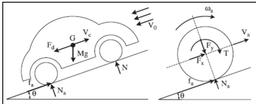
FIGURE 7: WHEEL MOTOR SLIP FOR AN INCLINED SLOPE (YANG AND LO, 2008)
