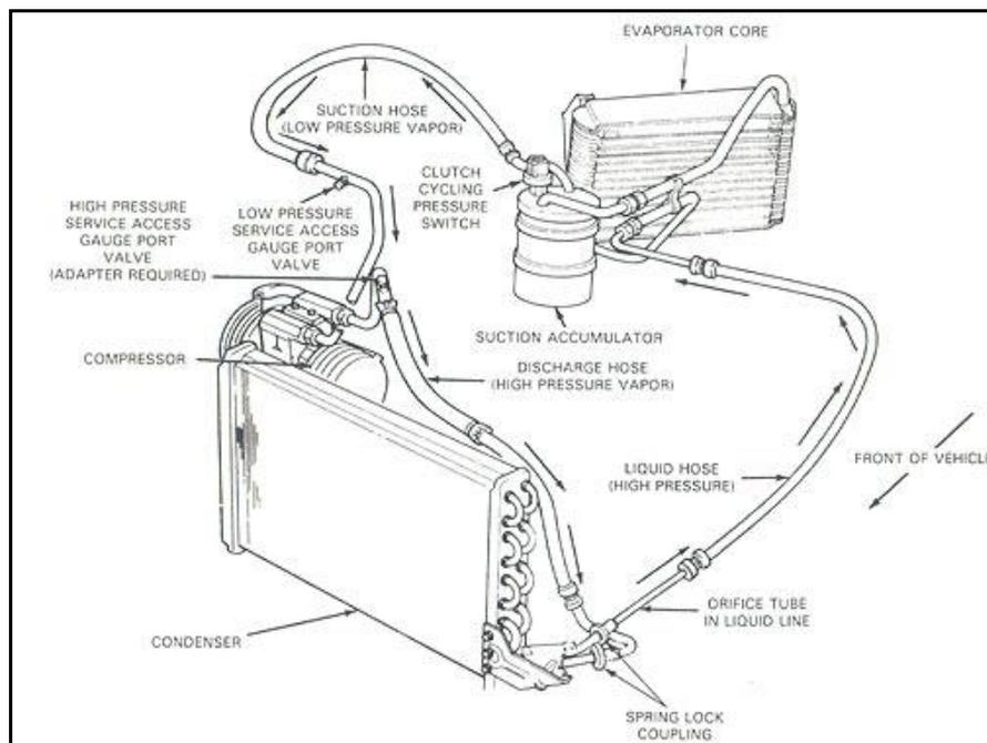
FIGURE 10: COMPLETE AIR-CONDITIONING CIRCUIT DIAGRAM,(EDMUNDS, 2008)
