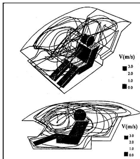
FIGURE 4: THREE DIMENSIONAL PARTICLE TRACK (VELOCITY), (CHIEN ET AL., 2008)
