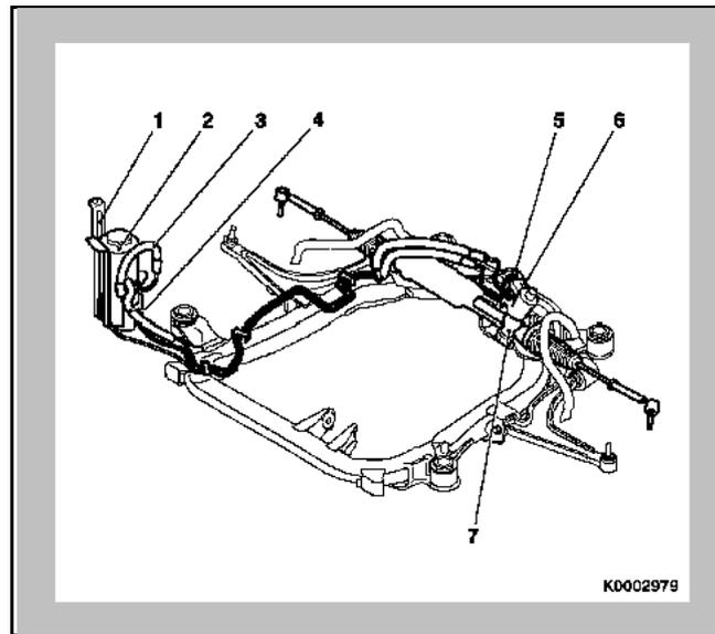
FIGURE 24: EHPAS SYSTEM CONFIGURATION (OPEL MOTORS CO.)
