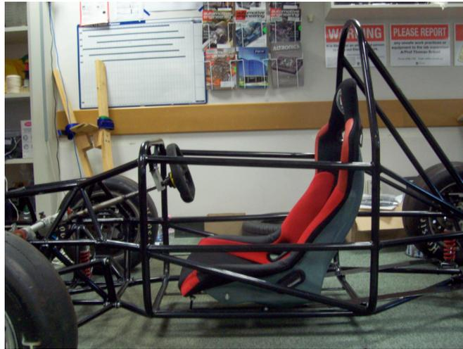
**Figure 2: REV-SAE chassis roll hoops**
