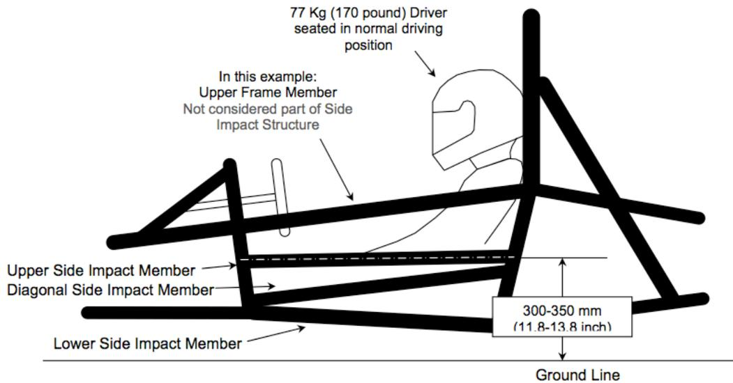
**Figure 3: Side Impact Structure Requirements**
