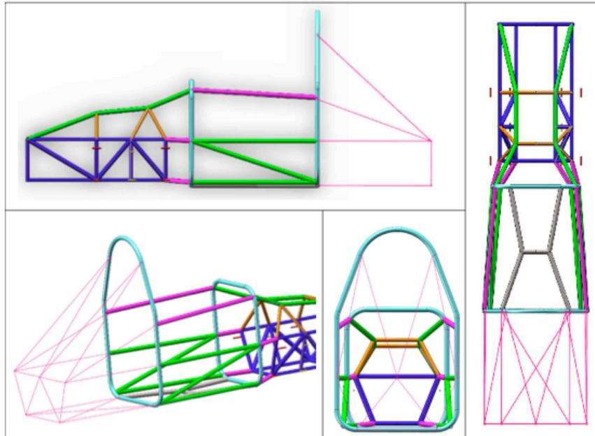
**Figure 9: Modified chassis schematic**
