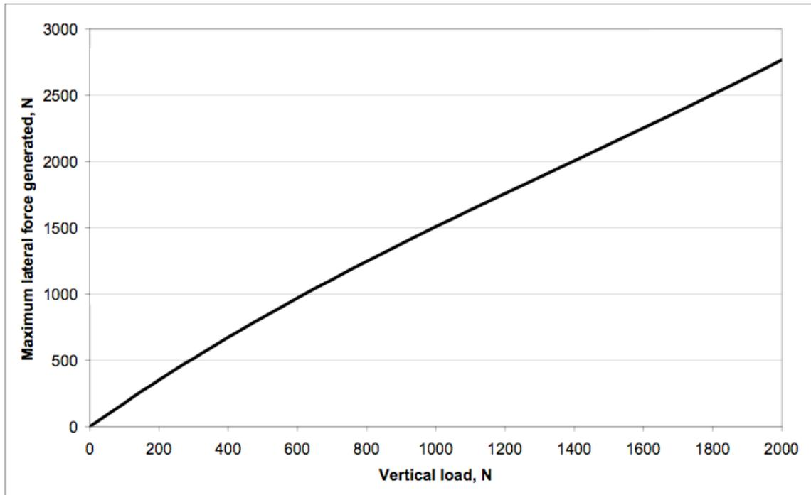
**Figure 5: Non-linear behaviour of a typical Formula SAE tyre**
