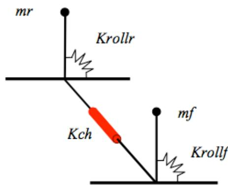
**Figure 6: Idealized chassis for analyzing stiffness**
