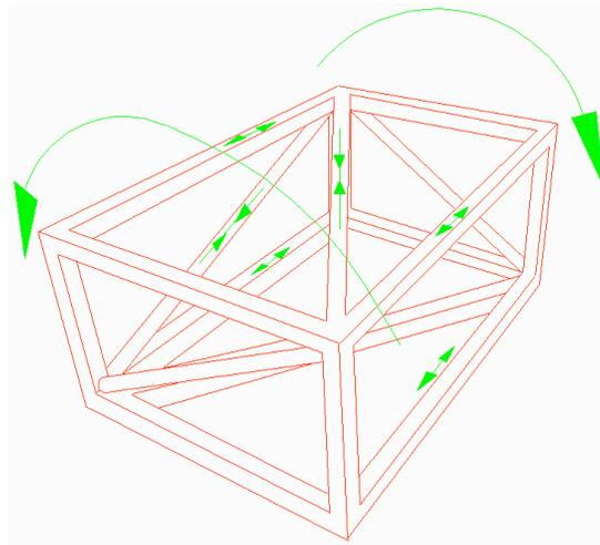
**Figure 4: Ideal space frame displaying loads**
