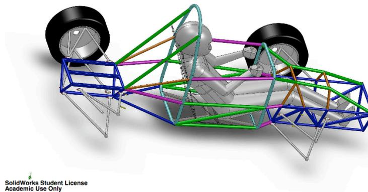
**Figure 7: Rev-SAE chassis rear bay**
