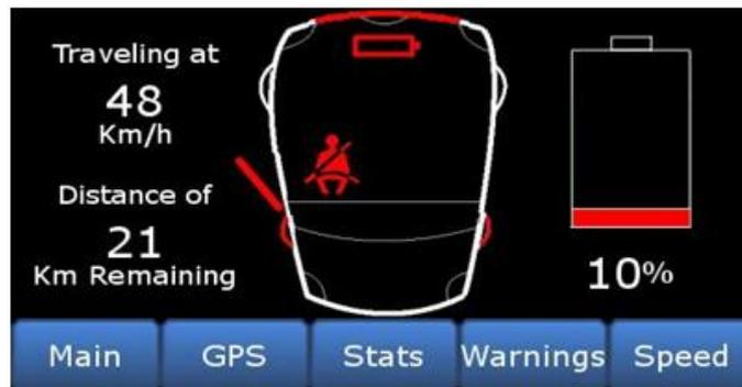
Figure 3.2: Main Screen with Warnings
