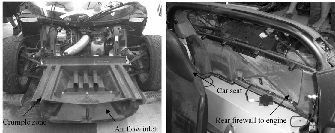
**Figure 16:** Lotus Elise crumple zone (left) and rear firewall behind seats (right).
