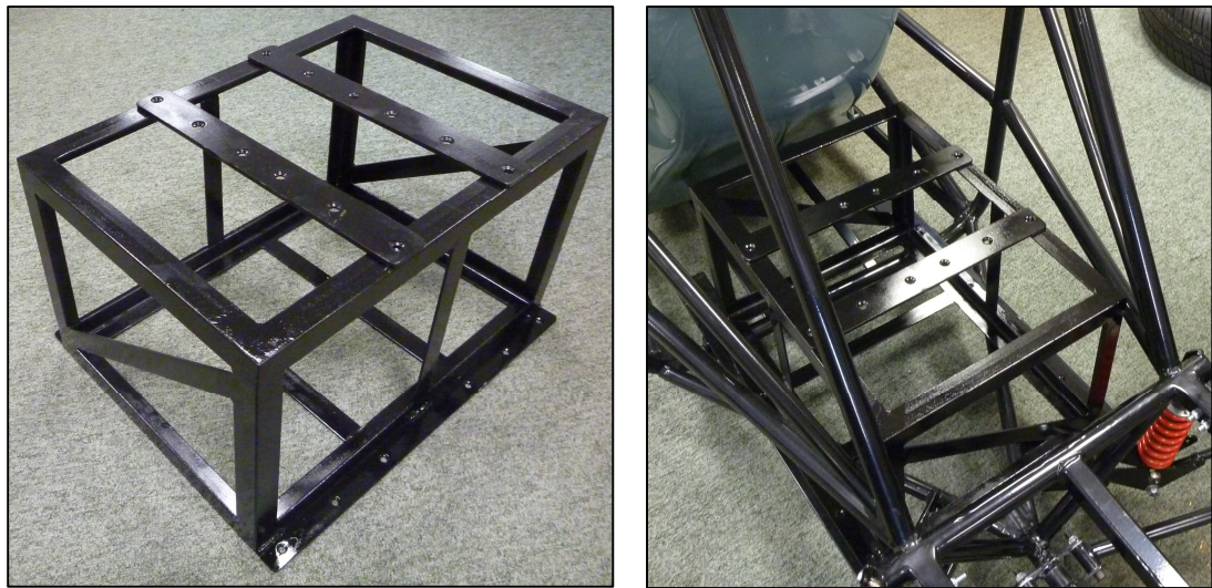
Figure 2.5-1: Left - manufactured battery cage; right – battery cage in its location behind the driver's seat.
