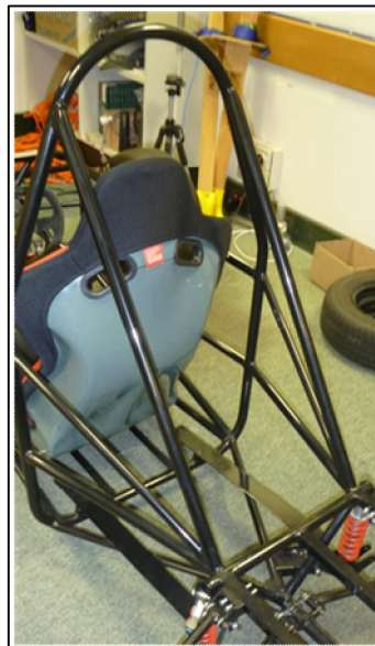
Figure 2.3-1: Proposed battery cage location behind driver seat.
