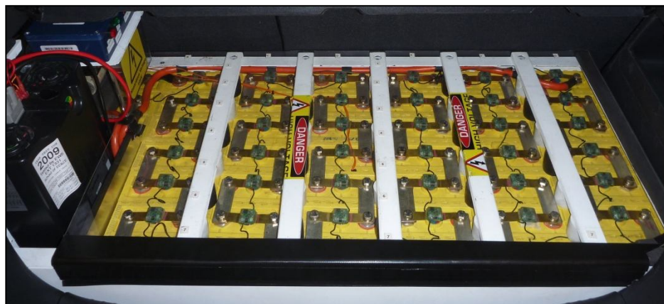
Figure 2.1-1: Getz battery cage in the boot of the vehicle.
