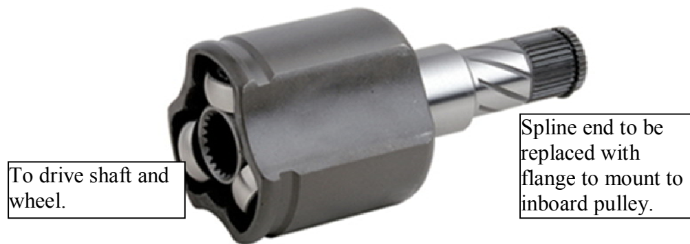
Figure 4.8-2: Inner CV joint modification. (KML Bearing 2009)
