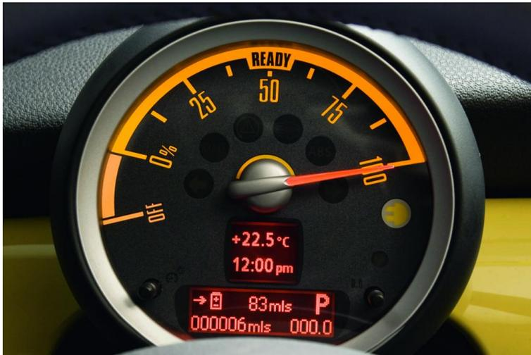
Figure 2.6.: Mini E battery indicator [bmw10]
