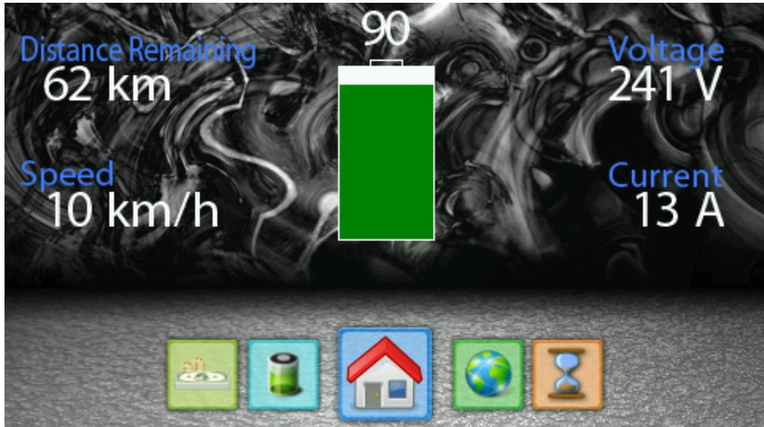
**Figure 6.3: Battery state panel** - Screen-shot of the battery state panel, showing the voltage, current, charge, speed (via gps) and distance remaining
