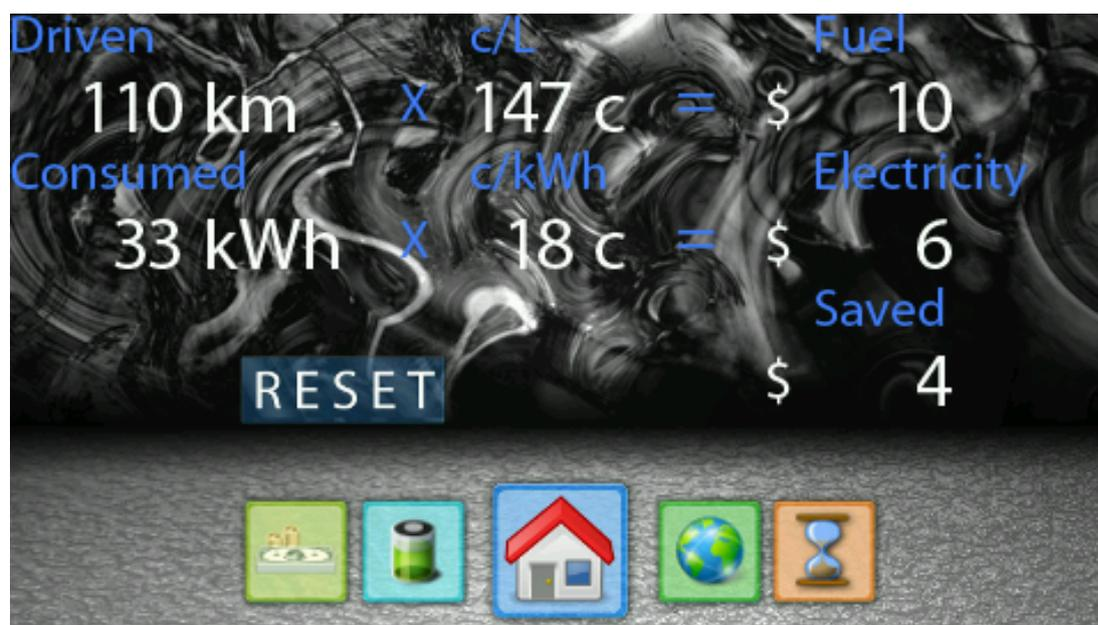
**Figure 6.12: Savings Panel** - This figure shows the savings panel, it calculates the cost of running the car on electricity and approximates the cost of running the car on petrol
