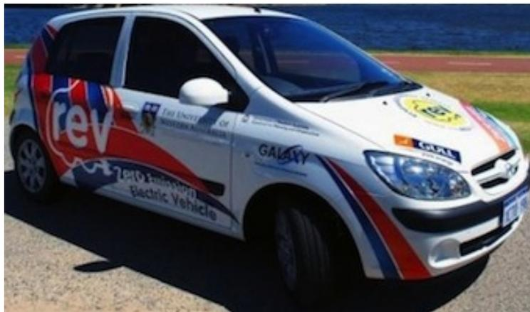
Figure 1: REV Eco : The Converted Hyundai Getz. Source: [<http://therevproject.com/>]
