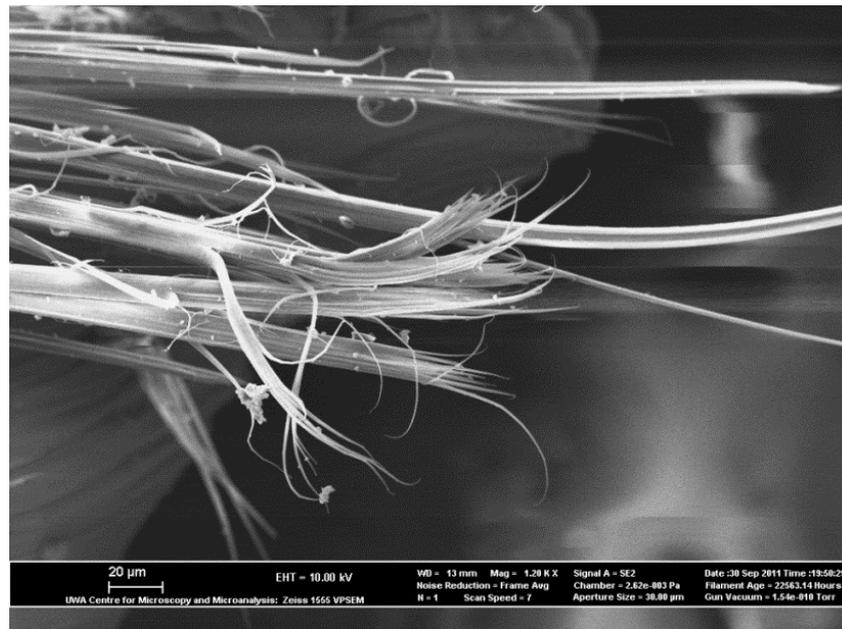
**Figure 19:** Multiple Split Break of Kevlar Fibres
