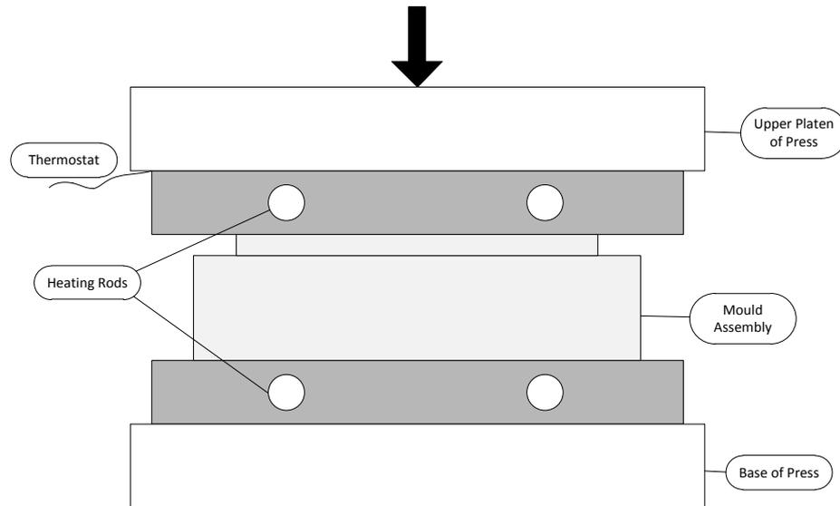
**Figure 11:** Arrangement of Hot Platen Air Press (Figure adapted from Jeyaraman 2010)
