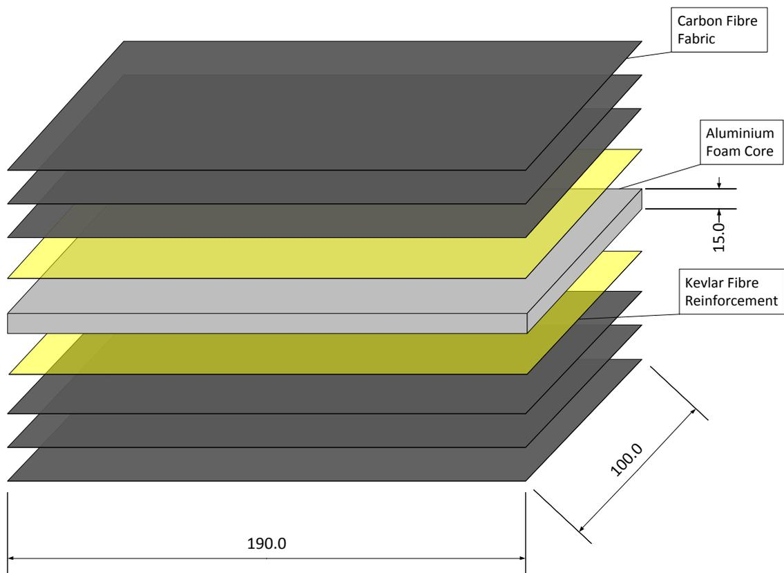
**Figure 10:** Composite Sandwich Structure Assembly
