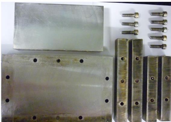
**Figure 6:** Parts of the Mould Assembly
