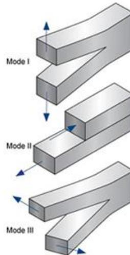
**Figure 3:** The 3 modes of fracture (NDT Resource Centre, 2011)
