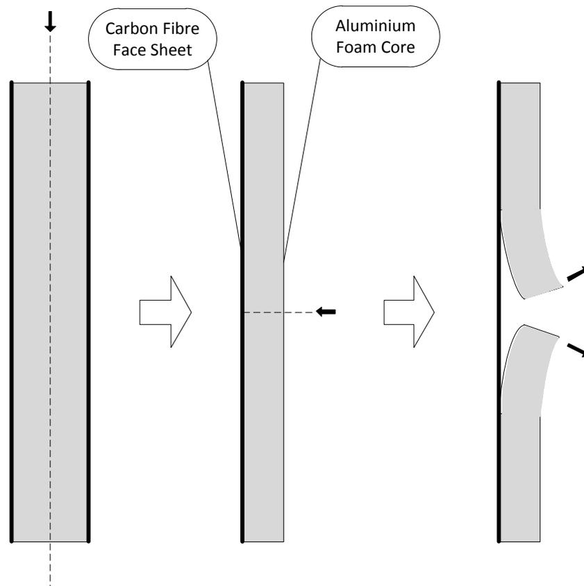
**Figure 14:** Method for Separating Core and Face Sheet
