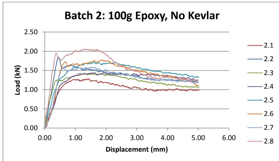
**Figure 17:** Load vs. Displacement for Samples in Batch no. 2
