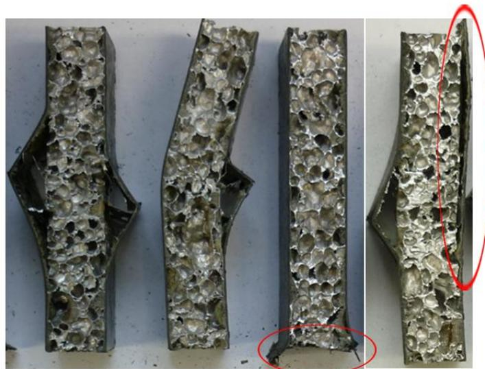
**Figure 18:** Failure mechanisms (From left to right: expected failure at starter crack, “bend effect”, “end effect” and delamination of skin)
