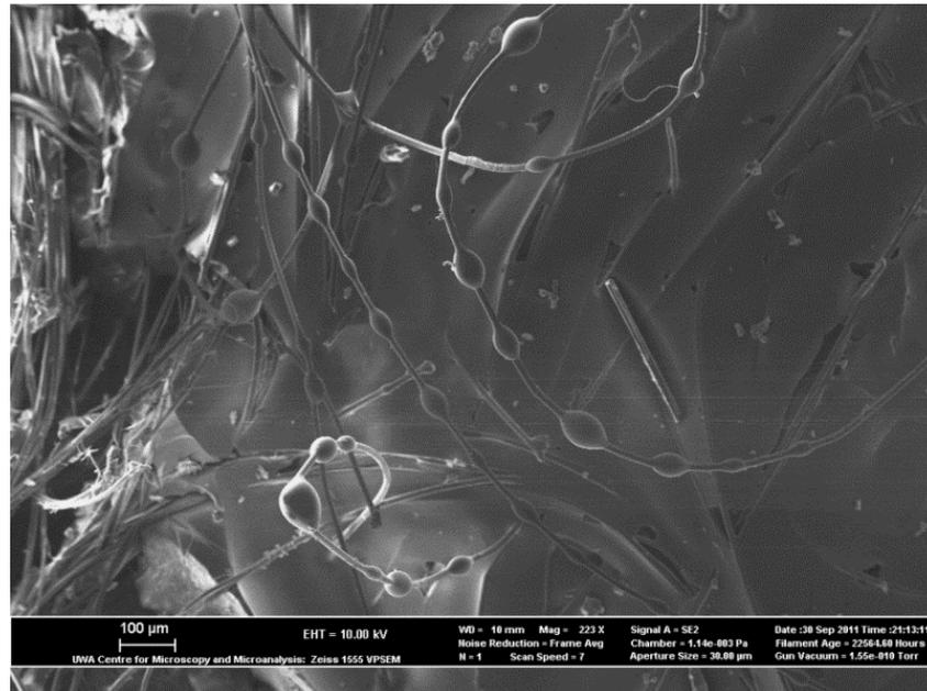
**Figure 21:** Kevlar Fibres Wet with Epoxy
