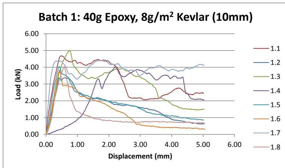
**Figure 16:** Load vs. Displacement with Multiple Peaks
