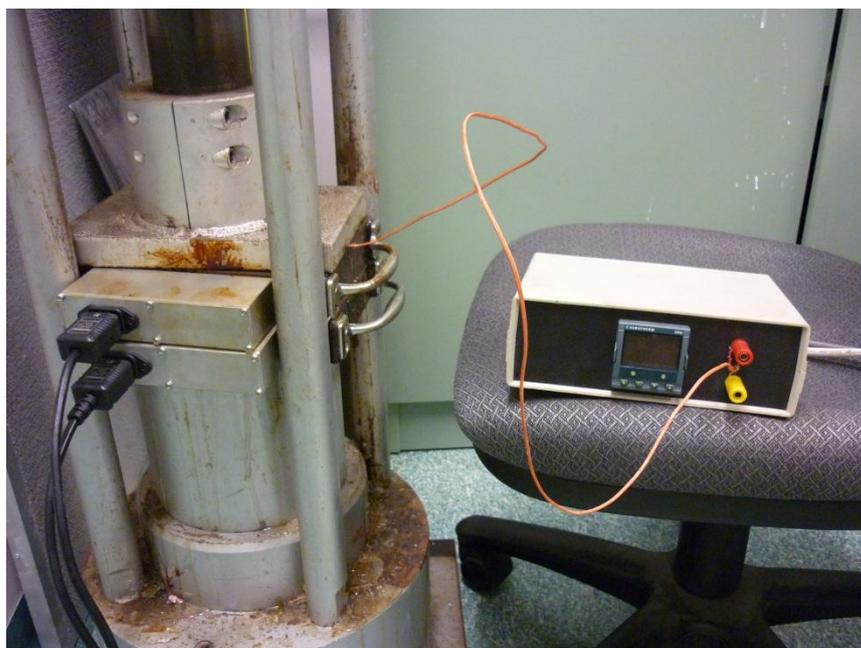
**Figure 26:** Hot Platen Air Press and Eurotherm 2416 PID Controller
