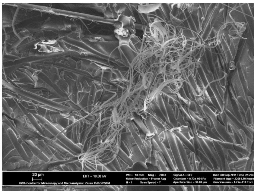
**Figure 20:** Fibrillation and Fibre Pullout Marks
