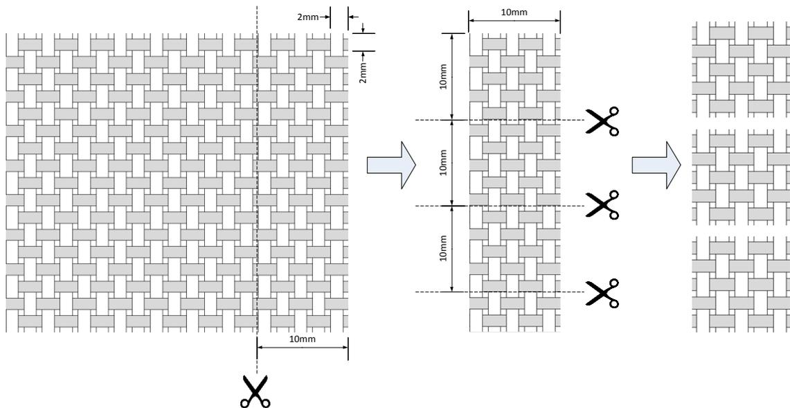
**Figure 8:** Kevlar Cutting Technique
