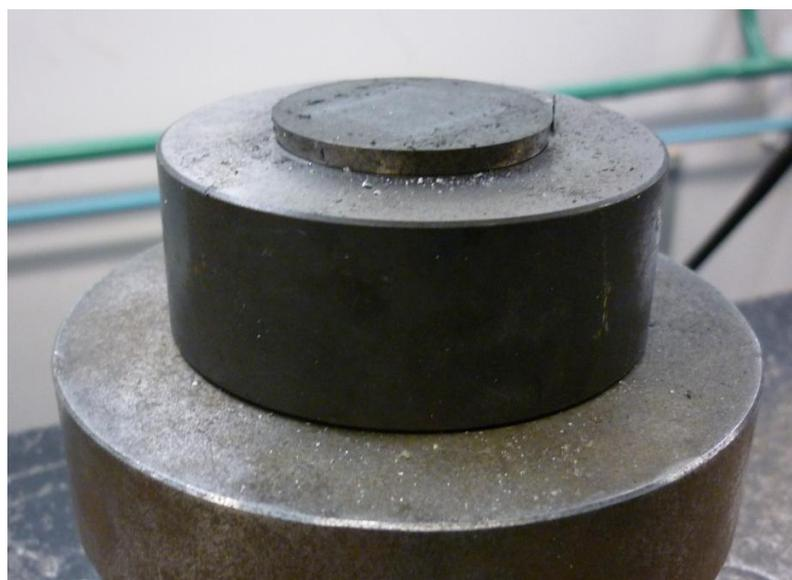
**Figure 25:** Hemispherical bearing used in compression testing
