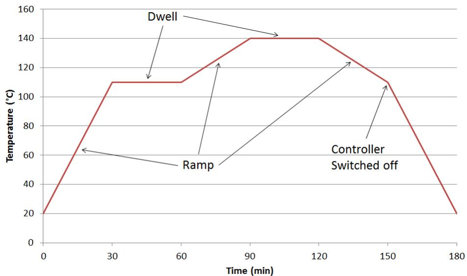
**Figure 12:** Curing Cycle
