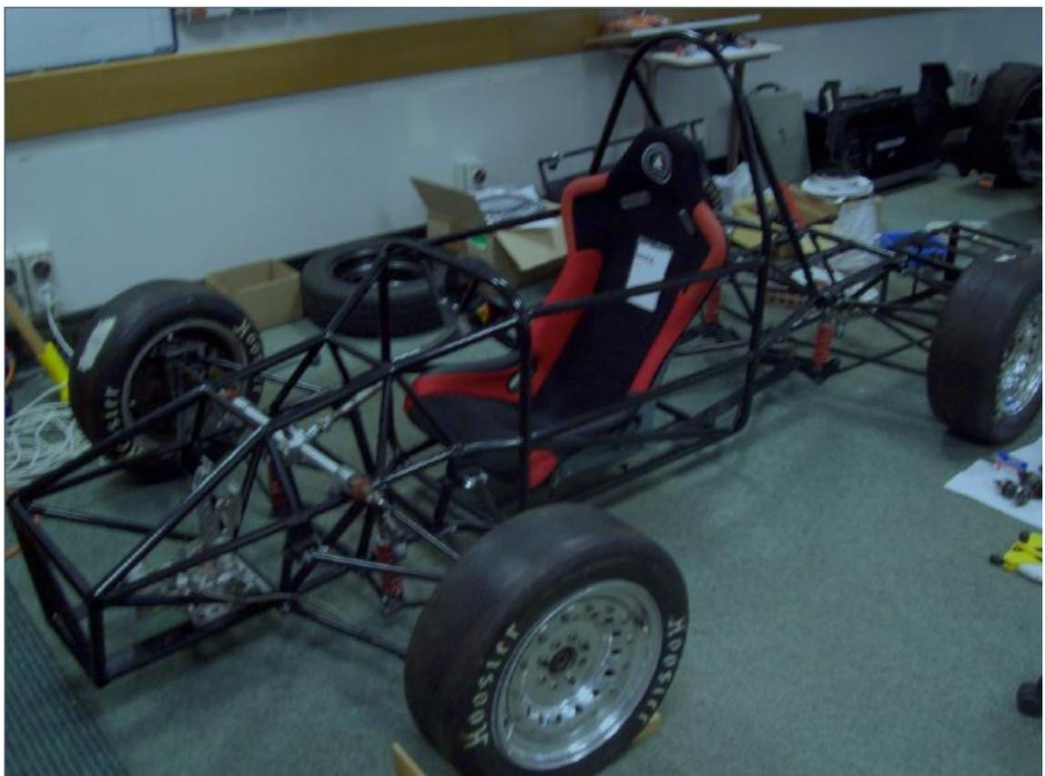
**Figure 3** : 2002 UWAM Rolling Chassis (Powers, 2009)
