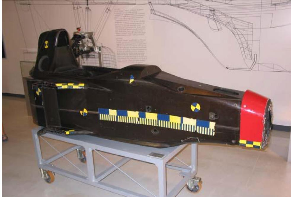
**Figure 11:** Modern carbon fibre monocoque (Bush, 2006)
