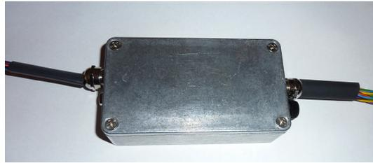
**Figure 3.2:** Instrumentation Control Box
