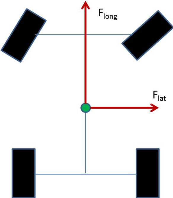
Figure 5.3: Lateral & Longitudinal Forces
