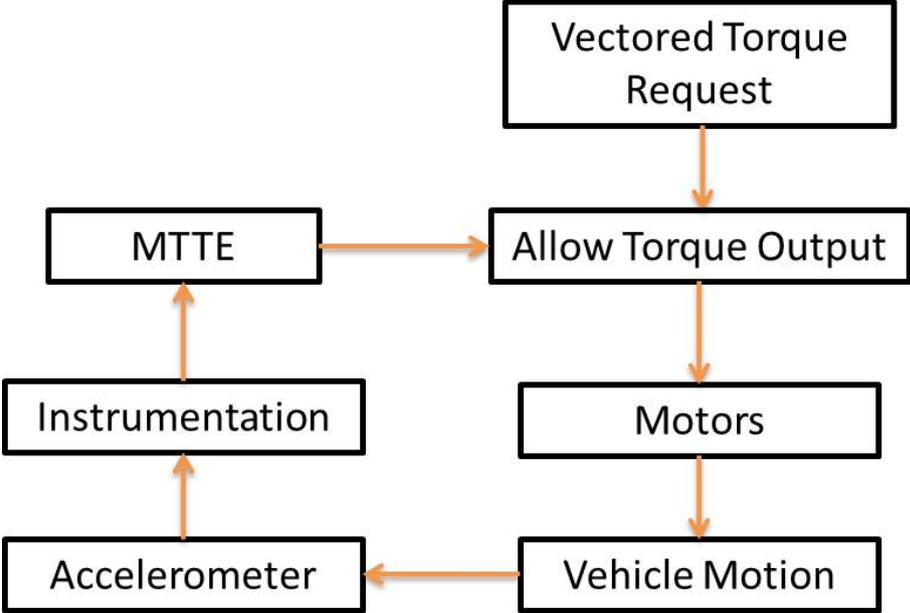
Figure 5.1: Traction Control Process
