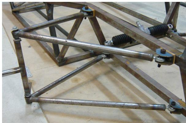
Figure 3.6: Suspension Mounts
