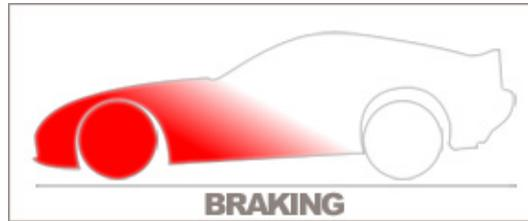
**Figure 5.5:** Longitudinal Load Transfer under extreme braking
