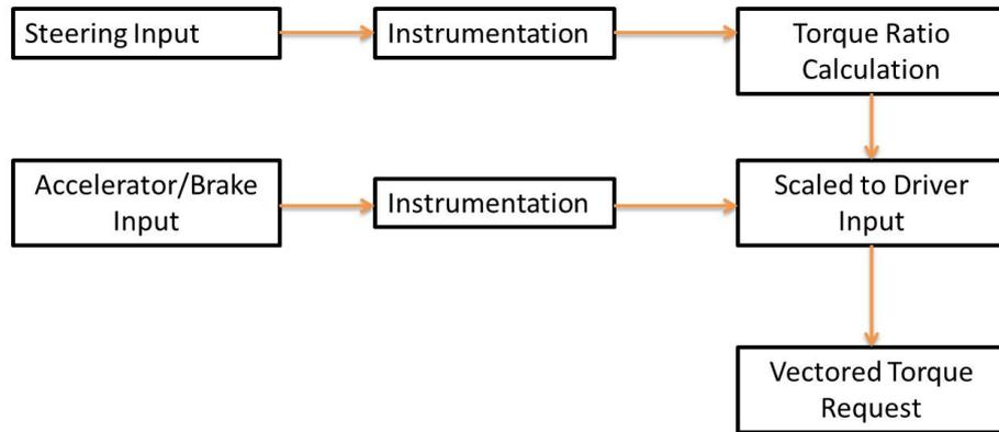
Figure 4.1: Torque Vectoring Flow Diagram
