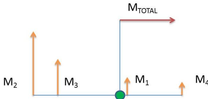
**Figure 4.4:** Torque Vectoring Moment
