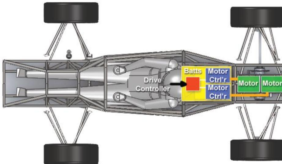
Figure 5 Top view of prototype vehicle showing component locations [7].
