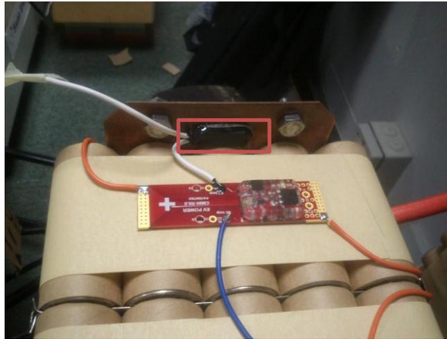
**Figure 27** Temperature switch's location indicated by red box.
