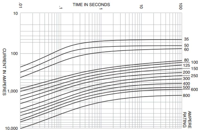
**Figure 16 Time-Current Characteristic Curve of ANN fuses [19].**
