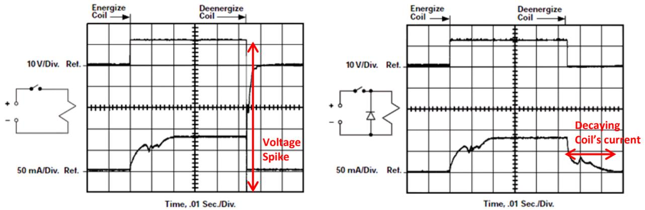
(a) Typical DC relay without diode
