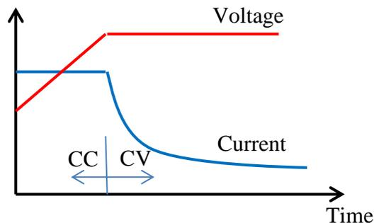
**Figure 14 The characteristic plot of CCCV charger.**
