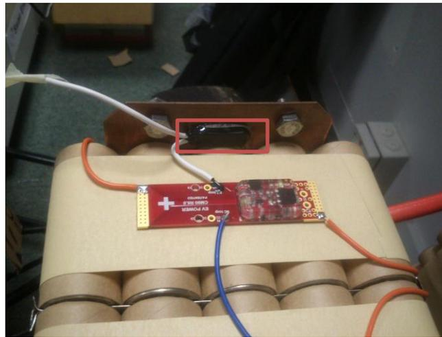
**Figure 27** Temperature switch's location indicated by red box.
