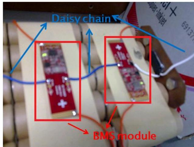
Figure 13 BMS module and its daisy chain.
