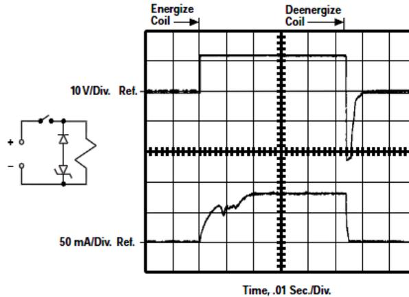
(c) Typical DC relay with diode and Zener
