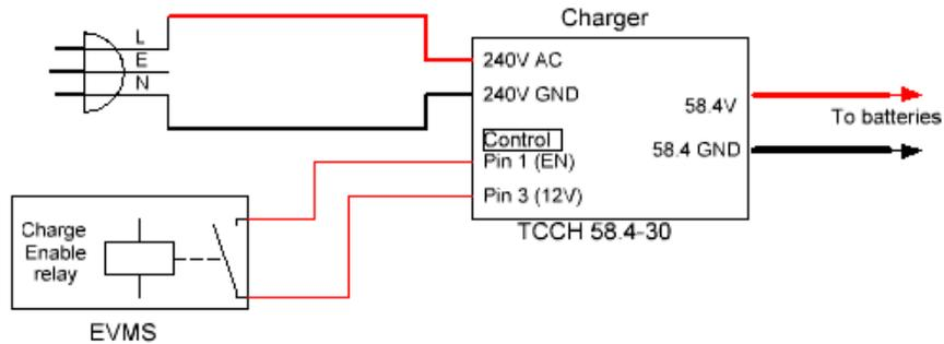
Figure 22 Interface between EVMS and charger
