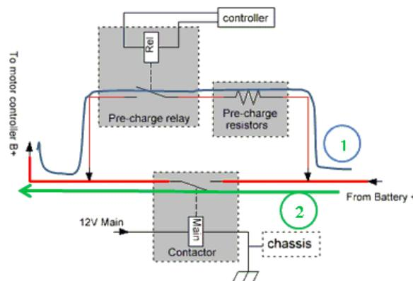
Figure 20 Precharge circuit
