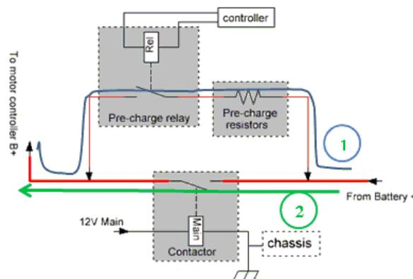
Figure 20 Precharge circuit
