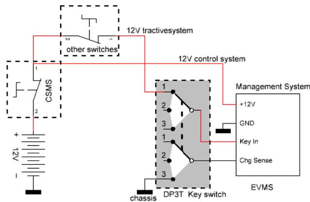
Figure 21 Interface the drive and charge interlock
