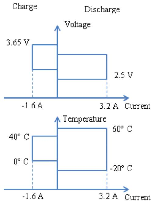
**Figure 11 Safe Operating Area of LiFePO<sub>4</sub> battery cell.**
