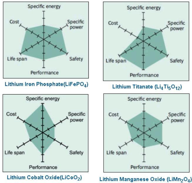
**Figure 10** The relative merit of various Li-ion chemistries [13].
