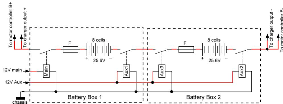
Figure 17 Preliminary design of the tractive system accumulator
