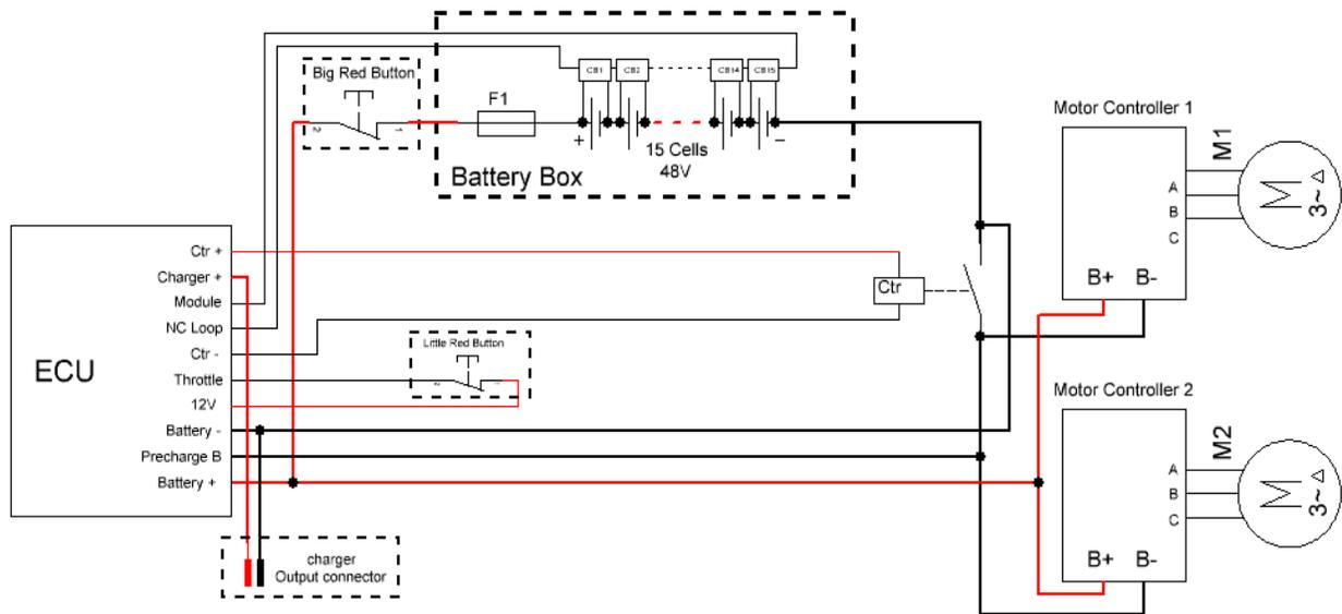
**Figure 6 The schematic of the electrical system of the prototype vehicle.**
