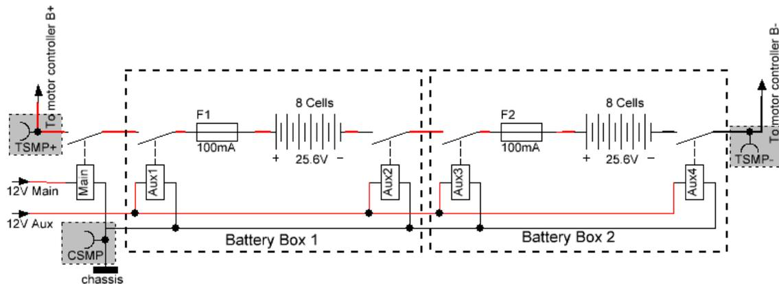
Figure 24 Battery box schematics showing measuring points
