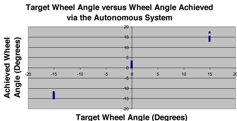
Figure 30: Graphical spread of the autonomous system's steering repeatability.
