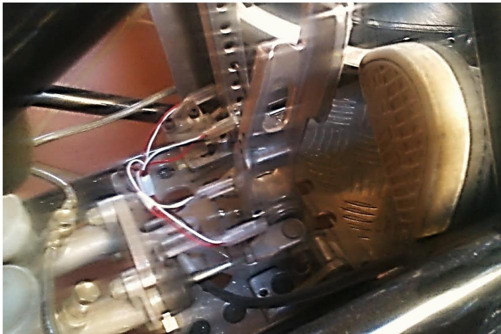
Figure 9: The brake pedal of the Formula SAE vehicle. The beige object is the shoe of a driver.
