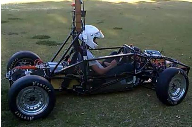
Figure 1: Formula SAE-Electric vehicle.
