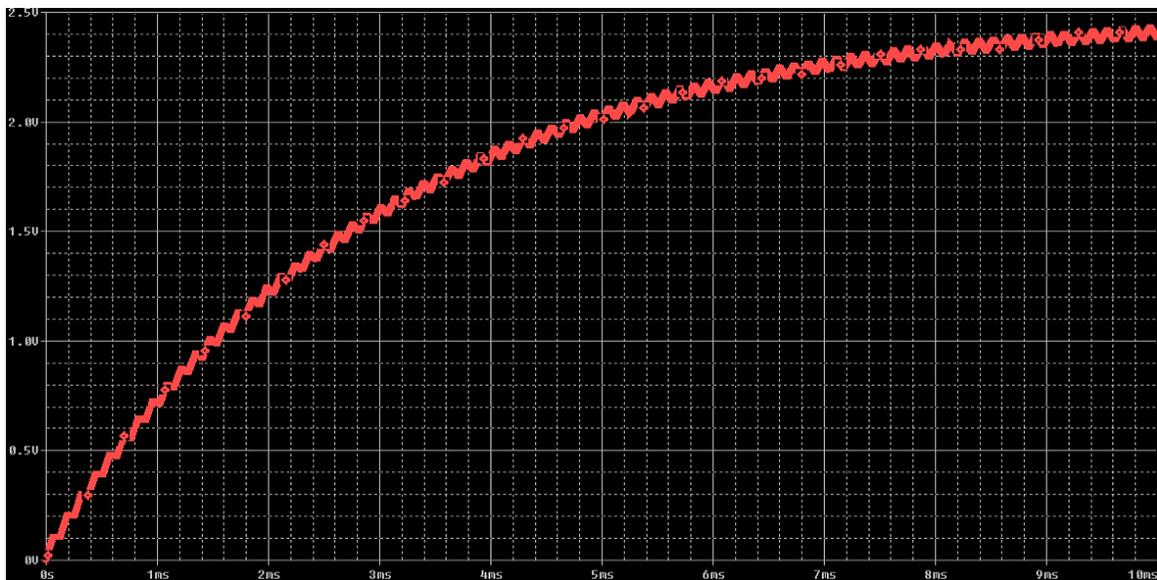
Figure 18: Output signal of the circuit in Figure 17 with a 50% input PWM duty cycle.
