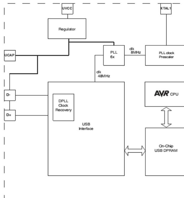
Figure 32: The diagram of the USB communication circuit located inside the ATMEGA16U2 on the Arduino board ([40], page 185).
