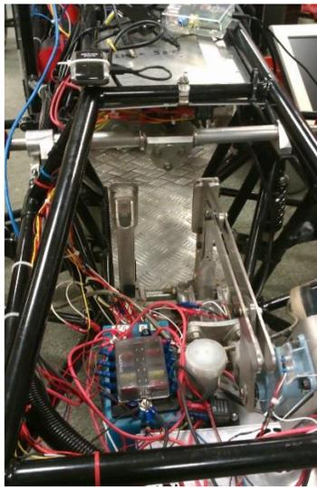
Figure 33: The nose of the vehicle which houses most of the low-level autonomous system. The brake mechanism is shown on the right with numerous electronic circuits housed in the blue box on the left.
