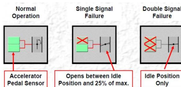
Figure 6: Operational states of engine throttle of Toyota's 2<sup>nd</sup> generation Electronic Throttle Control System-intelligence [14].
