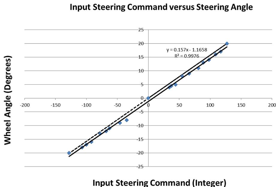
Figure 29: Data for measuring the linearity of the autonomous steering system and vehicle heading (courtesy of Thomas Drage). The dashed line represents the ideal, linear relationship.
