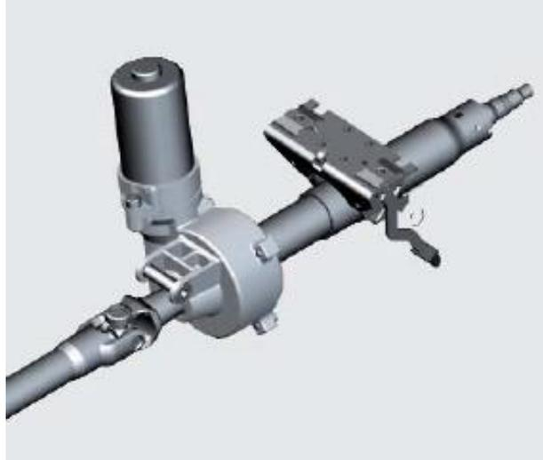
Figure 4: An electric motor (the vertical cylinder) provides steering assistance by driving the steering column [7].
