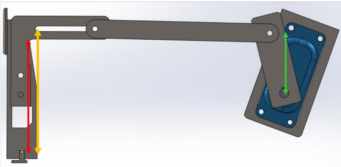
Figure 13: Measurements for design of the brake-by-wire linkage.
