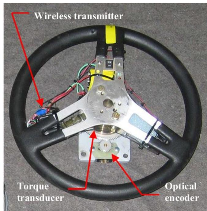
Figure 7: Steering wheel with position and torque feedback sensors [15].
