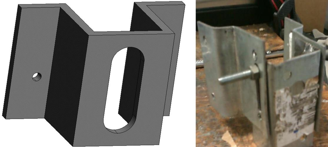
Figure 20: The initial bracket design to house the steering feedback sensor (left), with the final bracket shown on the right.
