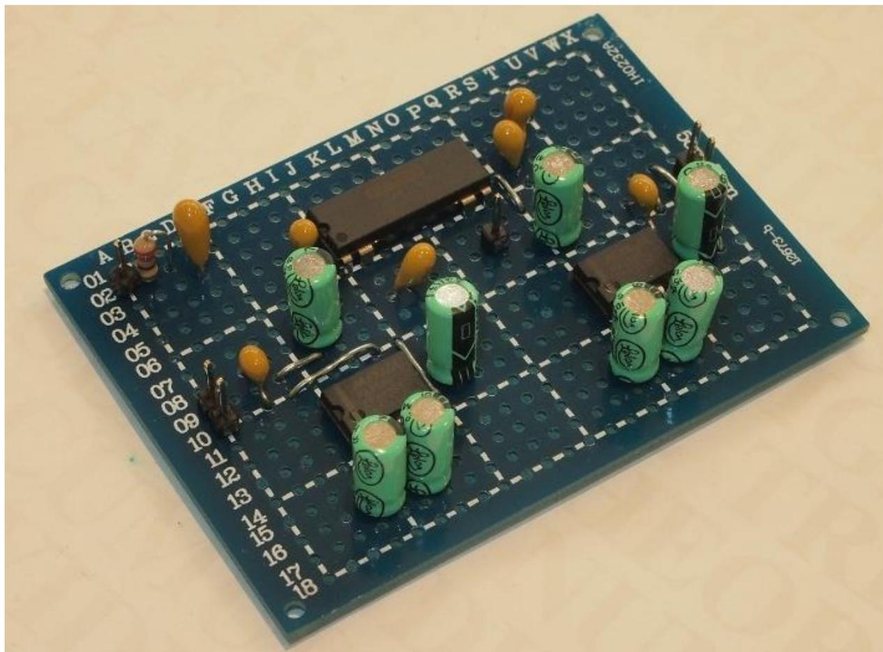
Image of the throttle-by-wire isolation amplifier system courtesy of Thomas Drage. The filter for the Arudino's PWM signal can be seen on the upper left of the board.
