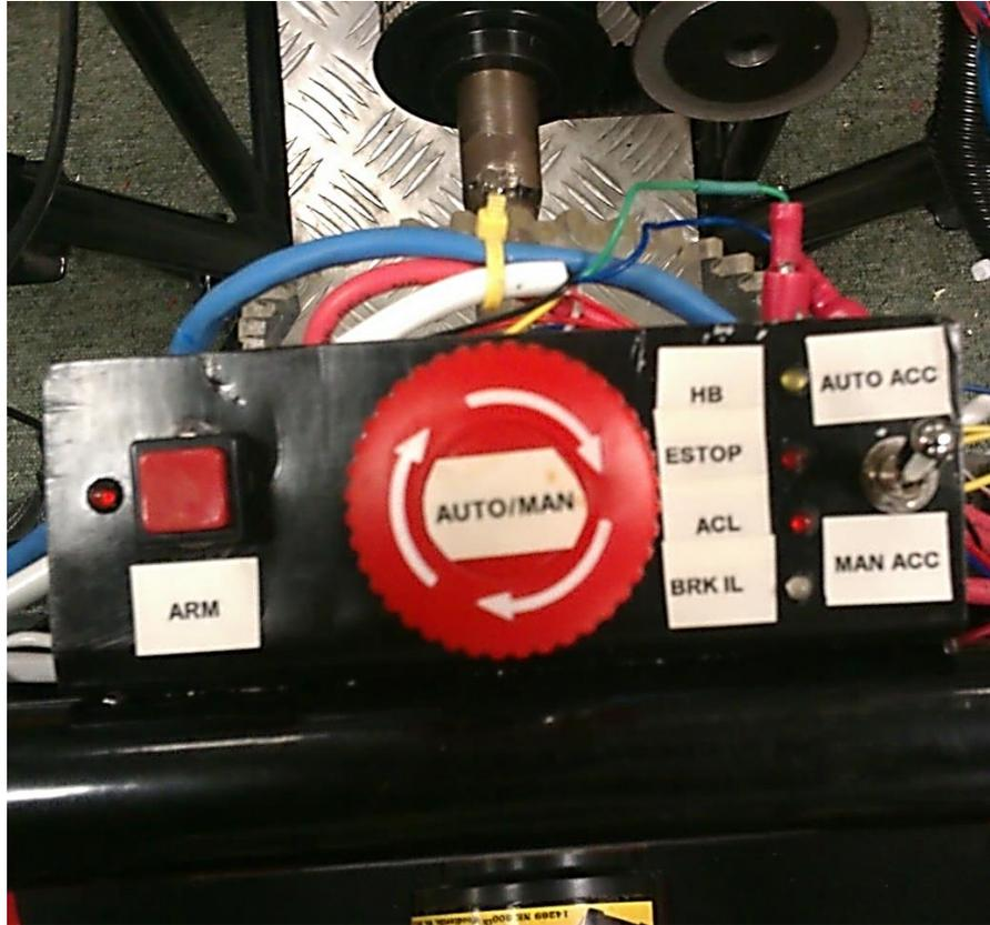
Figure 35: The interface between the driver and the low-level autonomous system. Components of the safety supervisor circuit designed by Thomas Drage are also present.
