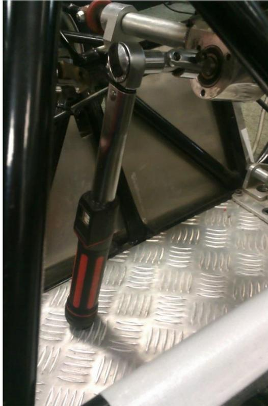
Figure 24: Method used to measure the torque required to turn the wheels of the SAE vehicle.
