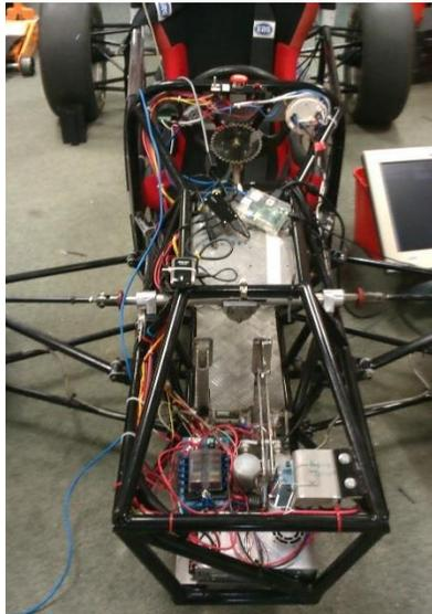
Figure 2: Formula SAE vehicle with drive-by-wire components installed.
