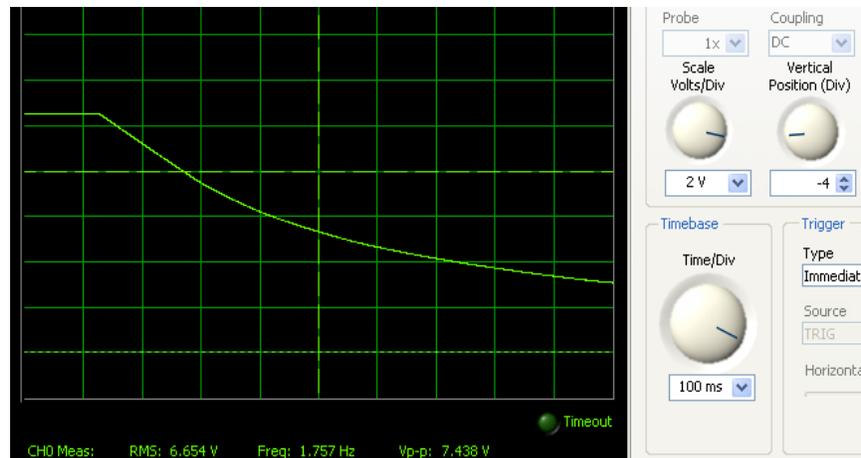
Figure 34: Voltage decay caused by the capacitance of the SSPS-105 servomotor.
