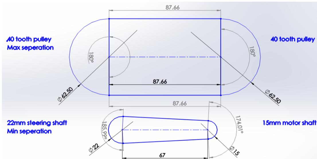
Figure 26: A Solidworks sketch used to determine the maximum and minimum belt lengths possible for use in the steering system.
