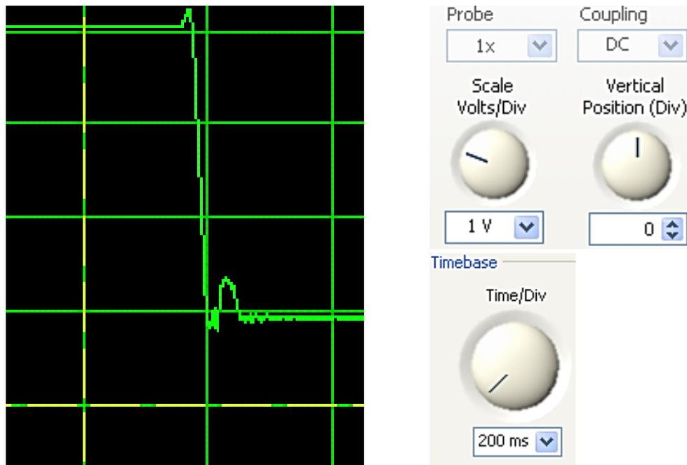
Figure 14: Measurement of the throttle hall sensor from full acceleration to no acceleration.
