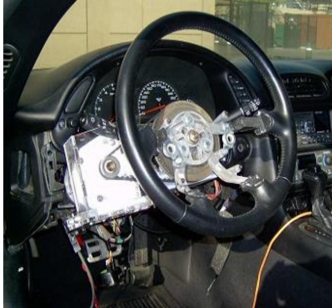
Figure 8: Modified steering setup for actuation by an electric motor [16].
