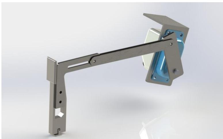
Figure 12: CAD Drawing of the final brake linkage used for the brake-by-wire system.
