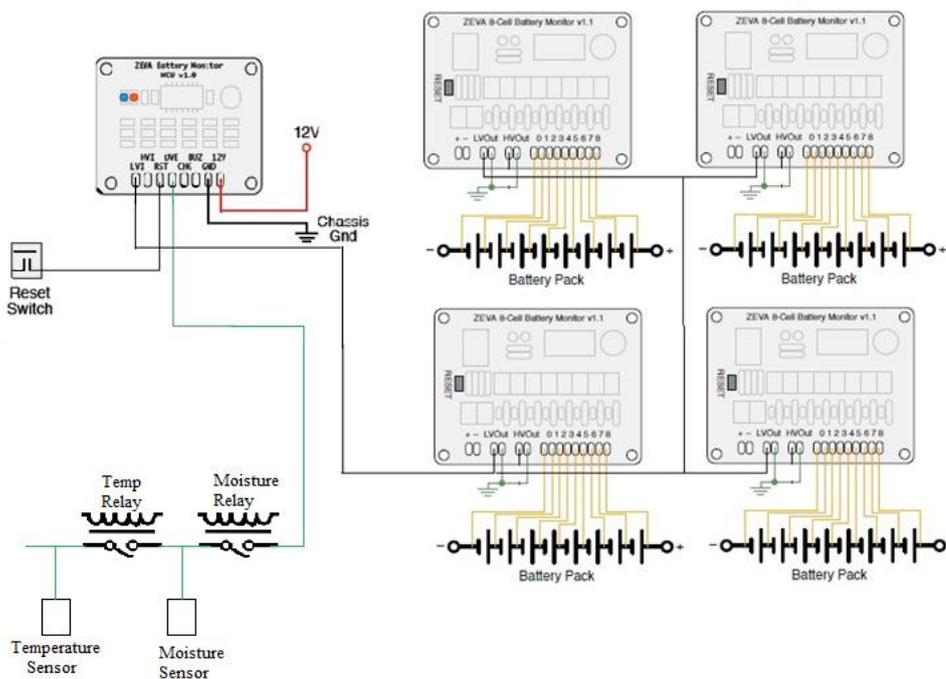
Each of the modules at every node shall be connected to a single battery module input numbered 0 through to 8. As per the module wiring diagram figures 25 to 27, low current wires shall be used in order to make these connections to each of the monitor module. To maintain a minimum ingress protection rating of IP65 as stipulated in the design scope section 3.8, waterproof connectors will be used to minimise the risk of moisture exposure. These waterproof connectors can be seen below:
