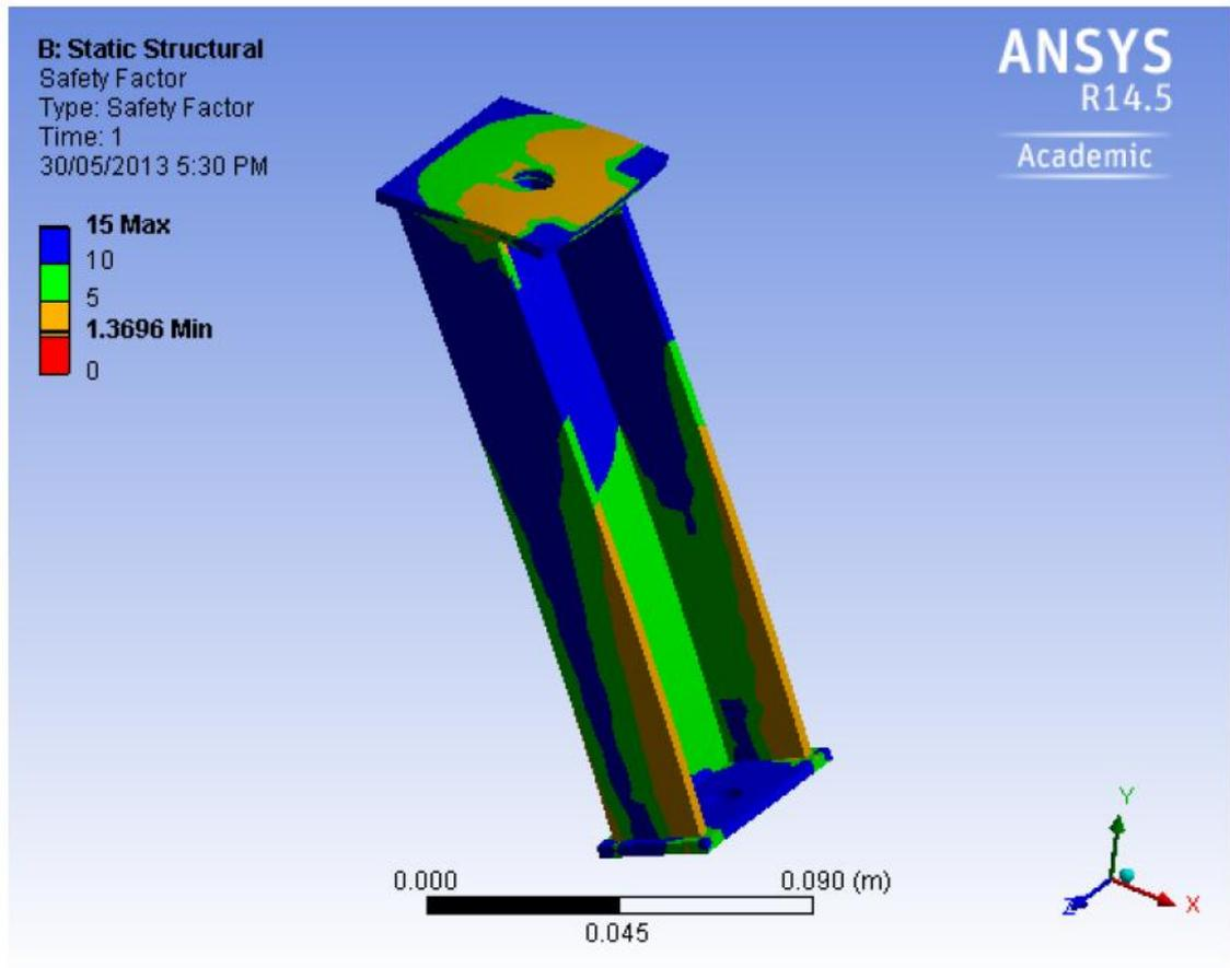
**Figure 16:** Safety factor analysis for the auxiliary mounting platform supports.
