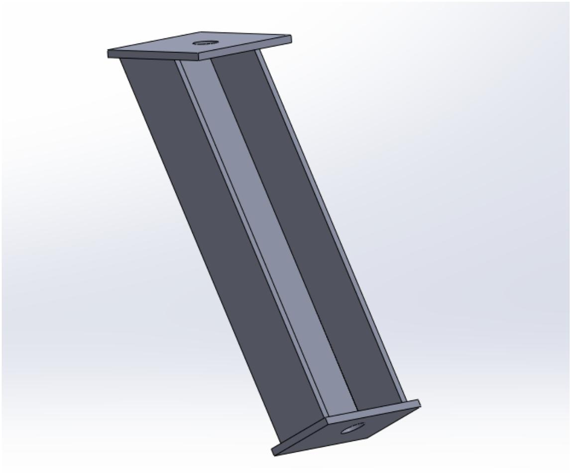
**Figure 12:** Support for auxiliary mounting platform for mounting components within the REVjet
