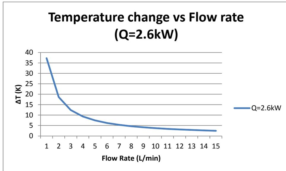
**Figure 4:** Relationship between flow rate and temperature change of coolant
