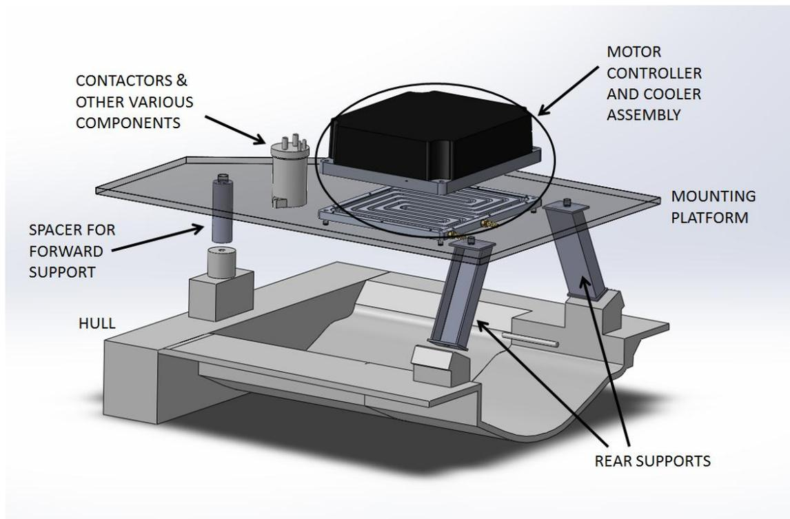
**Figure 18:** Model image of the auxiliary mounting system designed for the REVjet
