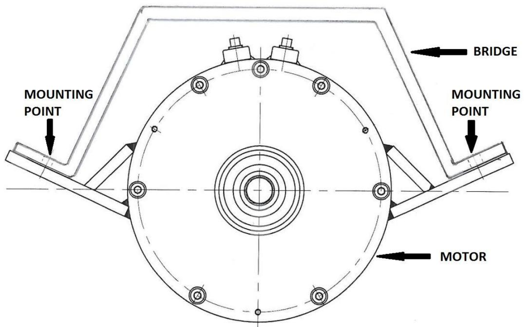
**Figure 9:** Simple flat bar bridge for mounting components above the motor in the REVjet
