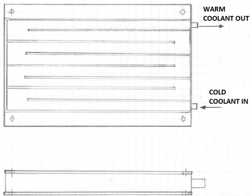
**Figure 7:** Sheetmetal cooling plate
