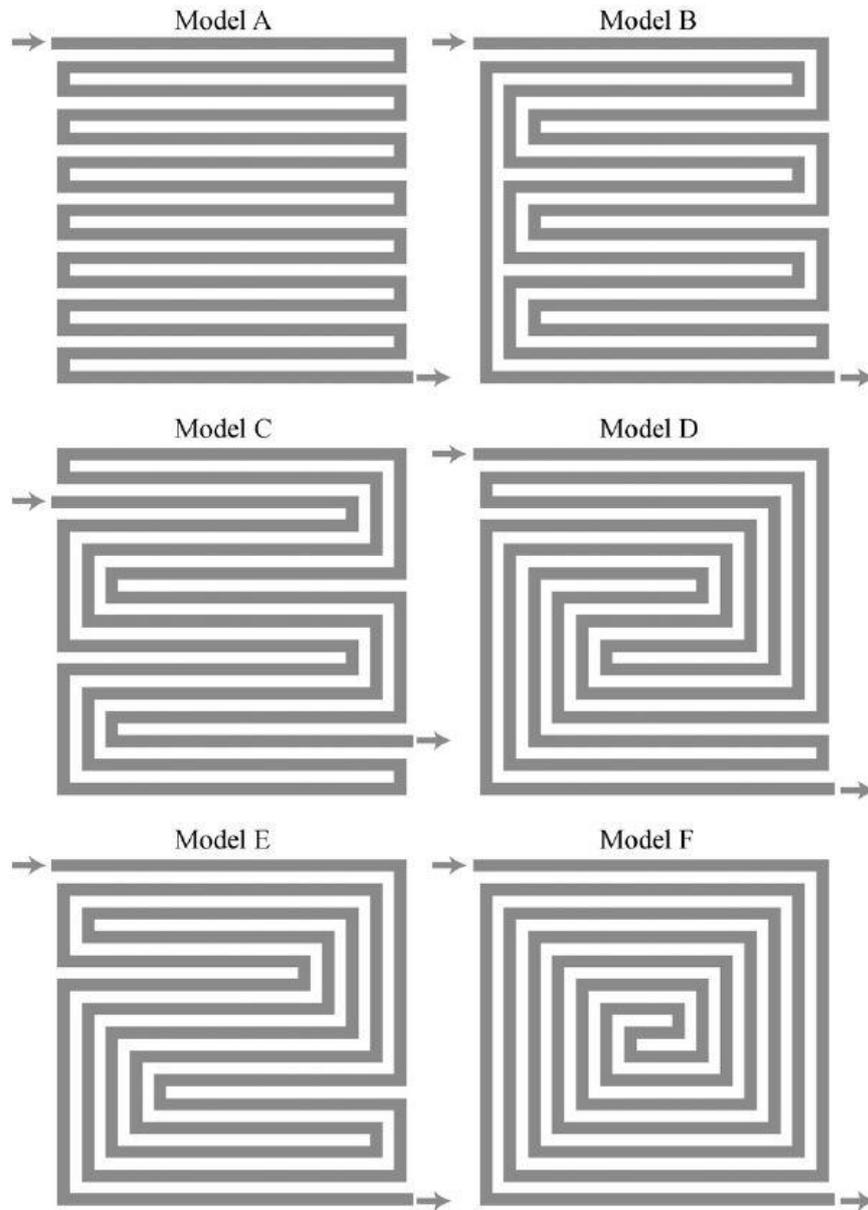
**Figure 6:** Configurations of flow channels in cooling plates analysed by Yu et al. (2009)
