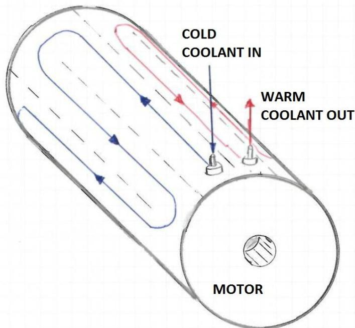
**Figure 3:** Illustration of the electric motor and its cooling jacket for the REVjet
