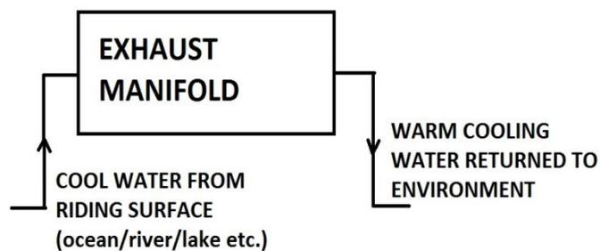
**Figure 2:** Representation of open loop system cooling configuration as used in the exhaust system of the Sea-Doo jetski
