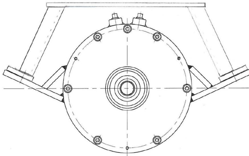
**Figure 11:** Bridge with channel sections for mounting components above the motor in the REVjet
