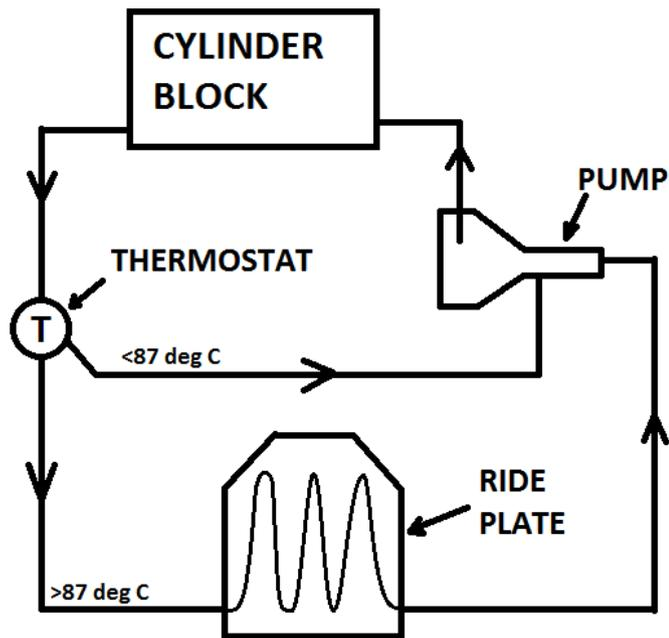
**Figure 1:** Existing cooling system for the internal combustion engine on the Sea-Doo jetski
