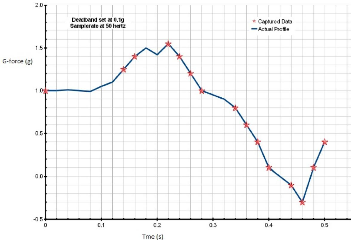
Fig 11 demonstrates the effect of the dead band setting. In fig 11 it can be seen that the dead band is specified by the user as 0.1g and the data sampling rate specified to be 50Hz. The red
