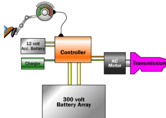
Figure 1 AC induction motor system
