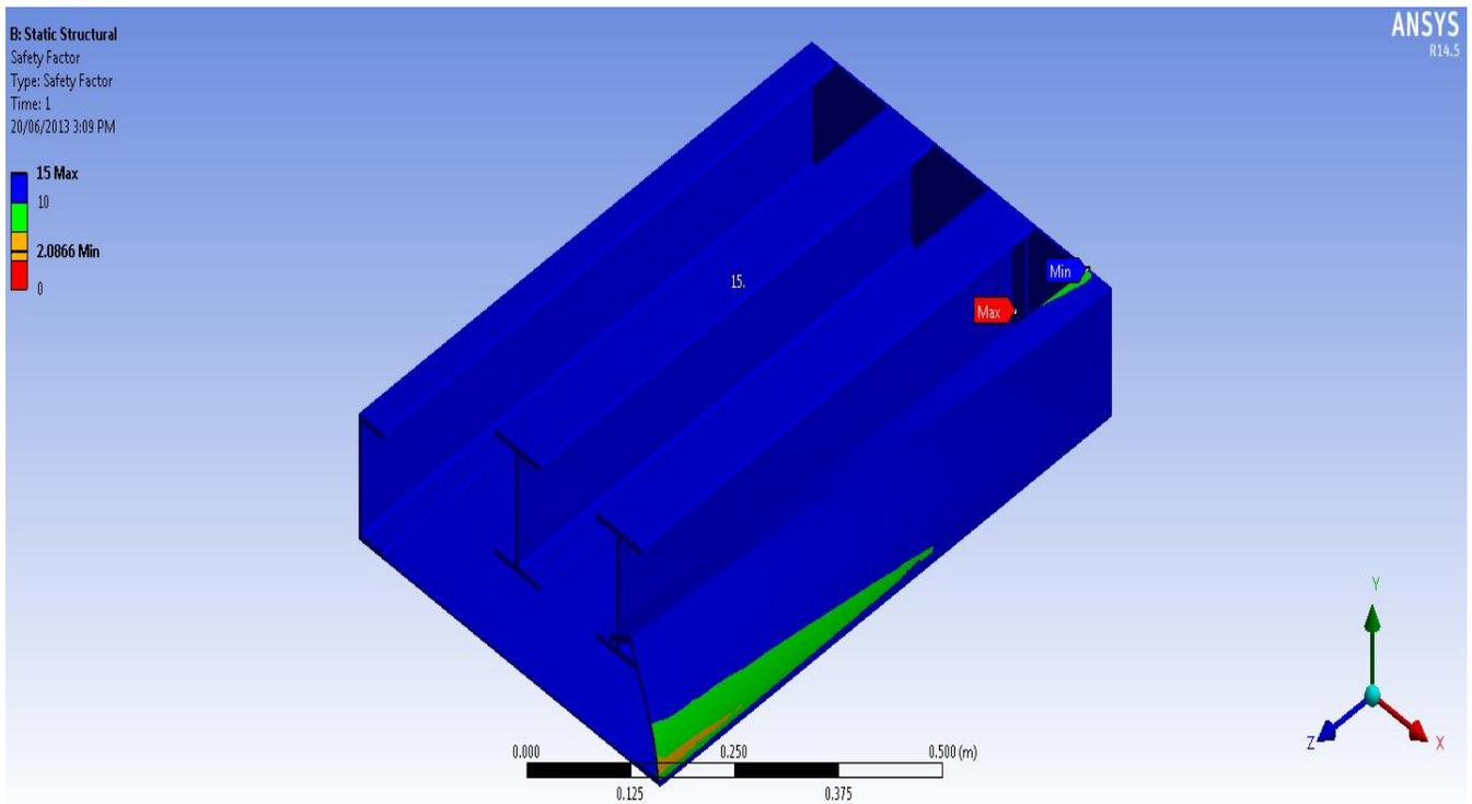
Figure 35 Safety factor, side impact, layer 1
