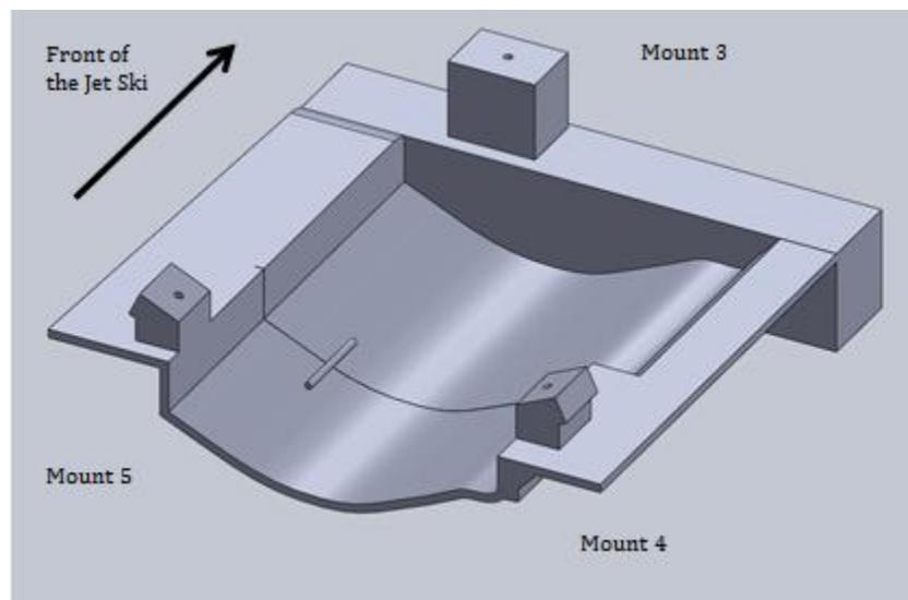
Figure 7 Surface model of the aft section
