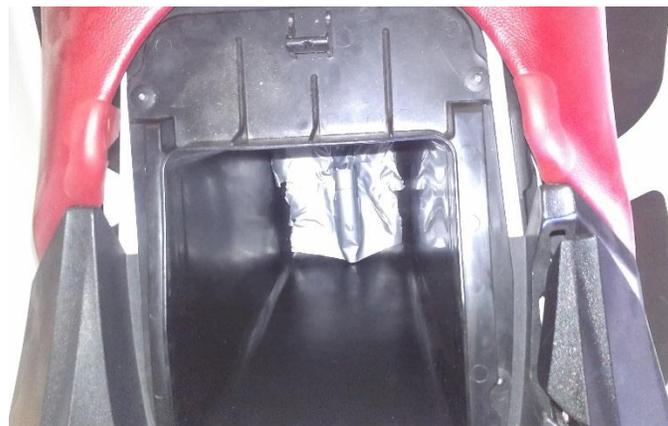
**Figure 9 Mounting point for the accelerometer**
