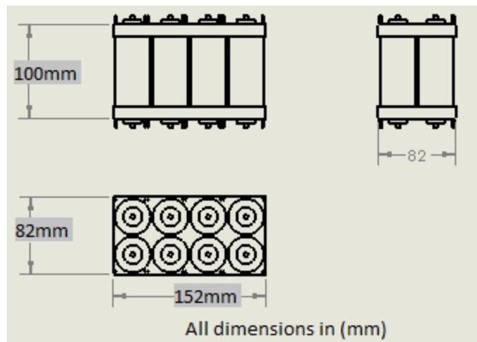
Figure 22 Dimensions for the battery module
