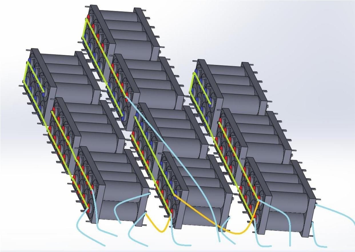
**Figure 24 Initial battery module arrangement**
