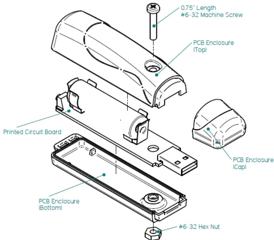
Figure 14 Accelerometer assembly
