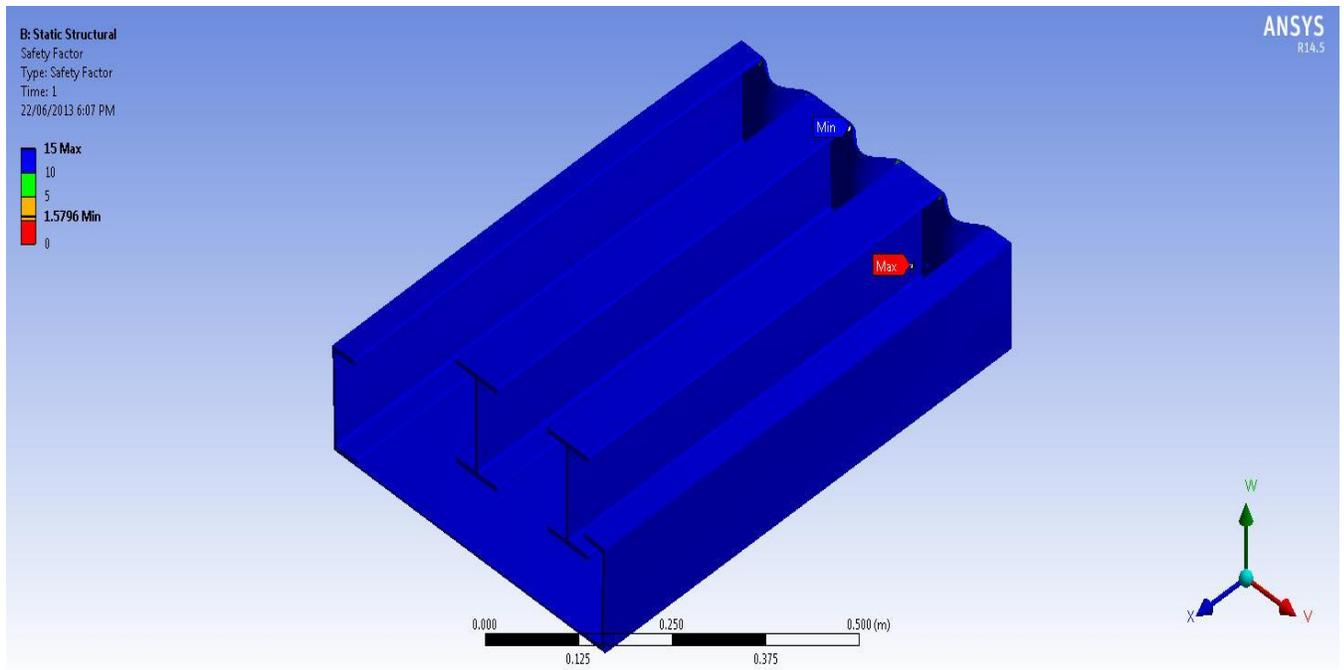
Figure 33 safety factor, front impact, layer 1
