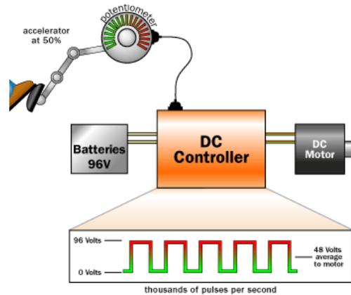
**Figure 2 DC motor system**
