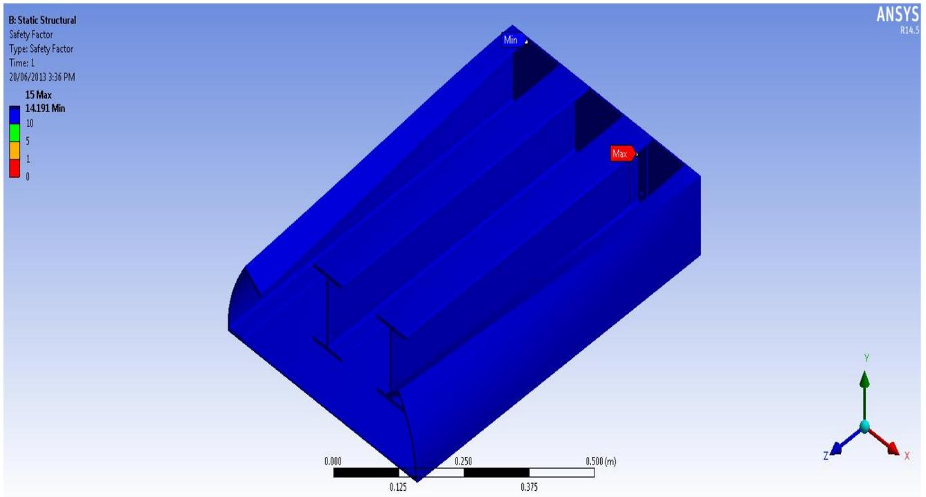
Figure 37 Safety factor, vertical impact, layer1
