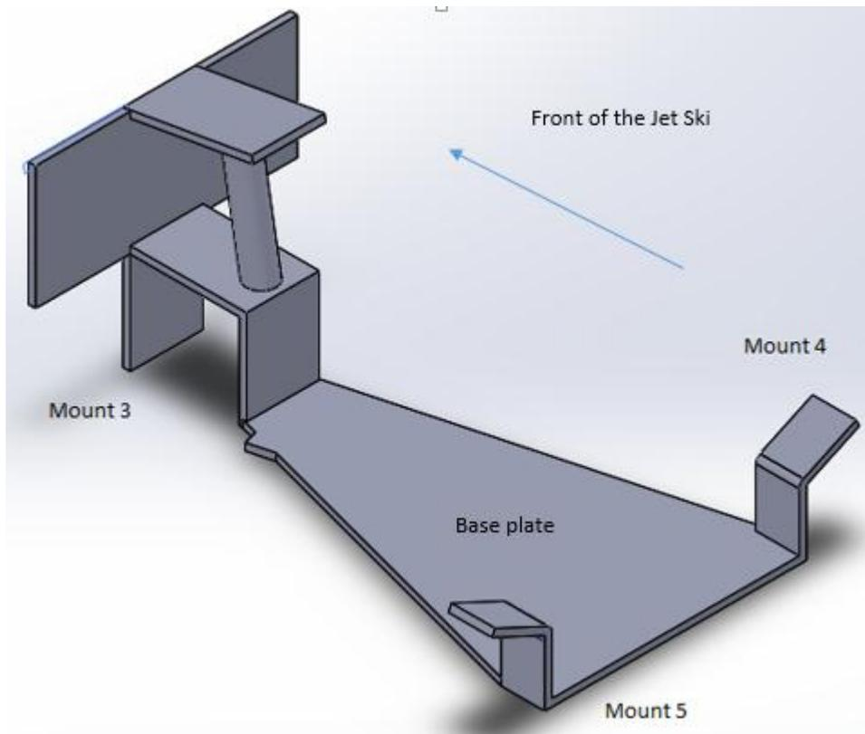
**Figure 44 Initial design for the motor mounting system**
