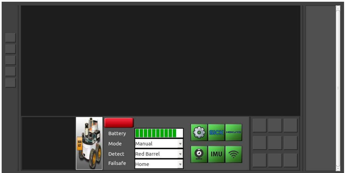
**Figure A4** Graphical interface version 4, non-functional purely a layout and visual design. Colour palette had to be abandoned as to be compatible with the rqt framework.
