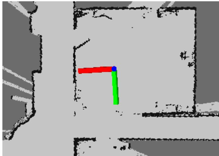
**Figure 2.2** A robot using SLAM to map an environment with the boundaries shown in black and free space shown in grey. The localised robot position is shown in the centre, displayed in red and green. (Kohlbrecher, 2012).
