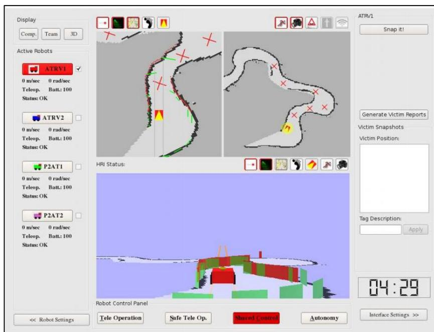
**Figure 1.3** A multi user, multi robot interface developed in 2010 by the University of Rome La Sapienza. Demonstrated in the screenshot is a user controlling a single robot by setting multiple waypoints (Gomez, 2010).
