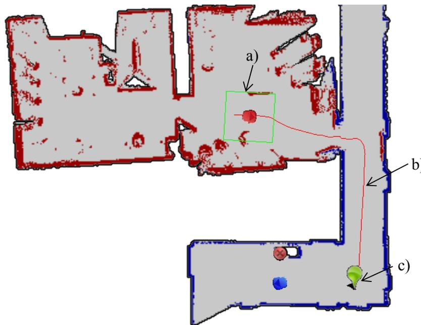
**Figure 3.7** The Map Module demonstrating the navigation features. The robot is traveling along a path to a user defined goal. a) robot is selected, b) calculated path is displayed c) goal icon is displayed.
