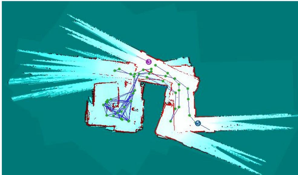
**Figure 2.4** A screenshot showing Map Building failing to fuse two robot maps.
