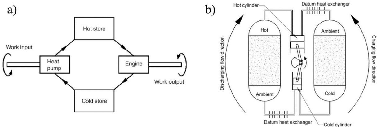
Figure 12 - a) simplified flow diagram of a PHES system, b) simplified schematic of an energy storage system
