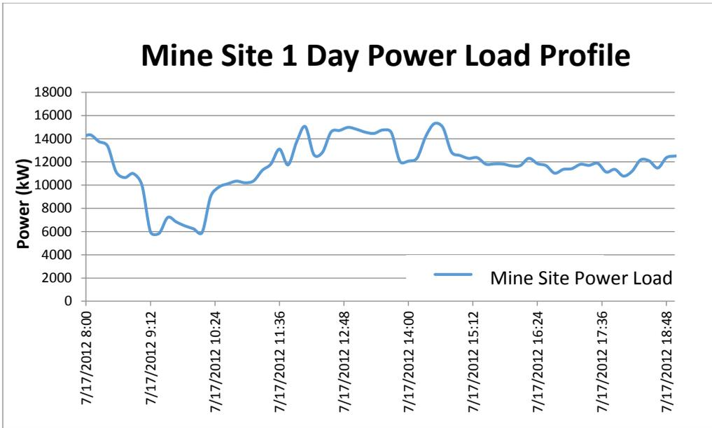
Figure 1 – Power Load Profile for a Mine Site over 1 Day
