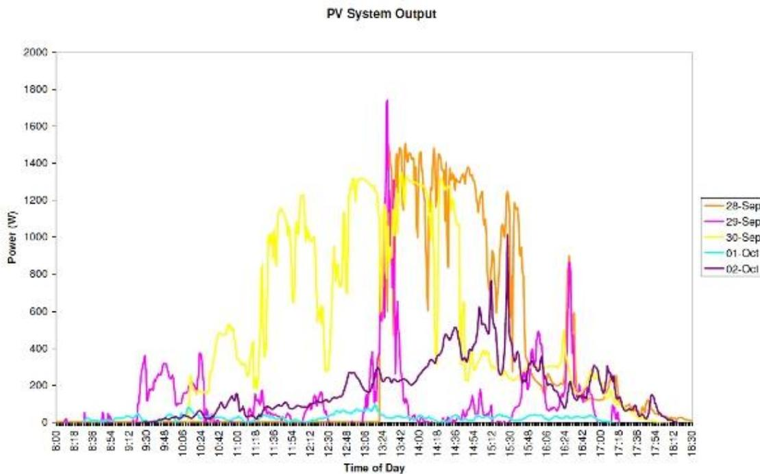
Figure 2 - Power Output Profile for a PV System over 1 day
