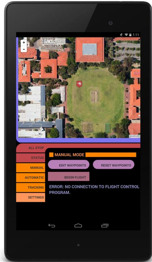
Figure 7: The final user interface, rendered on a Nexus 7 Android tablet. The user interface is shown waiting in ‘Manual Mode’, waiting for a connection to the hexacopter.
