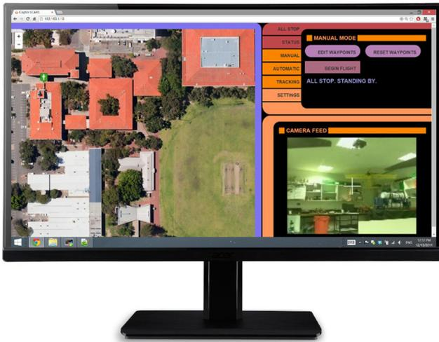
**Figure 8:** The final user interface, rendered on a Windows 8 machine through Google Chrome. The interface is shown waiting in ‘Manual Mode’ for user instructions. A camera feed (showing the research lab) is shown.
