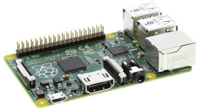
**Figure 4: The Raspberry Pi Model B+ is a credit card sized computer capable of running the Linux operating system. (The Register, 2014 [64])**
