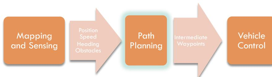
FIGURE 2 - CONTROL SOFTWARE FLOW
