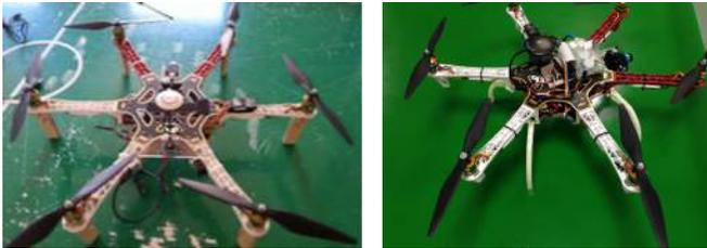
Figure 13: Old landing gear (left) and new landing gear (right)
