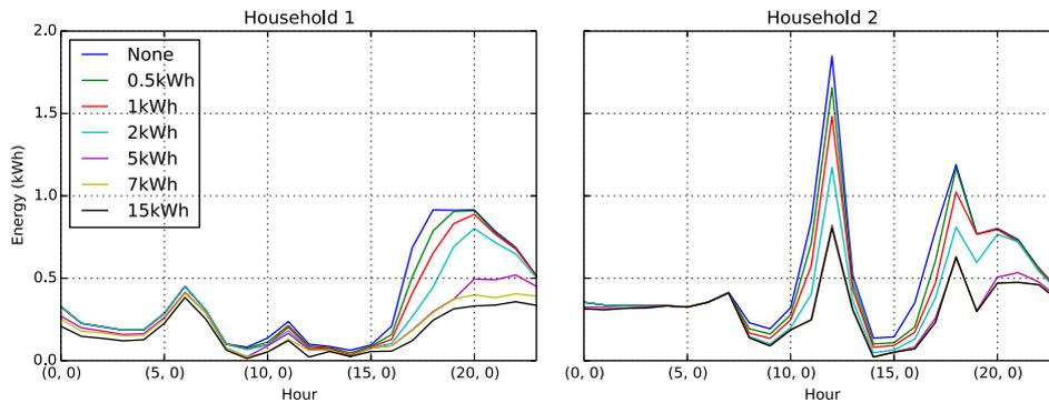
Figure 5.8: Impact of battery capacity on average energy import per 15min
