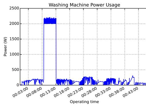
Figure B.3: Washing machine power consumption
