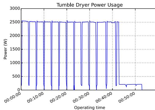
Figure B.1: Tumble dryer power consumption
