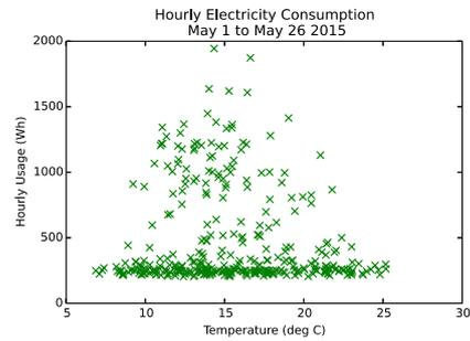
Figure 5.5: Scatter plot of hourly energy consumption for household 1 and temperature
