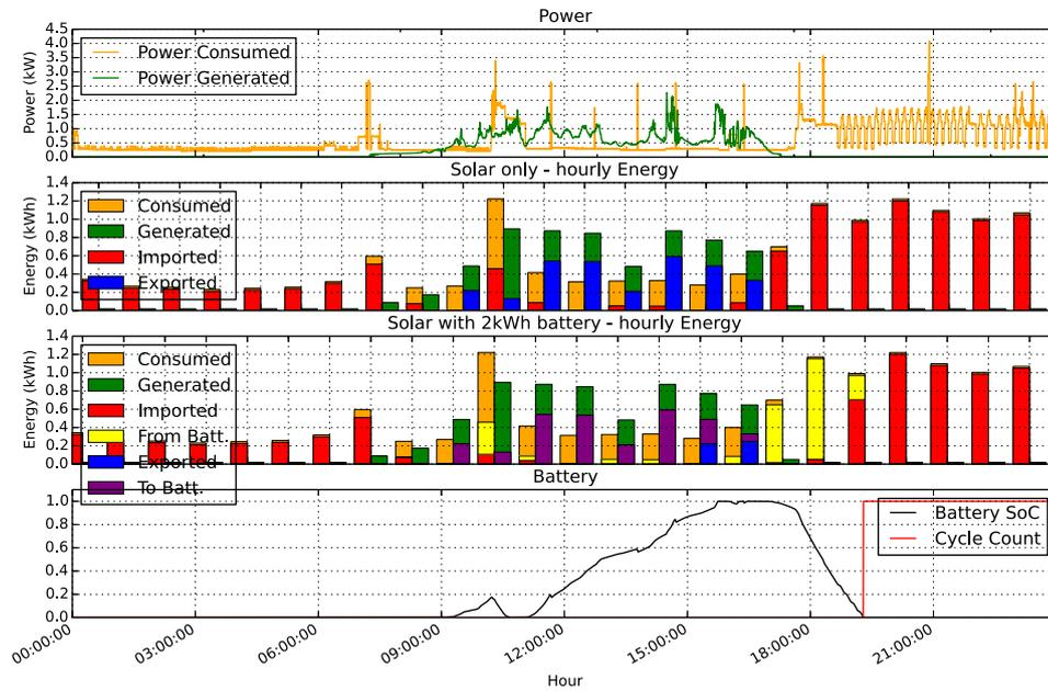
Figure 5.7: Comparison of power and energy over a day, with and without battery storage
