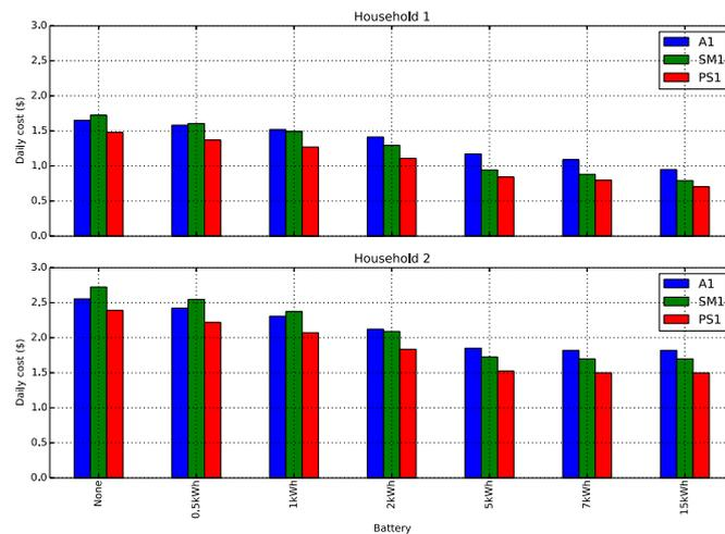
Figure 5.9: Average daily costs with the addition of battery capacity for 2015/05/14 and 2015/06/05 inclusive
