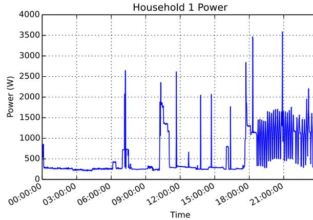
Figure 3.5: Power consumption in a household over the period of a day
