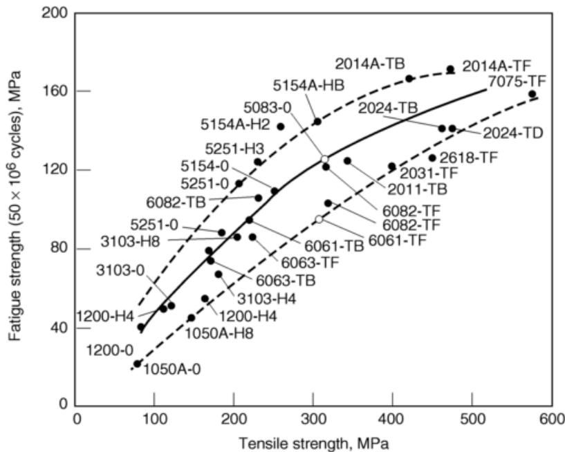
Figure 20: Relationship between the fatigue strength and tensile strength of some wrought aluminium alloys. From 'Selecting Aluminium Alloys to Resist Failure by Fracture - Fatigue Life of Aluminium alloys' (Bucci et.al. 1996)
