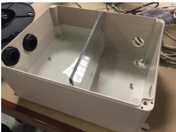
**Figure 18: Waterproof testing of small enclosure partition**
