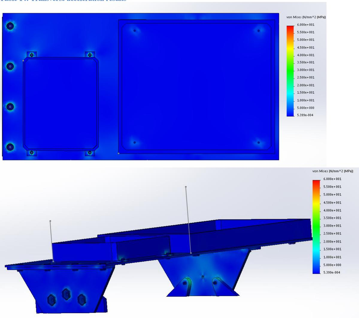
Figure 24: Transverse acceleration results
