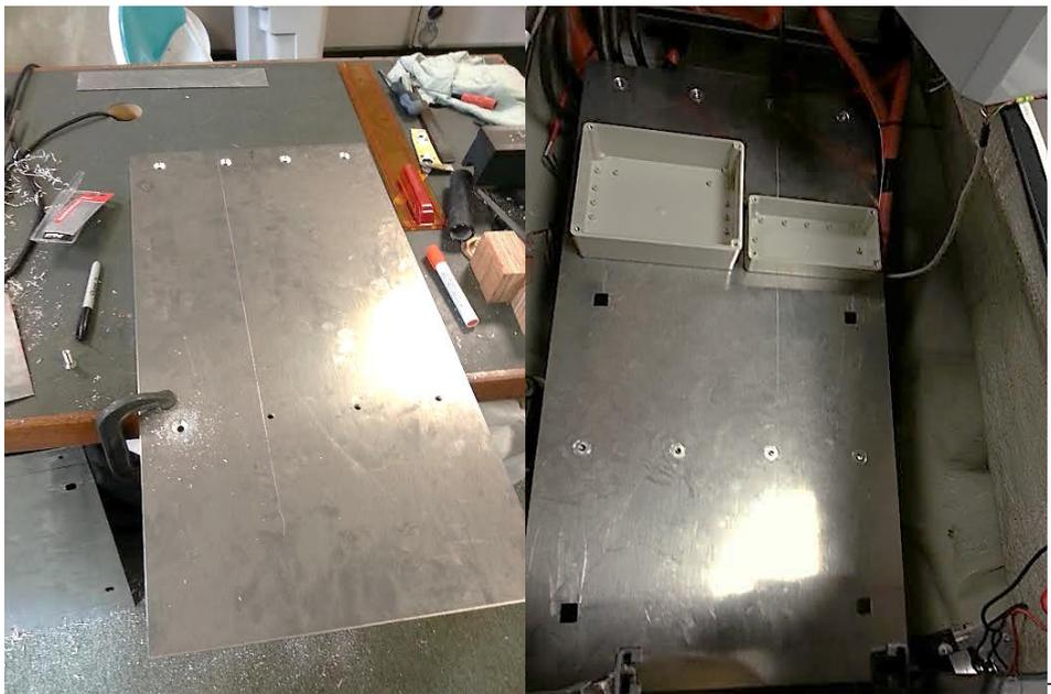
**Figure 14: Mounting plate fabrication showing counter sinking on left and the system installed with keying for the large enclosure visible on the right. Note, the two small enclosures shown is not the final layout**
