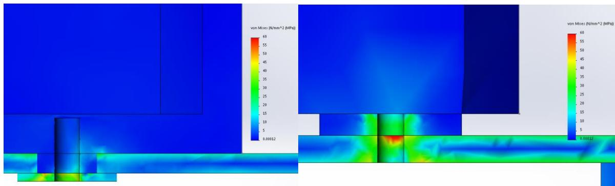
Figure 10: Von Misers stress in mounting points of plastic enclosures, large enclosure on the left and smaller enclosure on the right. Note scale set to maximum of 60MPa and stress in plastic below 40MPa.
