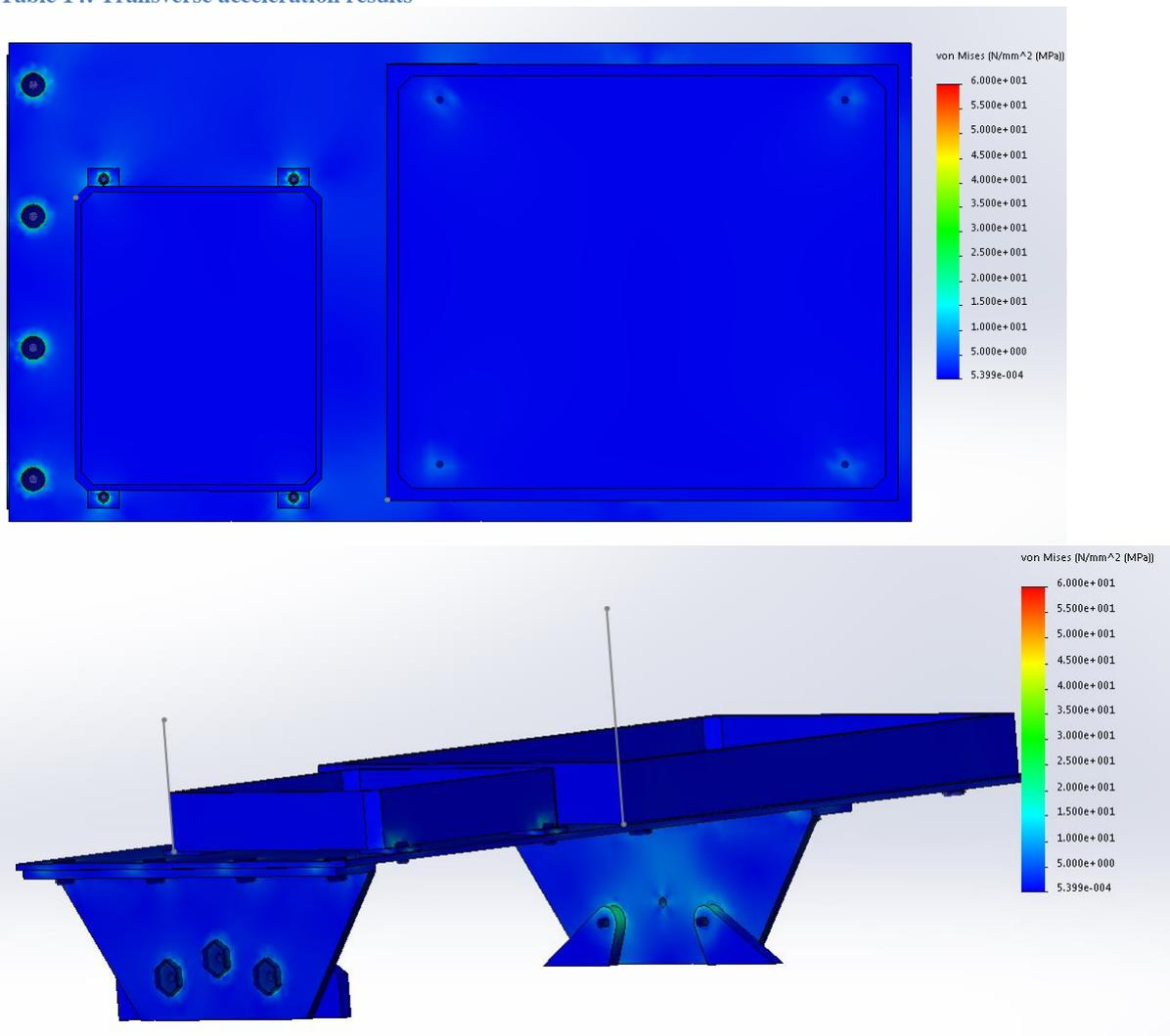
Figure 24: Transverse acceleration results
