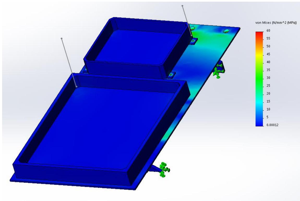
**Figure 11: Von Mises stress in structure with scale set to 60MPa maximum. Note very low stress in plastic components.**
