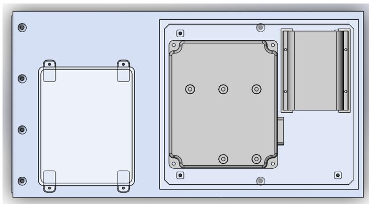
**Figure 15: Mock-up of component layout in the large enclosure and general layout of mounting surface for the final design**
