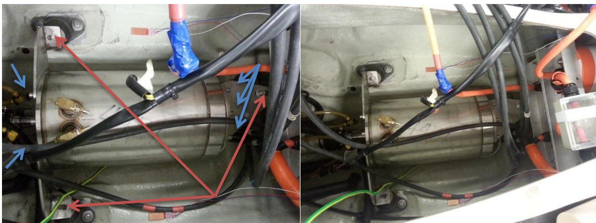
**Figure 2: Available mounting points and interior of hull. Mounts to hull highlighted in red and mounts to motor in blue.**
