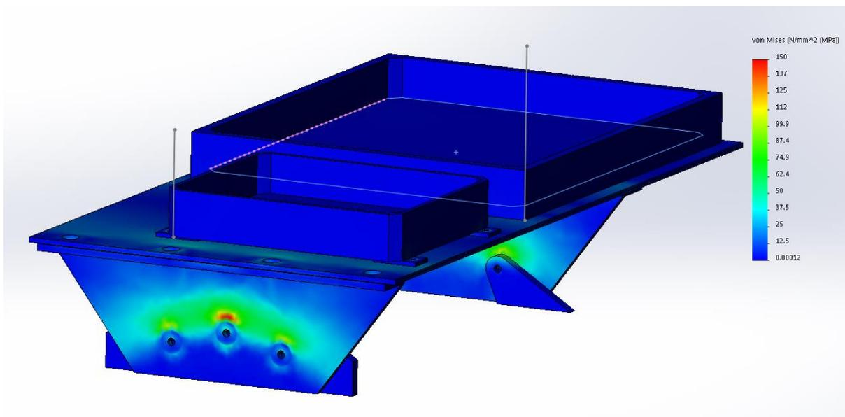
Figure 8: Von Mises stress distribution of the design undergoing highest stress test. Note, maximum stress is 150MPa shown in red.
