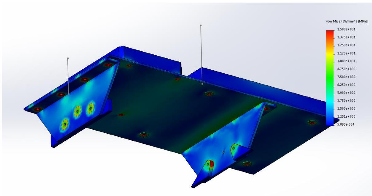
Figure 31: Transverse and Up fatigue stress results
