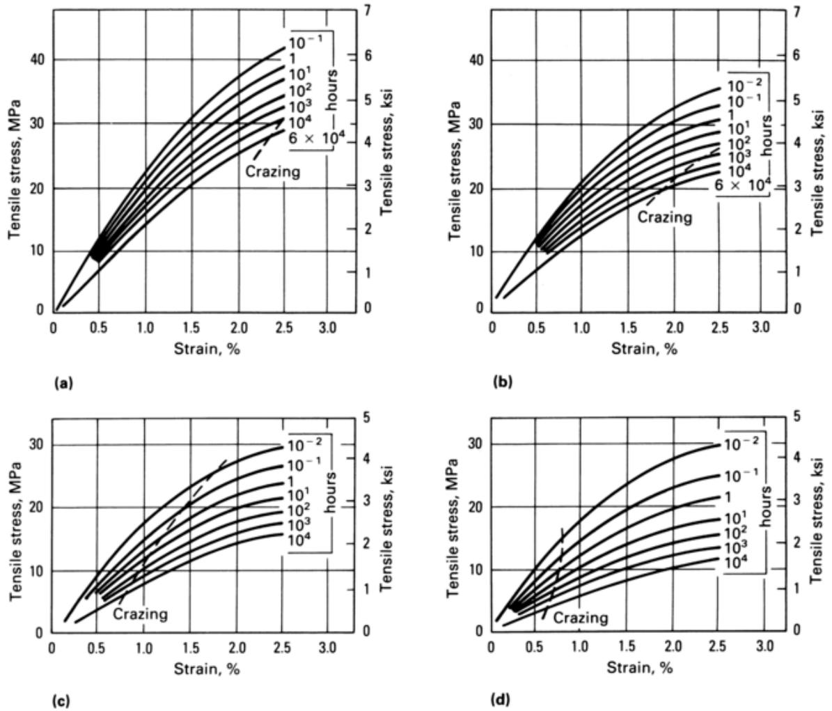
Figure 21: Isochronous plot of polycarbonate stress-strain behaviour as a function of temperature. (a) 23 °C (b) 40 °C (c) 80 °C (d) 100 °C. From 'Fracture of Plastics – Failure Analysis and Prevention' (ASM International 2002)
