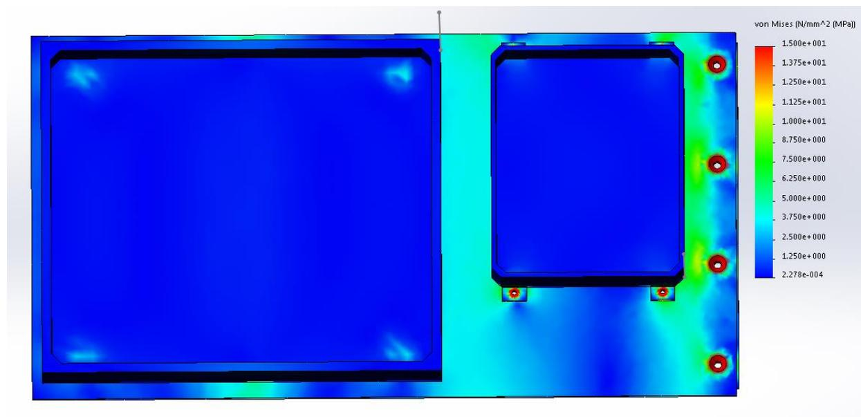
Figure 12: Highest stress typical load condition. Note, maximum of scale set to 15MPa.
