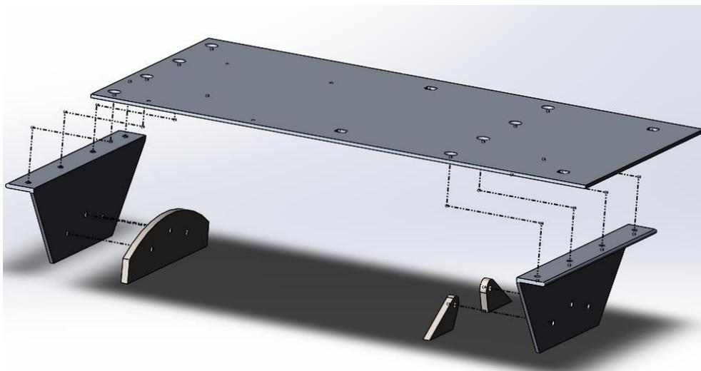
Figure 7: Final Design exploded view of mounting structure. Note, the small components to the bottom of the design are the representation of the mounting points on the motor.
