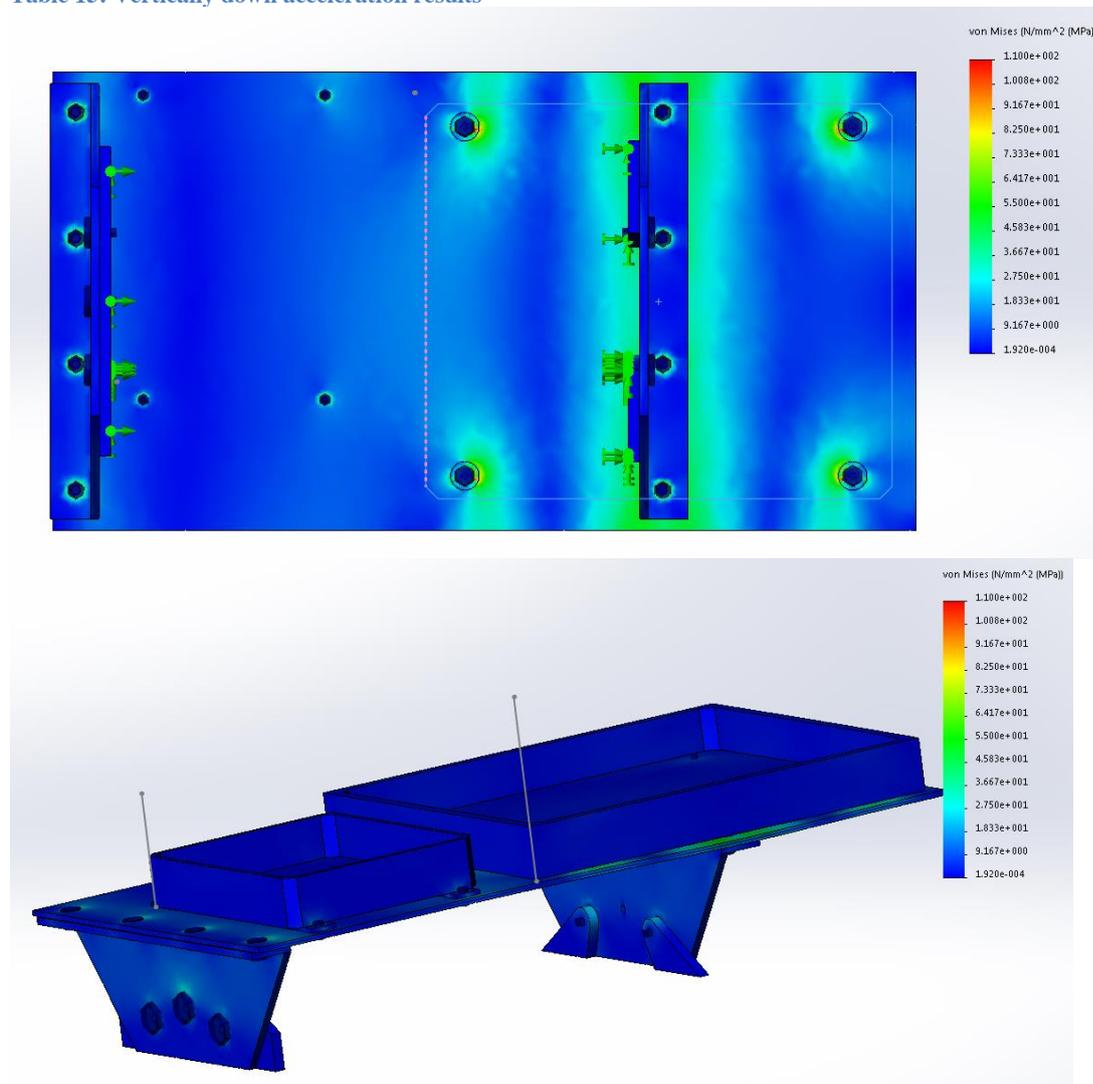
Figure 25: Vertically down acceleration results
