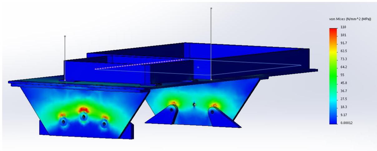
**Figure 9: Von Misers stress distribution of design undergoing highest stress test. Red highlighting any area over the yield strength of the material. Note large areas of vertical members below 70MPa suggesting localised but not total yield.**
