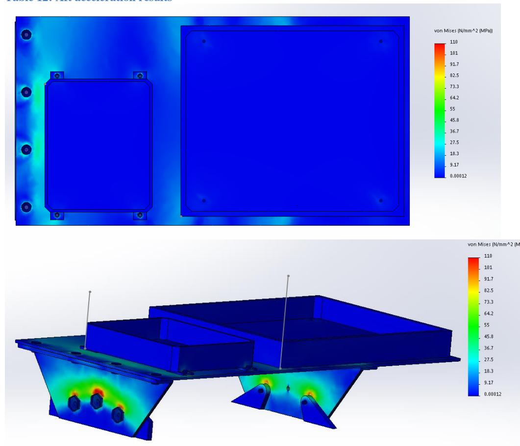
Figure 22: Aft acceleration results
