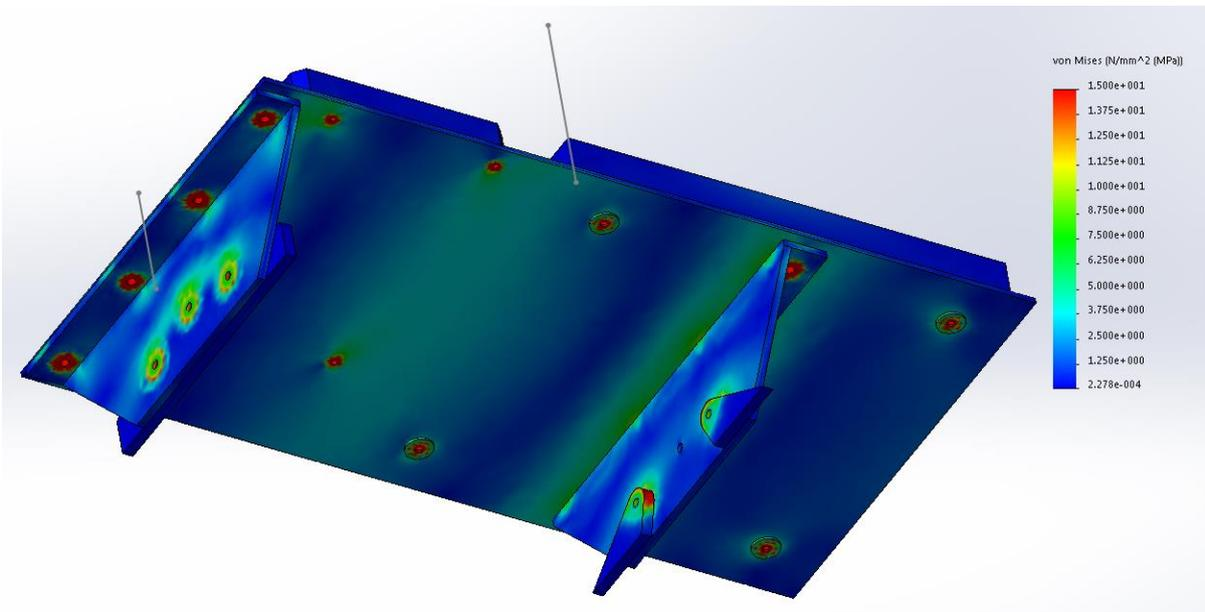
Figure 30: Aft and Up fatigue stress results
