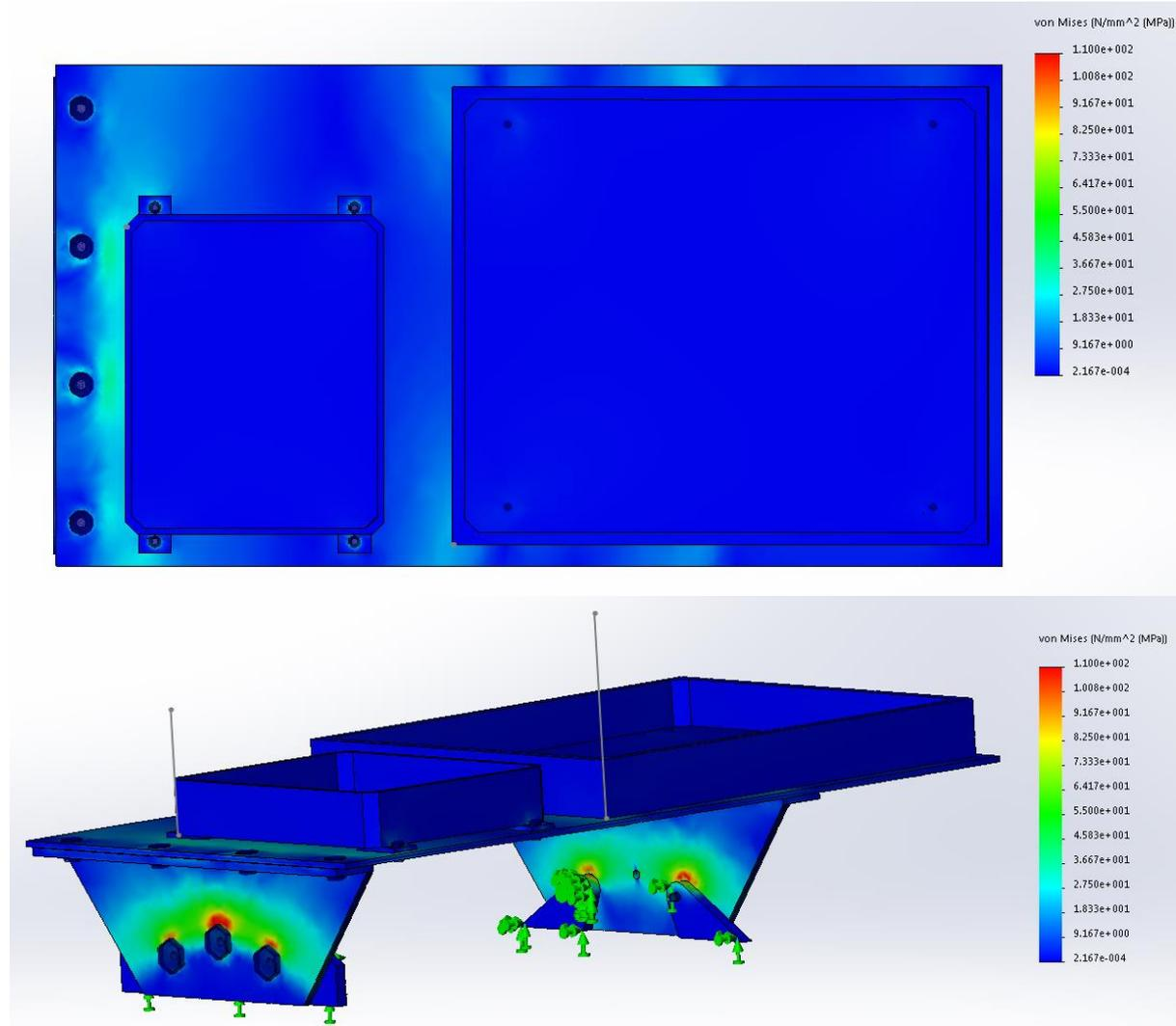
Figure 27 Aft and transverse combination acceleration results
