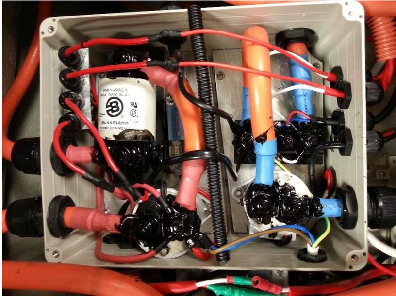
**Figure 17: Additional components in their final installation. Note, waterproof partition between the two potentials, with 96v on the left and ground to the right.**
