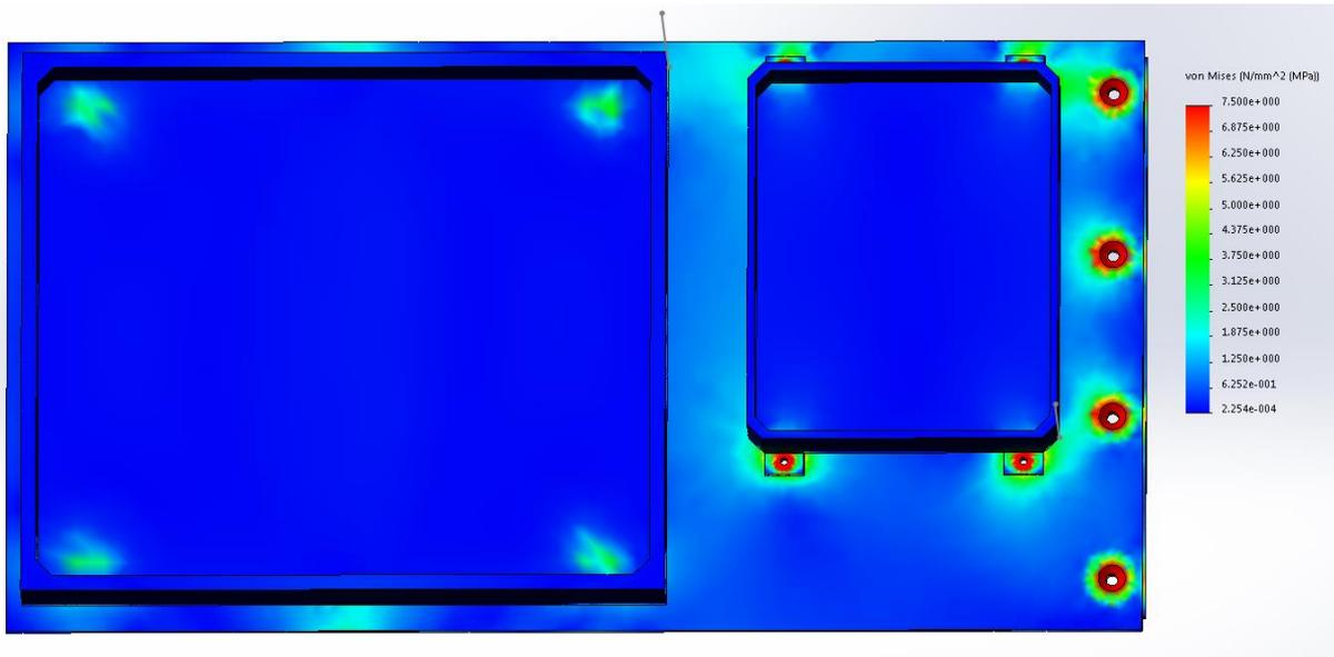
Figure 13: Minimum load condition of gravity force. Note, maximum of scale set to 7.5MPa.
