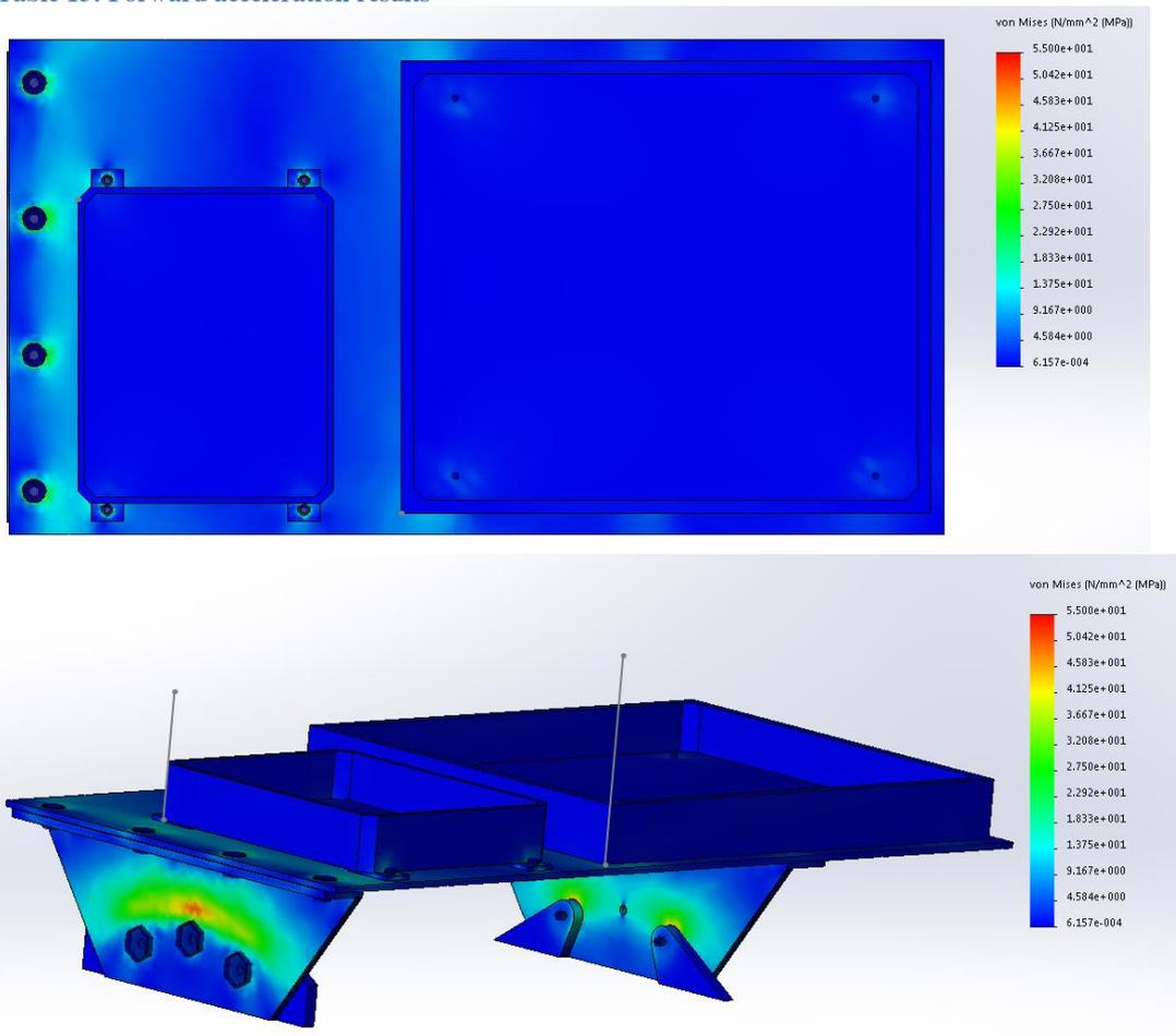
Figure 23: Forward acceleration results
