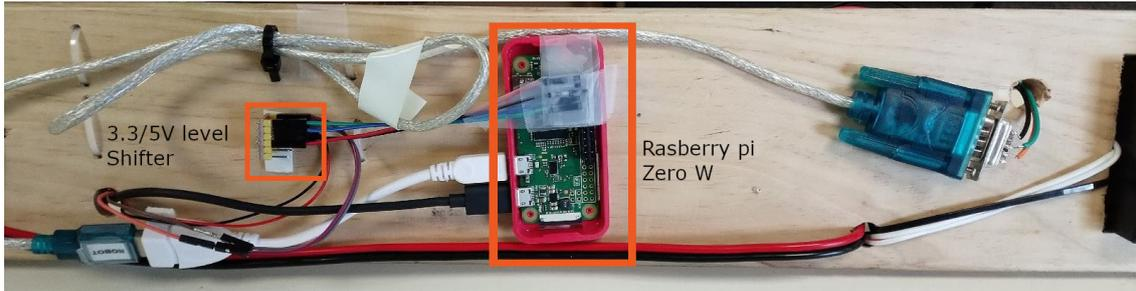
Figure 3: New hardware components
