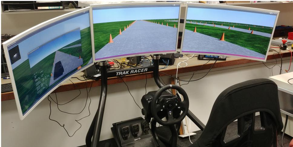
Figure 4: Autonomous driving simulator setup.
