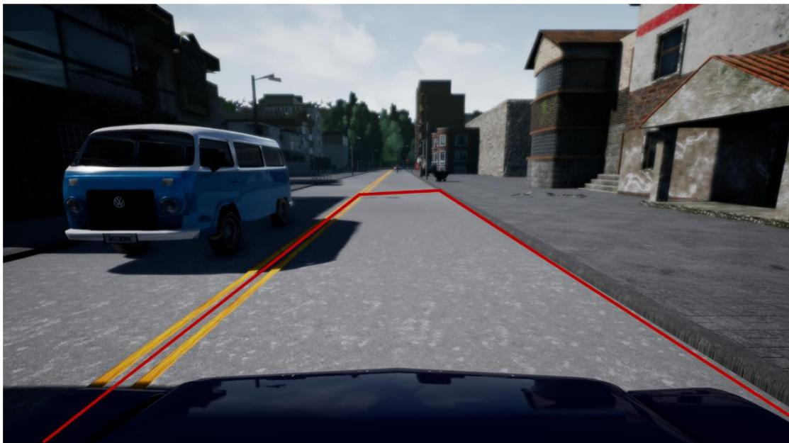
Figure 23: ROI area for vehicle and pedestrian detection
