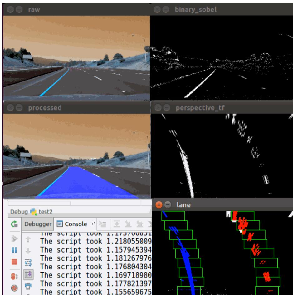
Figure 10 Process breakdown of lane detection
