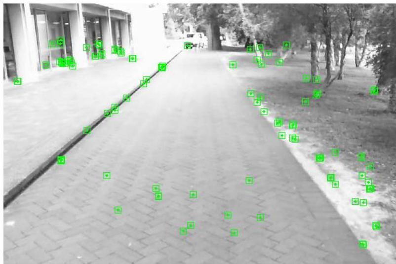
*Figure 15 Feature Extraction in ORB SLAM2. (green marker is the ORB feature matched with current key frame)*
