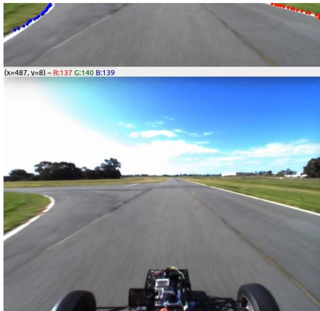
*Figure 23 Lane detection on RAC race track.
