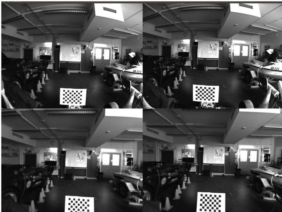
*Figure 5 Top: Raw Images for both Cameras; Bottom: Calibrated Images from both Cameras*
