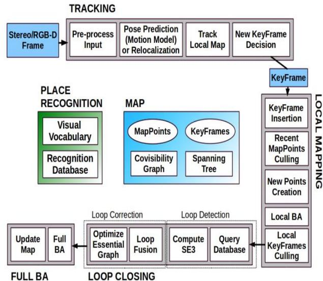
Figure 9 System Overview of ORB SLAM2 [2]
