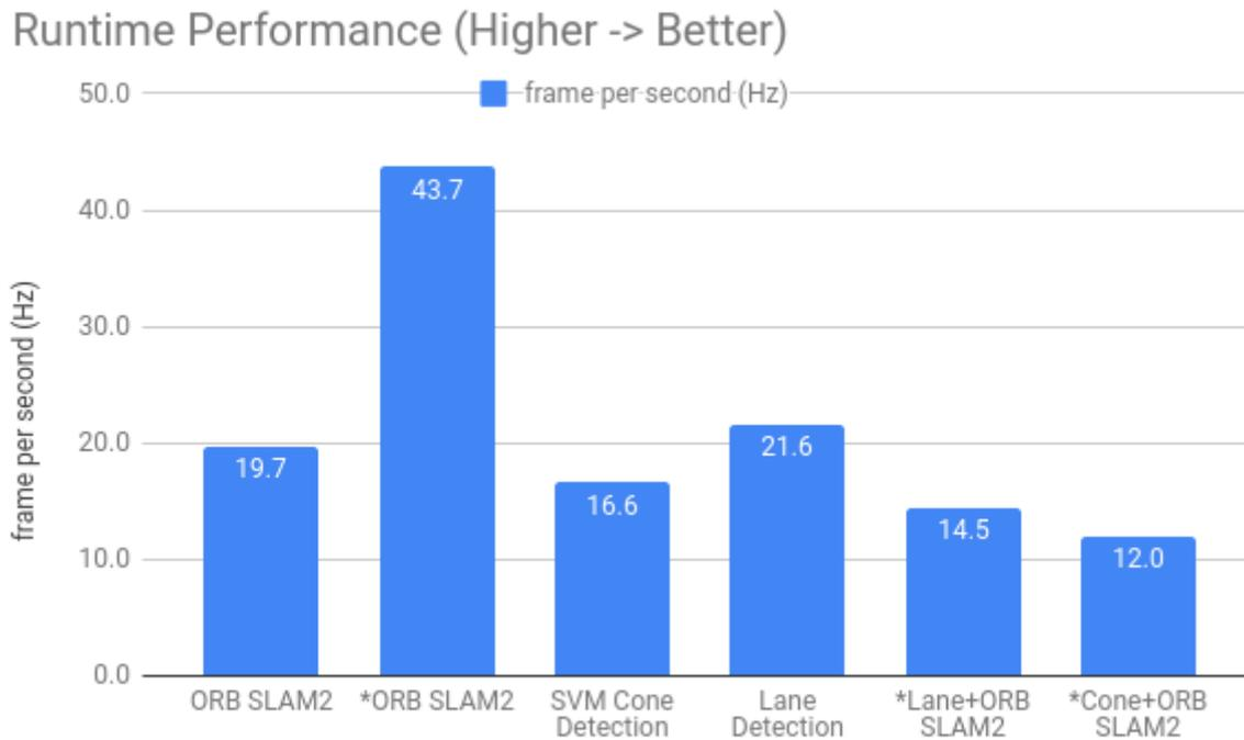
Figure 24 Runtime Performance on SAE vehicle.
