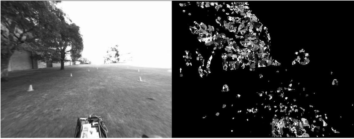
*Figure 6* Depth Map generated with stereoscopic cameras
