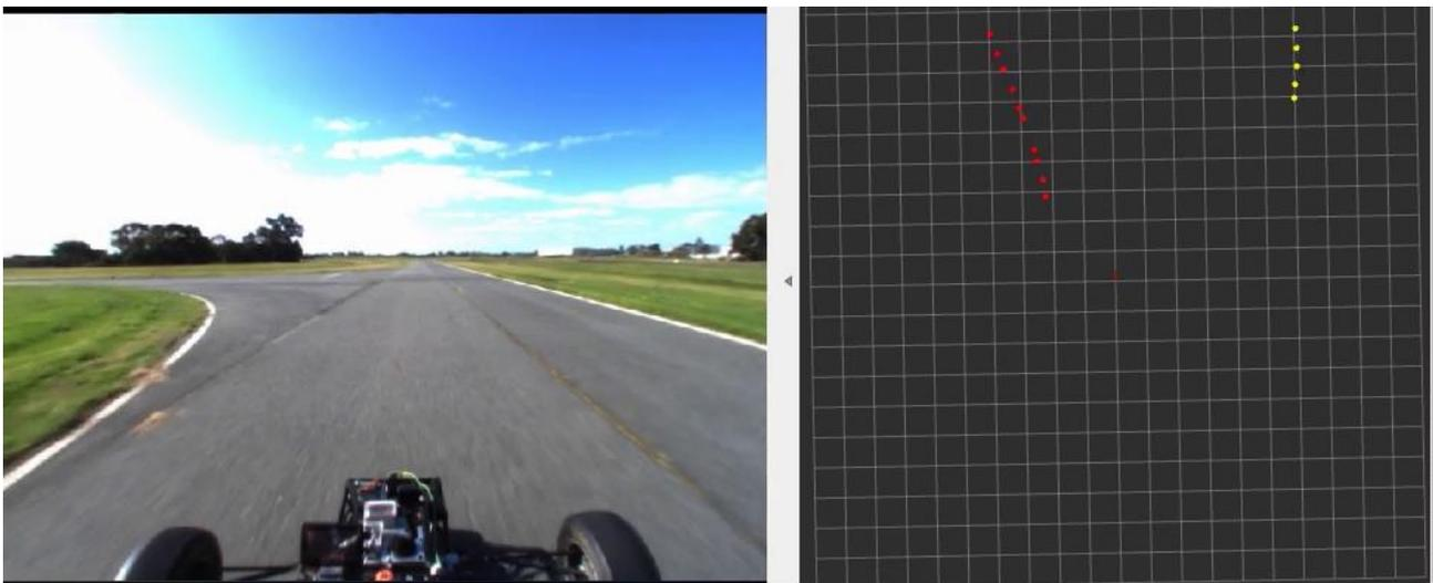
*Figure 22 left: raw image; right: lane points passed to path planner*
