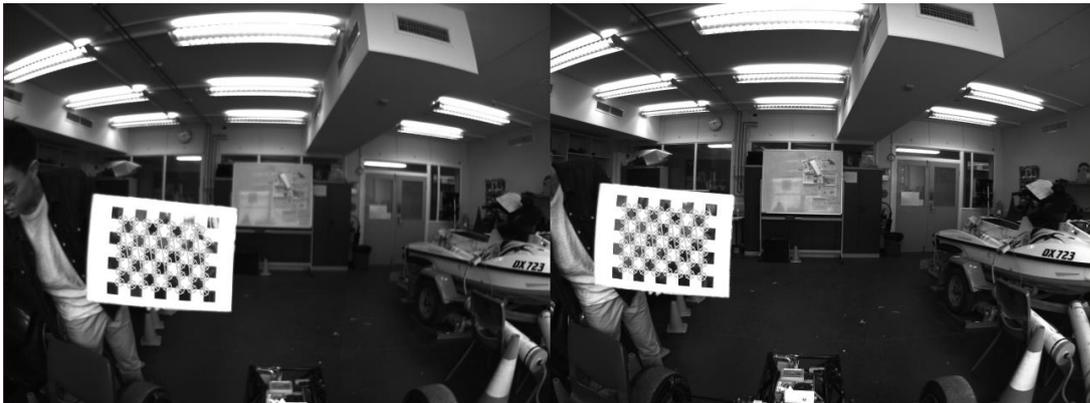
*Figure 4 Camera Calibration Examples for both Cameras*
