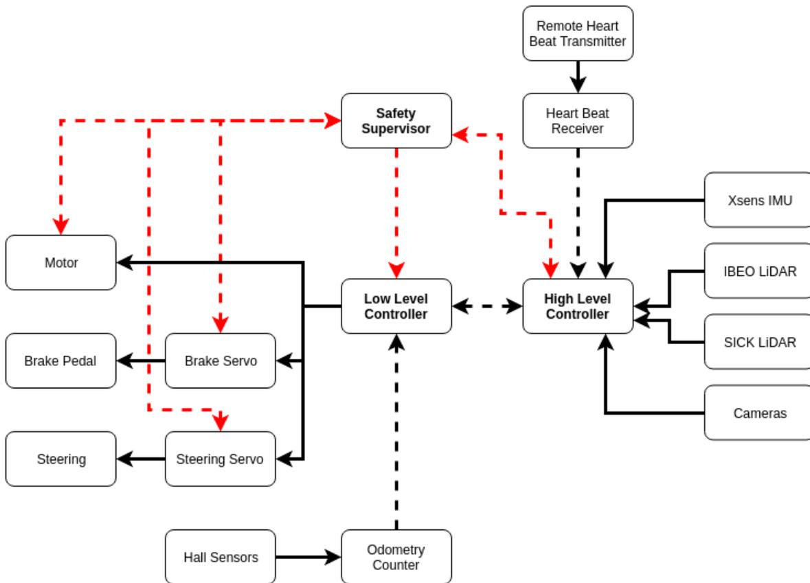
Figure 3 System Architecture
