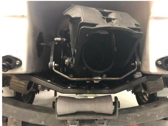
Figure.8 Outlet of the propeller duct full right
