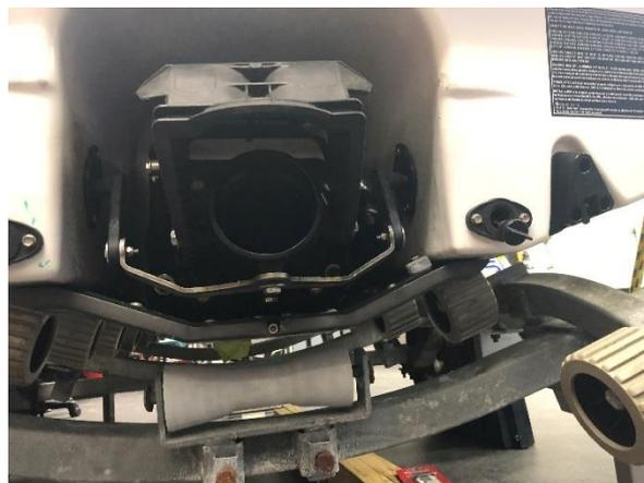
Figure.8 Outlet of the propeller duct without steering angle
