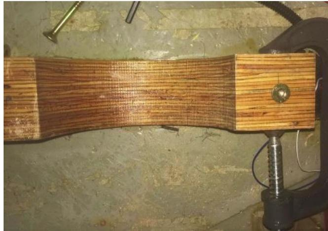
*Figure 8: The screw on the right enters between the laminated sheets of wood.*
