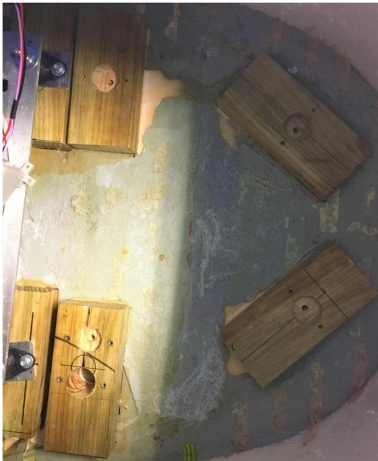
*Figure 47: The blocks were now adhered to the hull.*
