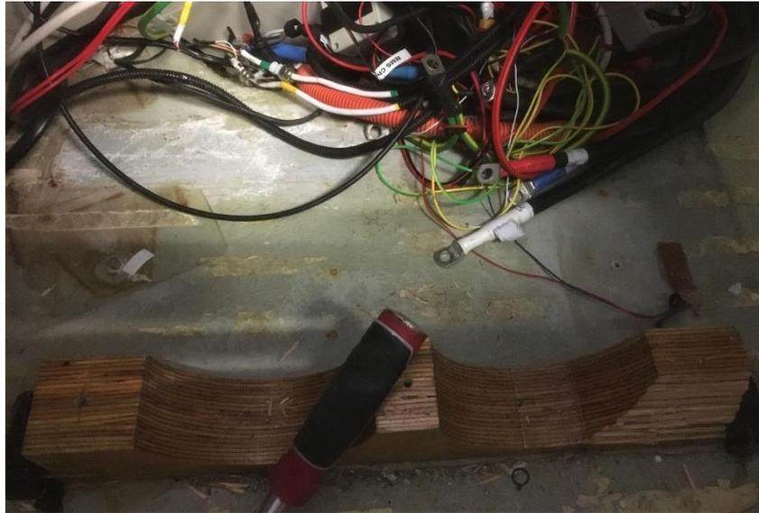
*Figure 42: One laminated wooden cradle removed.*
