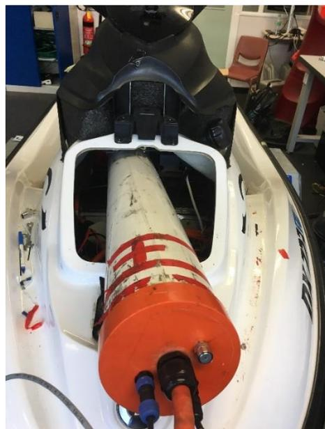
*Figure 58: Starting to load a battery tube through the front.*
