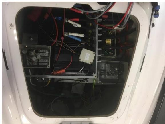
*Figure 5: Relocated position of the MC box and other components at the bow.*
