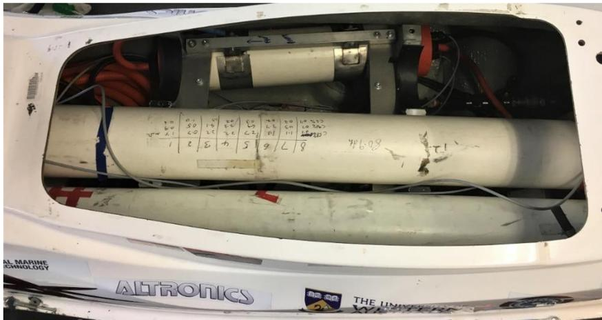
*Figure 4: Partially disassembled battery mount reveals small battery tube (top), and two large tubes.*
