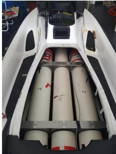
Figure 12: The latest battery mounting system (Chau 2017).
