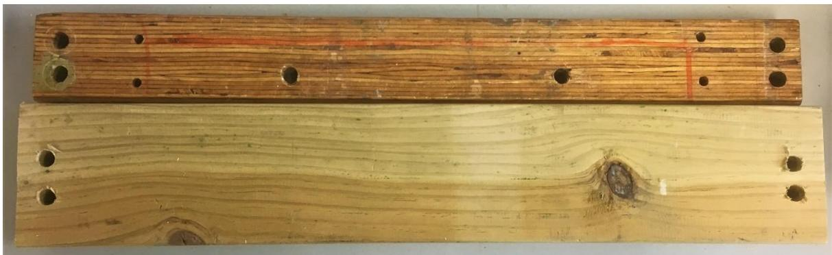
*Figure 43: A comparison between the original laminated crossbeam (top), versus the structural pine crossbeam (bottom).*
