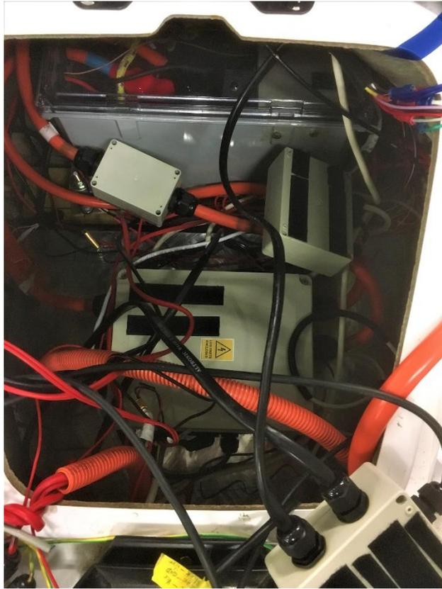
*Figure 54: Smaller components being mounted onto the plate with Velcro strips.*
