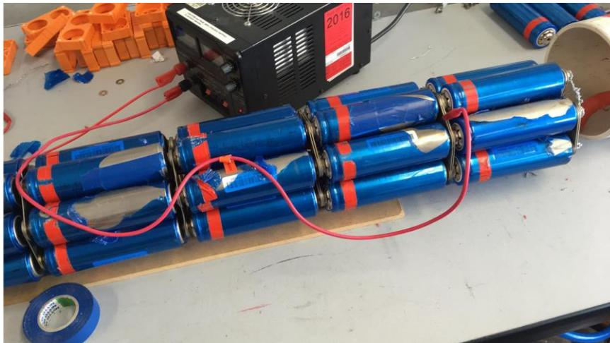
*Figure 55: The cells within a large tube, with each section consisting of eight parallel cells.*
