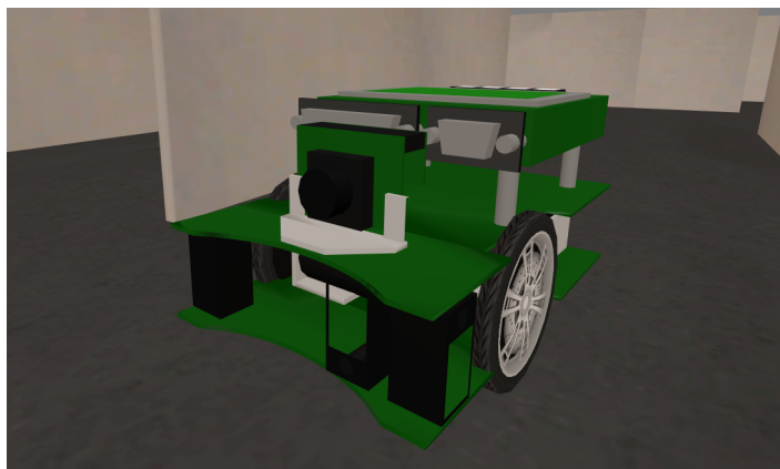
Figure 2.2: Simulation of a differentially driven robot with EyeSim.
