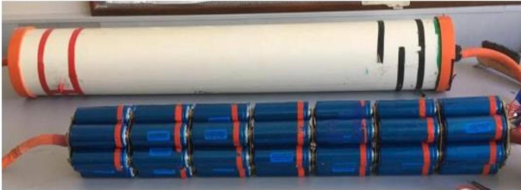
Figure 24 - 38120L Batteries, and Battery Pack Tube [2]
