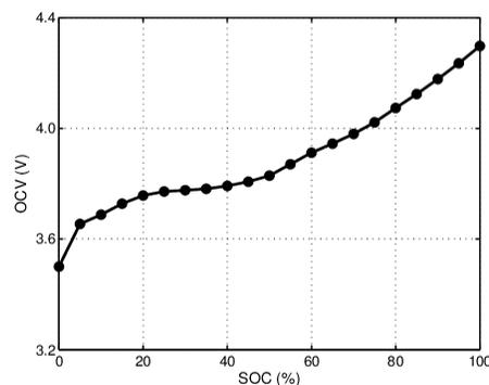
Figure 3 - OCV/SoC of a Li-ion Battery [6]
