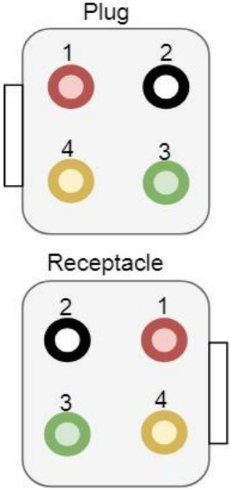
**Figure 27 - Cable Standard: Back of Deutsch Connector**
