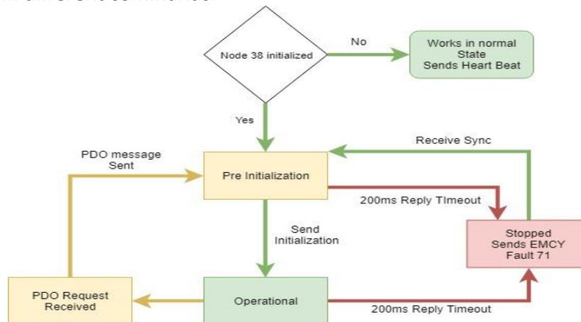
Figure 12 - CANopen implementation for Curtis Motor Controller
