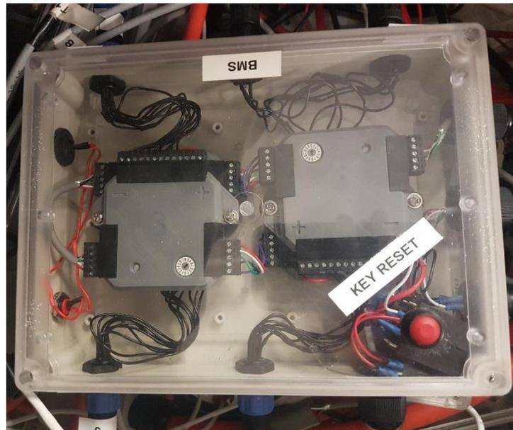
Figure 23 - BMS12 installation inside the REVski
