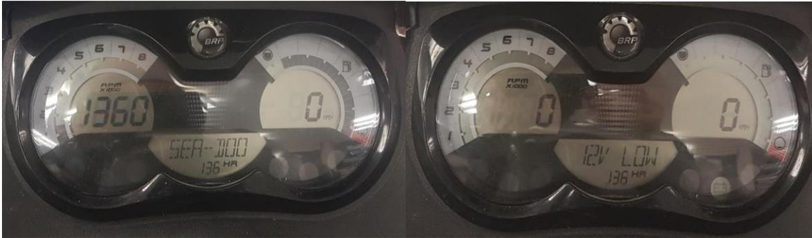
Figure 19 - RPM Meter displaying 136 Amp Draw, and low SoC warnings presented on display
