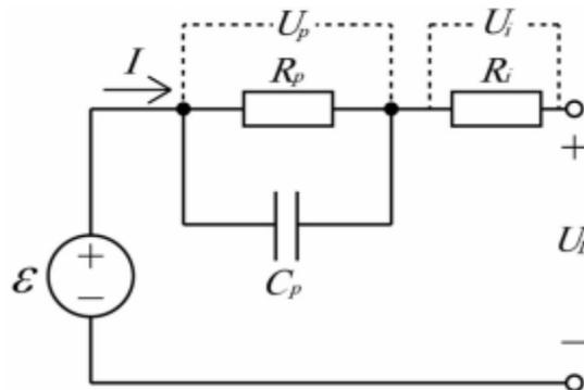
**Figure 2 - Lumped Model of Cell [5]**
