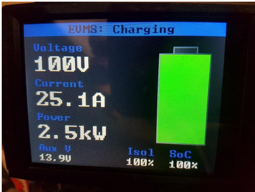
Figure 30 - EVMS monitor during 25A charging
