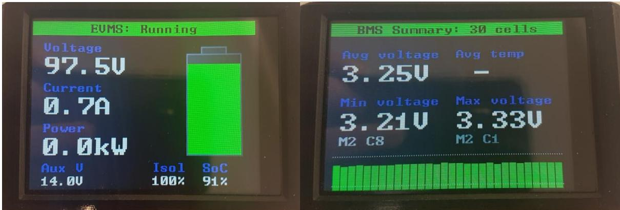
Figure 29 - ZEVA Monitor displaying REVski pack voltages and outputs
