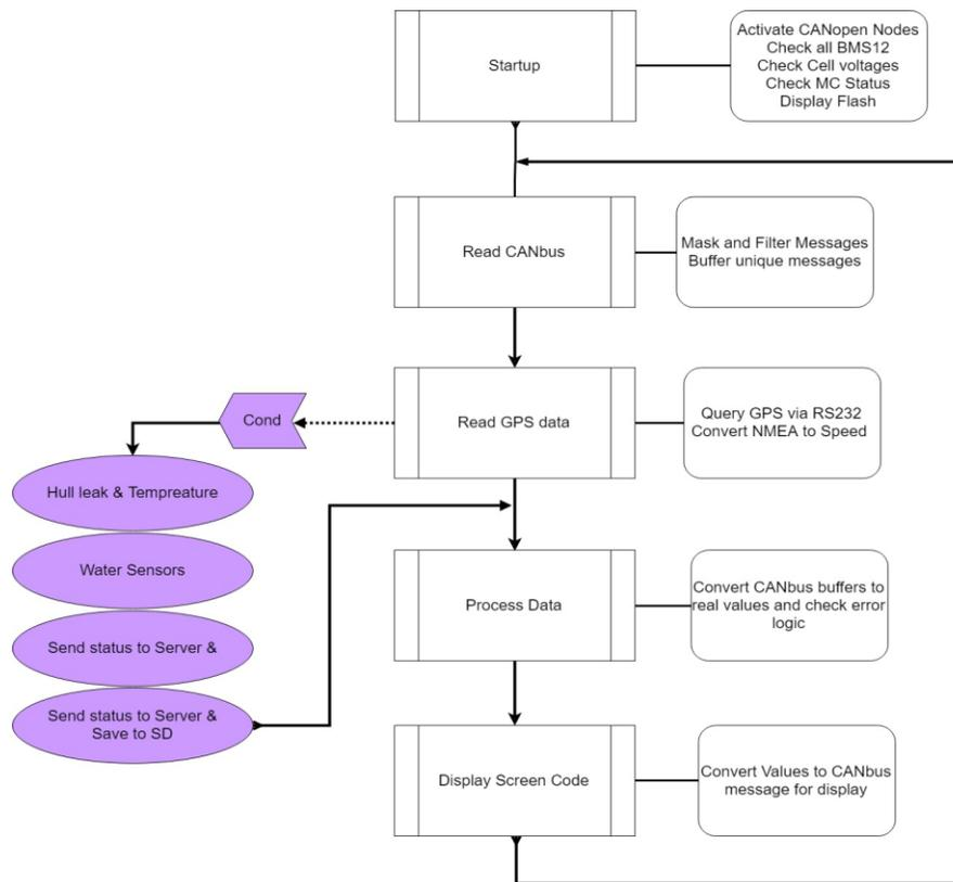
Figure 18 - ECU state machine diagram
