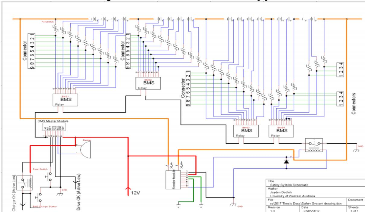
Figure 7 - Previous Safety System Architecture [2]
