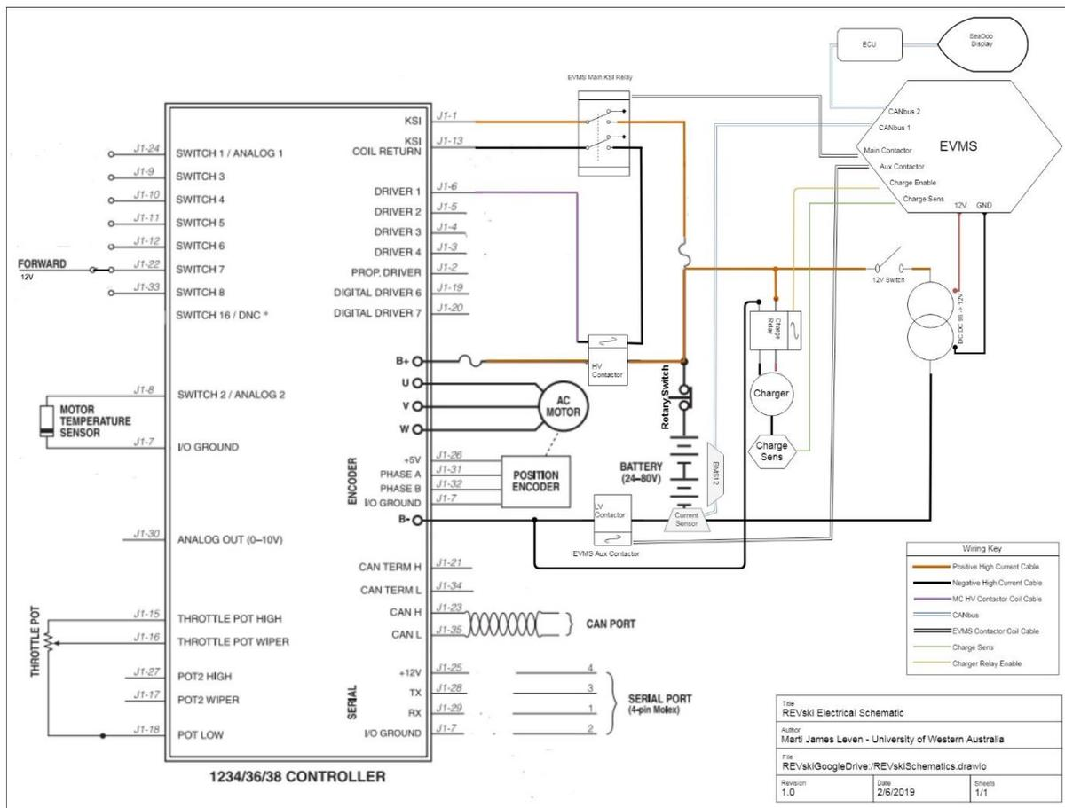
Figure 14 - Updated Electrical Schematic
