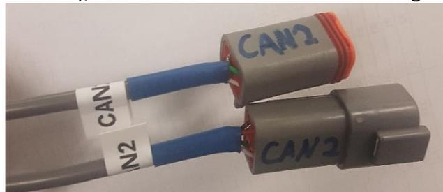
**Figure 28 - Standard for CAN2 using Deutsch Inline connectors**
