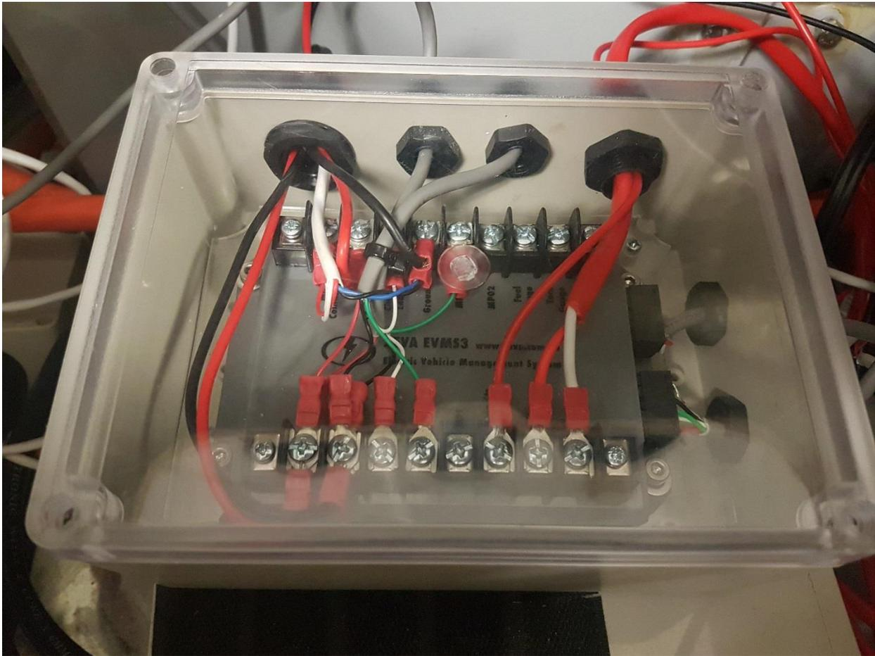
**Figure 21 - Mounted EVMS within system**
