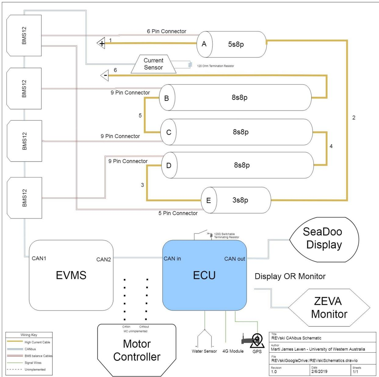
Figure 15 - CANbus schematic
