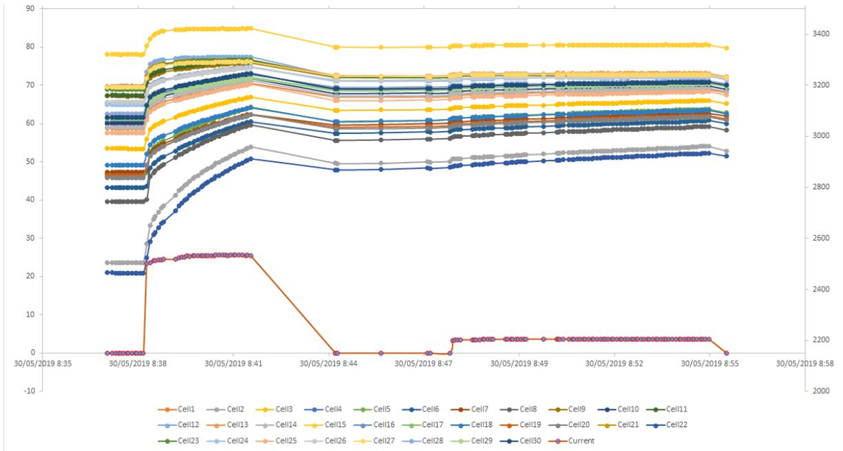
**Figure 31 - Cell Voltages (mV) during continuous current charging, at 25A and 3.5A modes**
