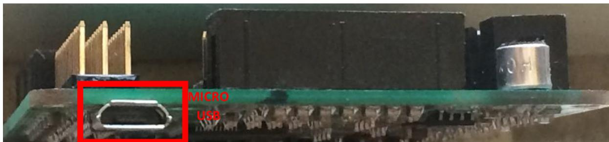
Figure 4.11: Micro USB to communicate with a host controller (e.g. Raspübery Pi)
