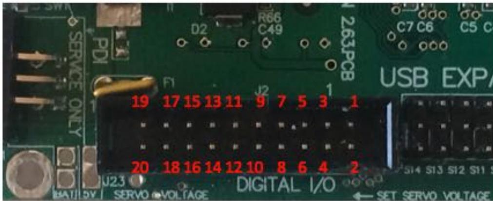
Figure 4.10: Digital I/O Port. These ports are designed so that a user can write and read data as a Byte.
