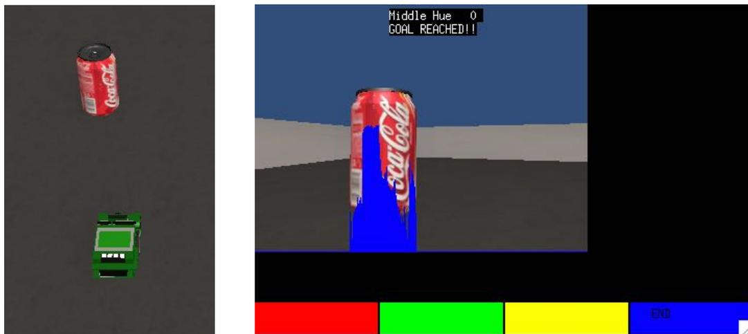
Figure 5.2: Robot closing in on Coke can; robot display with superimposed color histogram
