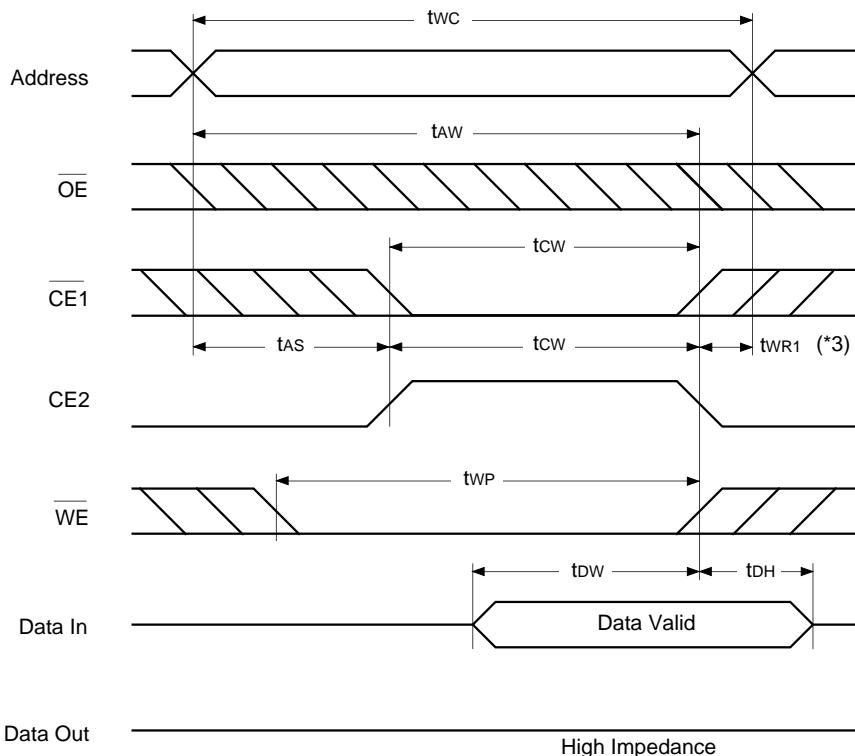
\*1 Write is executed when both  $\overline{CE1}$  and  $\overline{WE}$  are at low and  $CE2$  is at high simultaneously.
