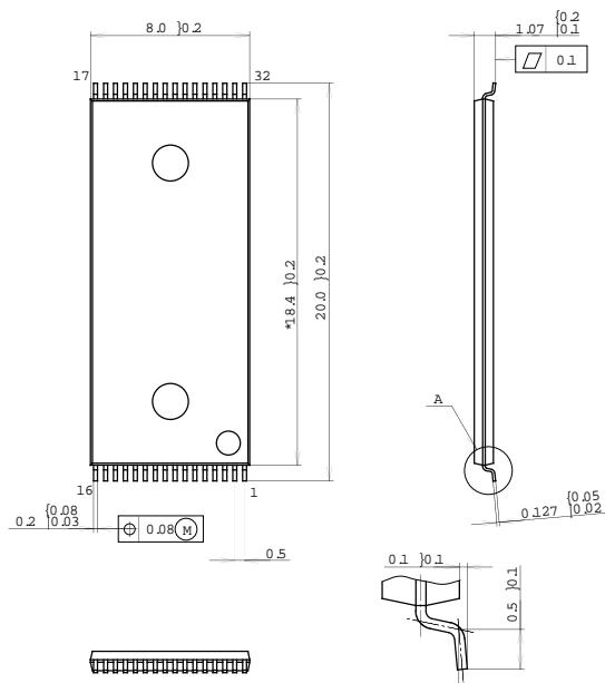
NOTE Dimension g does not include mold protrusion.
