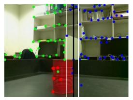
In the picture above, green dots and blue ones are the corners in the left and right side of the frame and the red dots are potential obstacles. Around this frame the eyebot moves rather slowly as no distinct optical flow vector lines can be seen.
