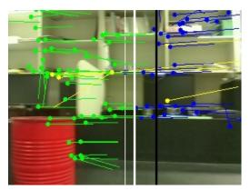
The green and blue dots are (current) corners and the lines are their optical flow vectors. The yellow lines are optical flows that are too large. In this frame nearly all the optical flows are large, which indicates that the eyebot has moved very fast.
