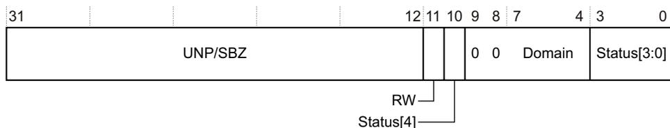
**Figure 3-33 Data Fault Status Register format**
