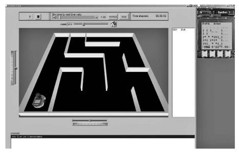
The simulation system "EyeSim" has been completely revised, resulting in the release of versions 6.0 and 6.1. EyeSim now also runs under Windows and has a greatly improved user interface and graphics display. Research on error models has allowed us to build improved sensor and actuator models. These result in more realistic robot behavior and can be used to test the robustness of robot application programs in more realistic simulations.
